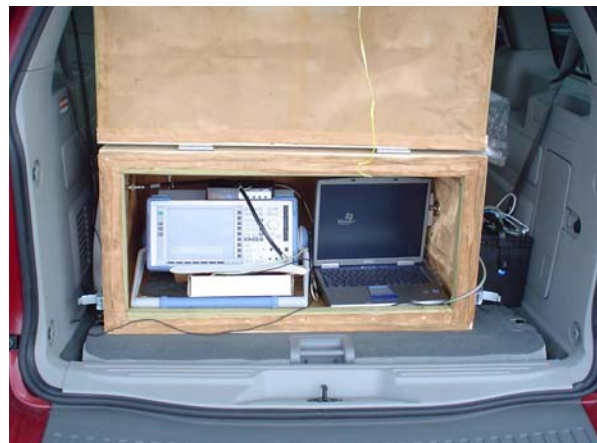
Figure 1: The RF shielded enclosure in which all the data collection equipment is placed.
