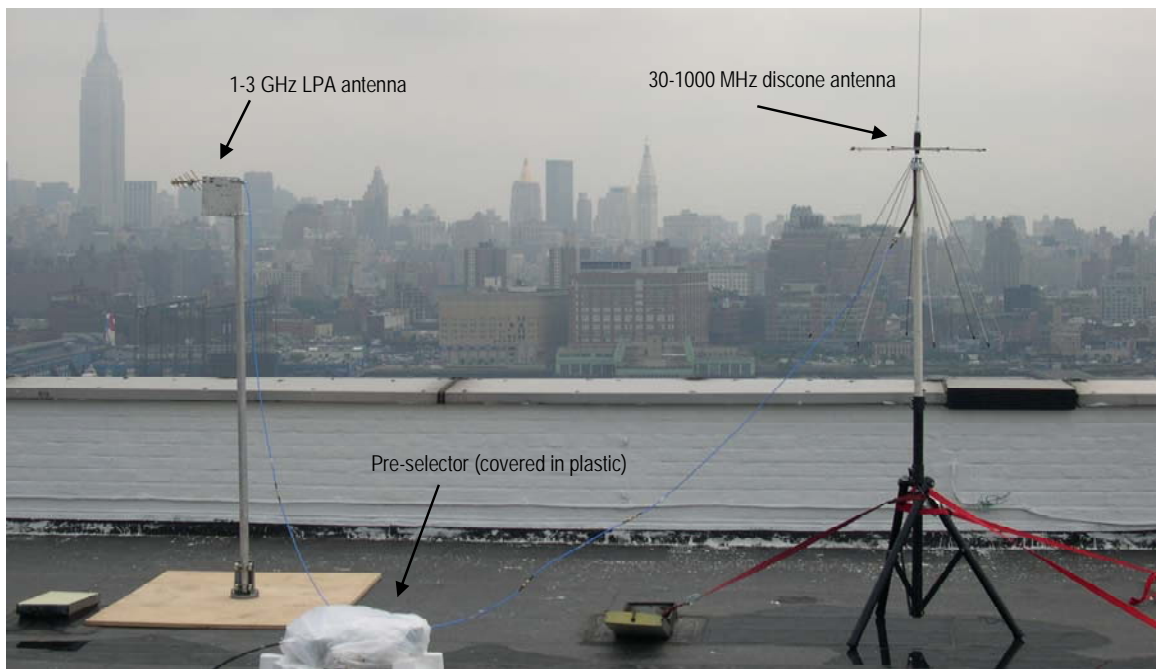
Figure 2: Antenna and Pre-Selector on roof in New York City.
