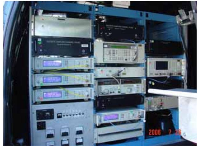
Figure 7. Interior view of the receiver mounted in the van.
