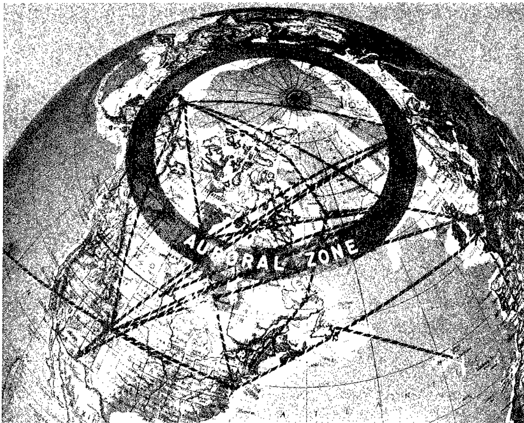
Radio propagation paths used in auroral region experiment to measure high frequency transmission loss.
