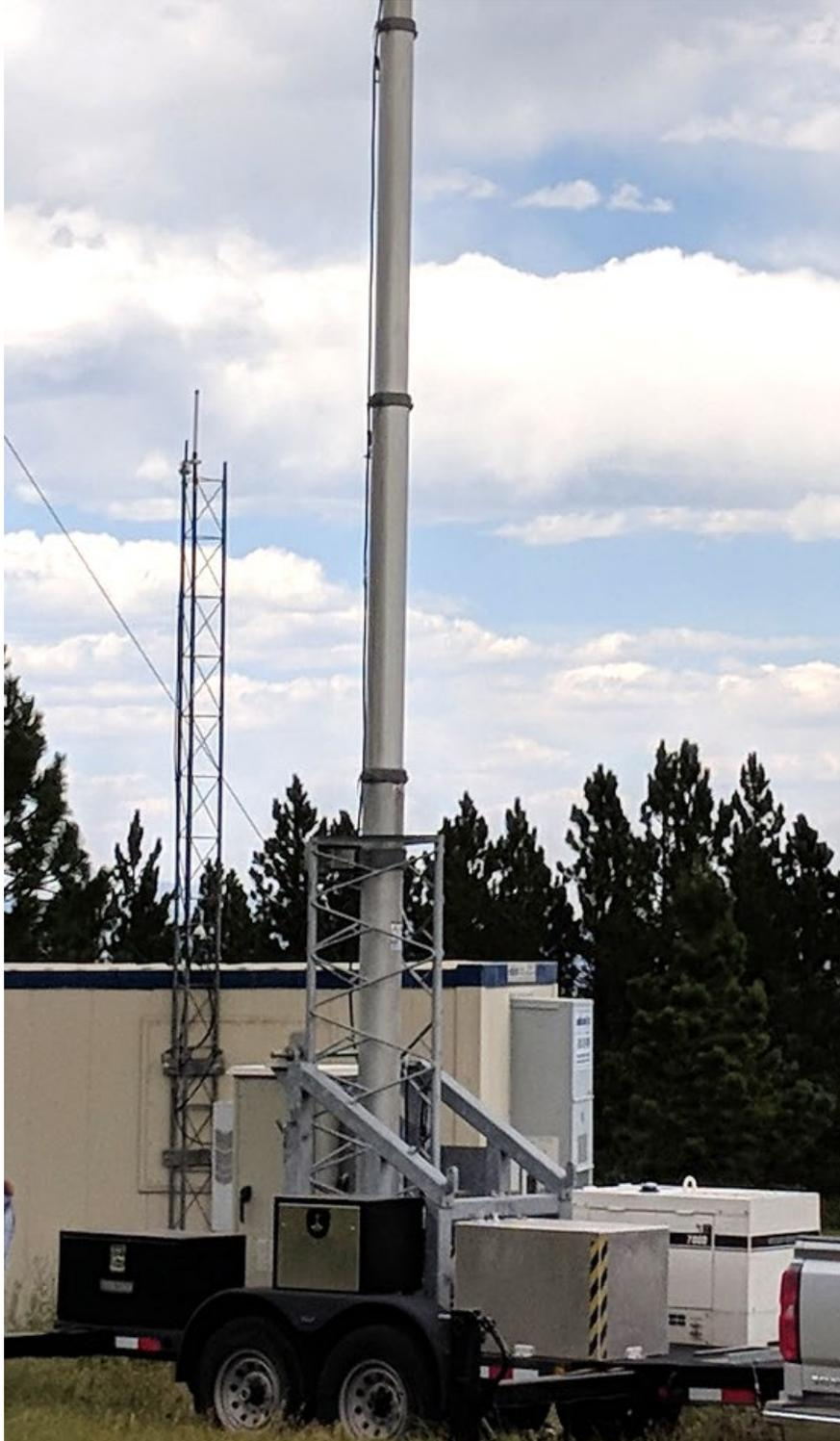
Figure 2. Picture of the COW set up at the transmit location on Kohler Mesa. The mast is extended 60 feet with the antenna mounted on the top of it. The equipment cabinet is seen near the rear of the trailer behind the mast.
