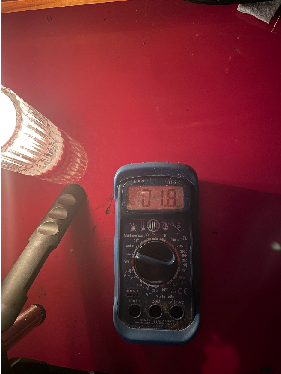
Figure 14. Scenario 3 (Candle) 01.8 lux (01.8 on \times 1 lux scale).
