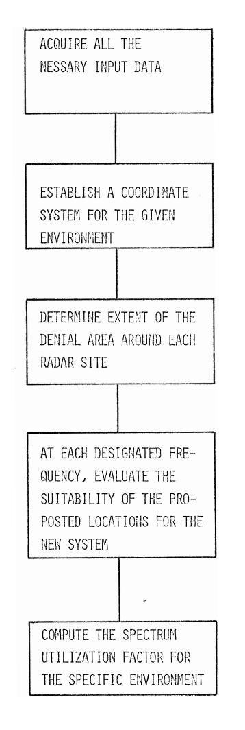
Figure 2-2. Simplified Flow Diagram for the Processor Program
