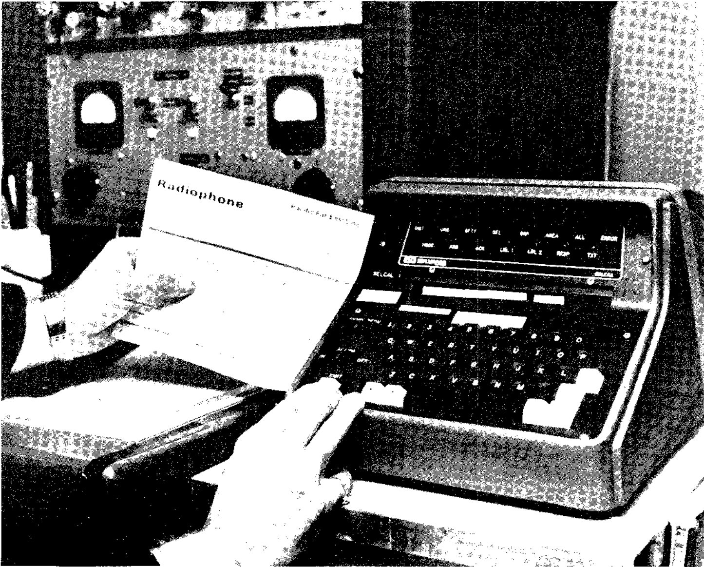
Figure 2-12. A terminal for an experimental digital selective calling system (SELCAL) for maritime use.
