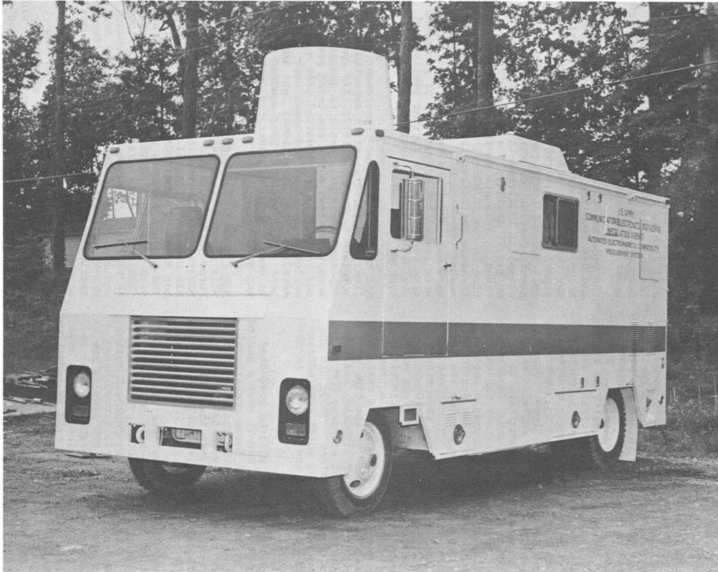
Figure 1-19. Data acquisition vehicle of TAEMS system. This unit is designed to be air transportable and can be air lifted by helicopter.
