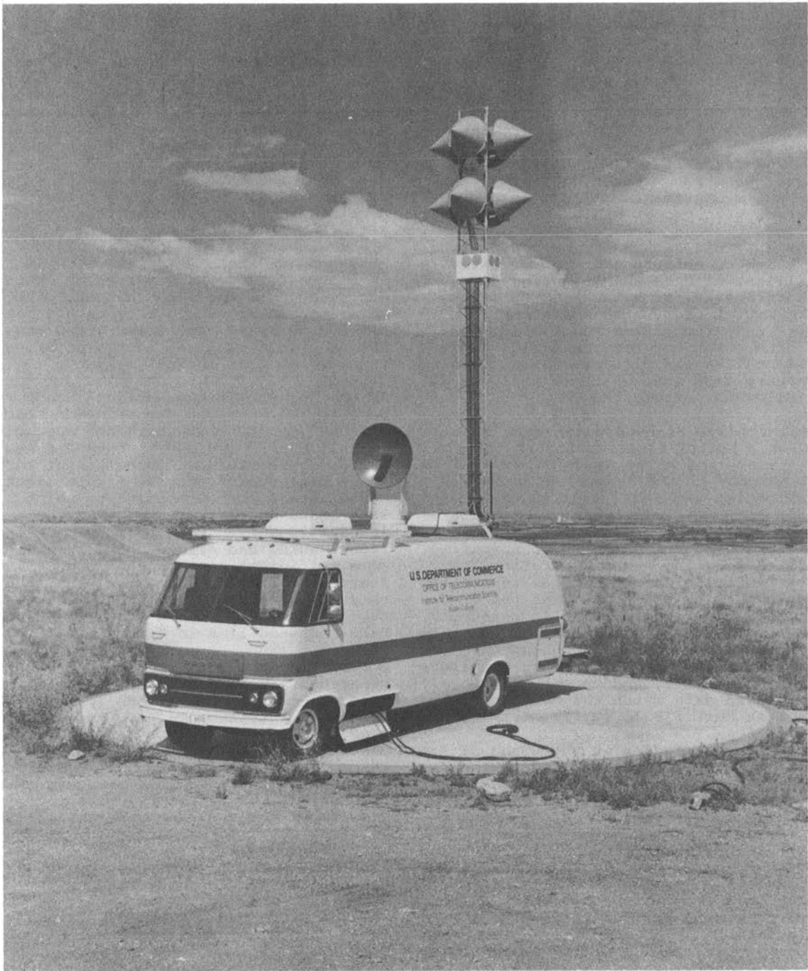
Figure 1-24. The Radio Spectrum Monitoring System undergoing antenna calibration testing at an OT/ITS antenna range.
