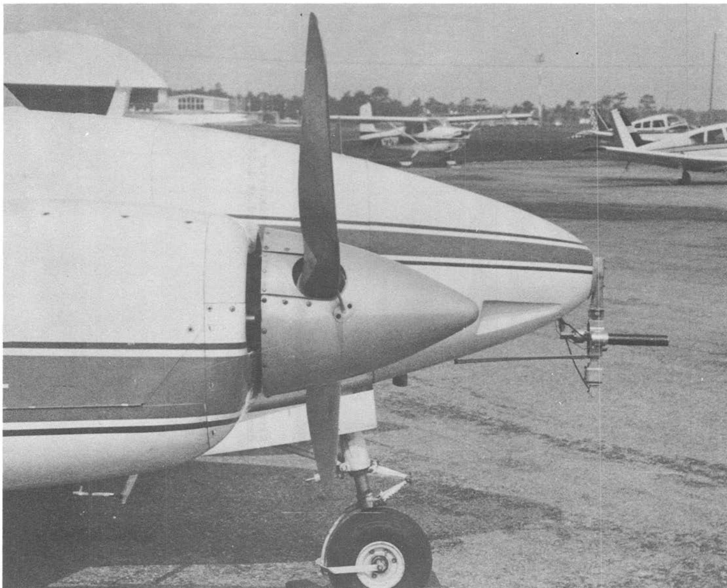
Figure 3-16. Sensing cavity of microwave refractometer with temperature and pressure sensors mounted on nose of aircraft. Profiles of structure function parameter C_n are calculated up to 30,000 feet altitude from resulting data.
