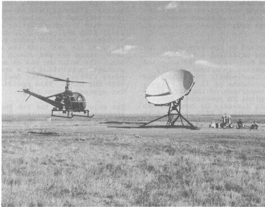
Figure 1-31. Light Terminal (LT) Antenna Group (G/T-26) at the ITS Table Mountain test range. The helicopter is the airborne platform for positioning the source of test site illumination. The optical tracking system is to the right of the test antenna with the standard gain horn, used as a reference antenna, at the horizon line pointing straight up.
