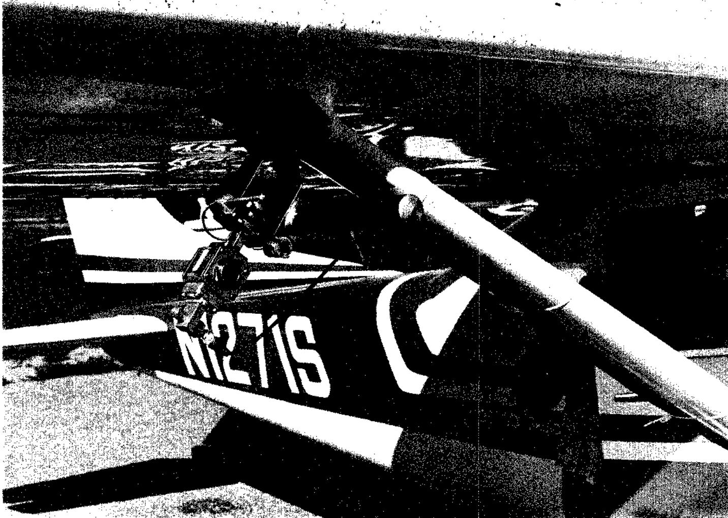
Figure 3-8. Single engine aircraft equipped to make simultaneous measurements of refractivity, temperature, and pressure.
