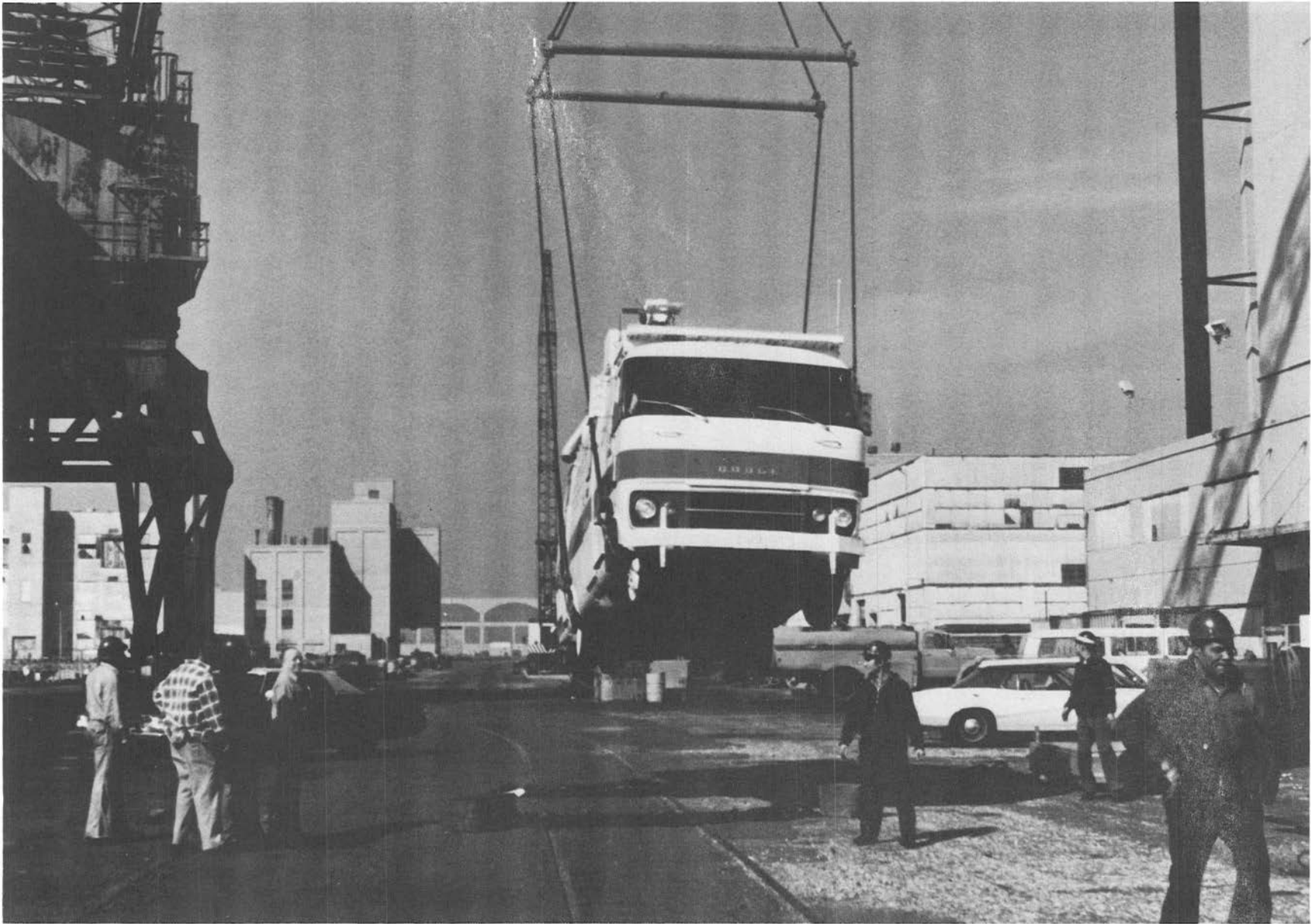
Figure 1-22. RSMS being raised to top of building for New York measurements.
