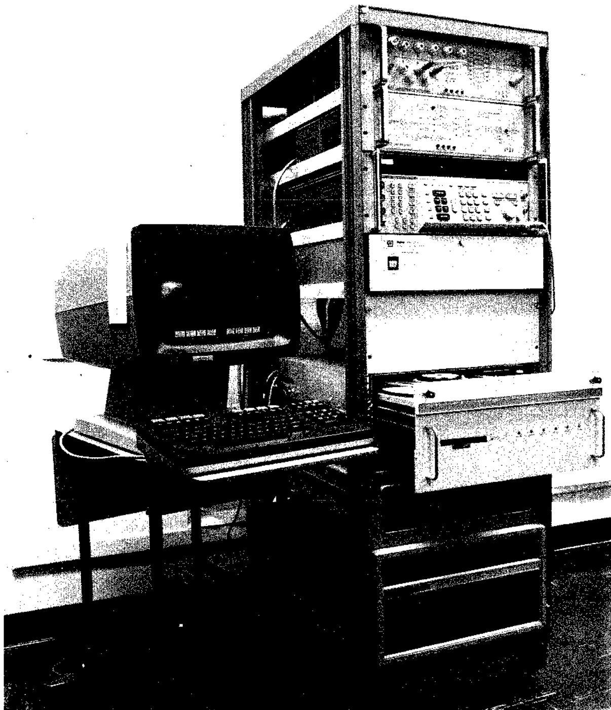
Figure 1-7. Upgraded LMR measurement system (configured as one rack and terminal).
