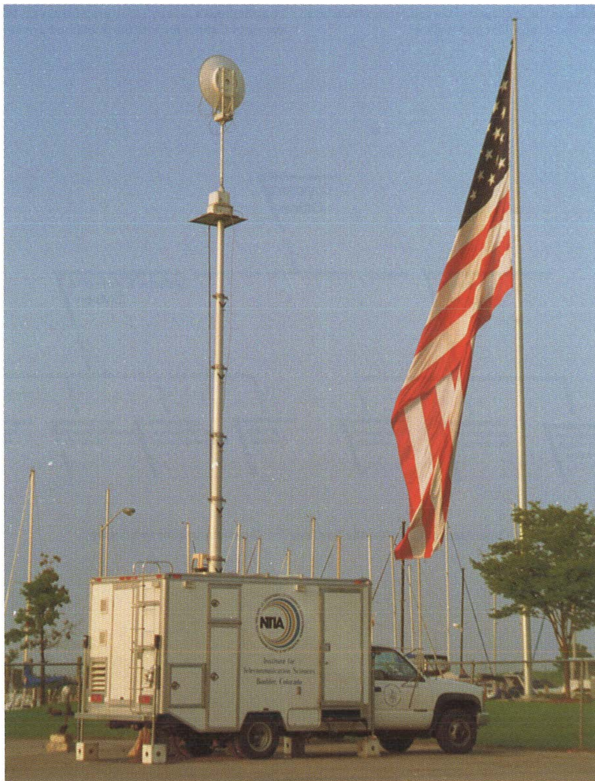
Radio Spectrum Measurement System Van Performing a Spectrum Survey near the Kent Narrows Bridge in Maryland, Virginia. See RSMS Spectrum Surveys, Page 12. Photograph by F. Sanders.
