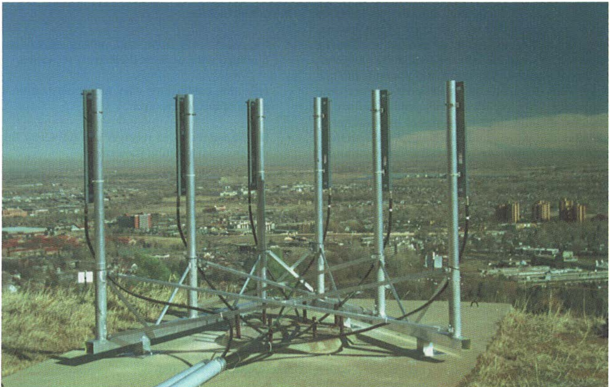
Antenna of a PCS System Under Test on Enchanted Mesa West of the Department of Commerce Boulder Labs (visible at the lower right). Photograph by F Sanders.
