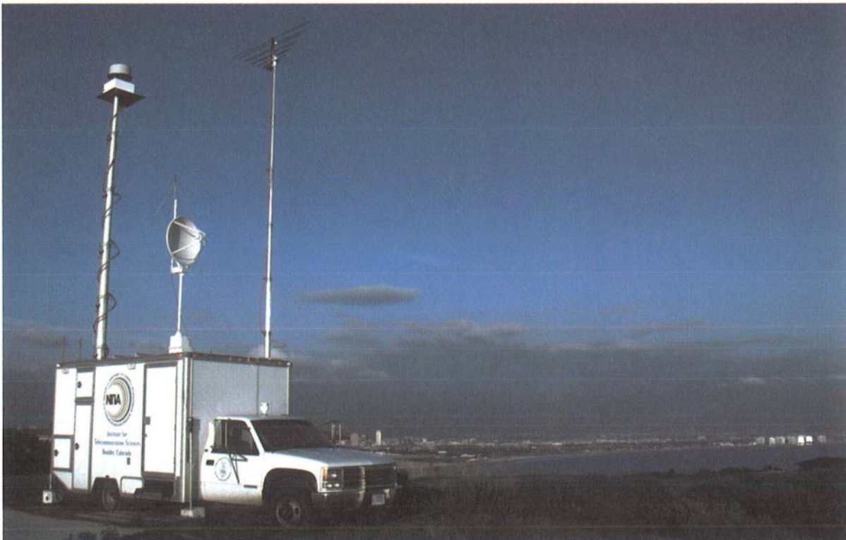
Figure 1. RSMS during a spectrum survey at Point Loma near San Diego, California (photograph by F. Sanders).
