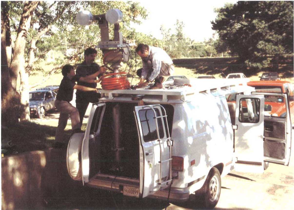
Radio research measurement van configured for a 30-GHz local multipoint distribution services propagation study. This vehicle, equipped with a GPS dead-reckoning system, is used for mobile cellular radio, PCS, and millimeter-wave measurement studies (photograph by F. Sanders).
