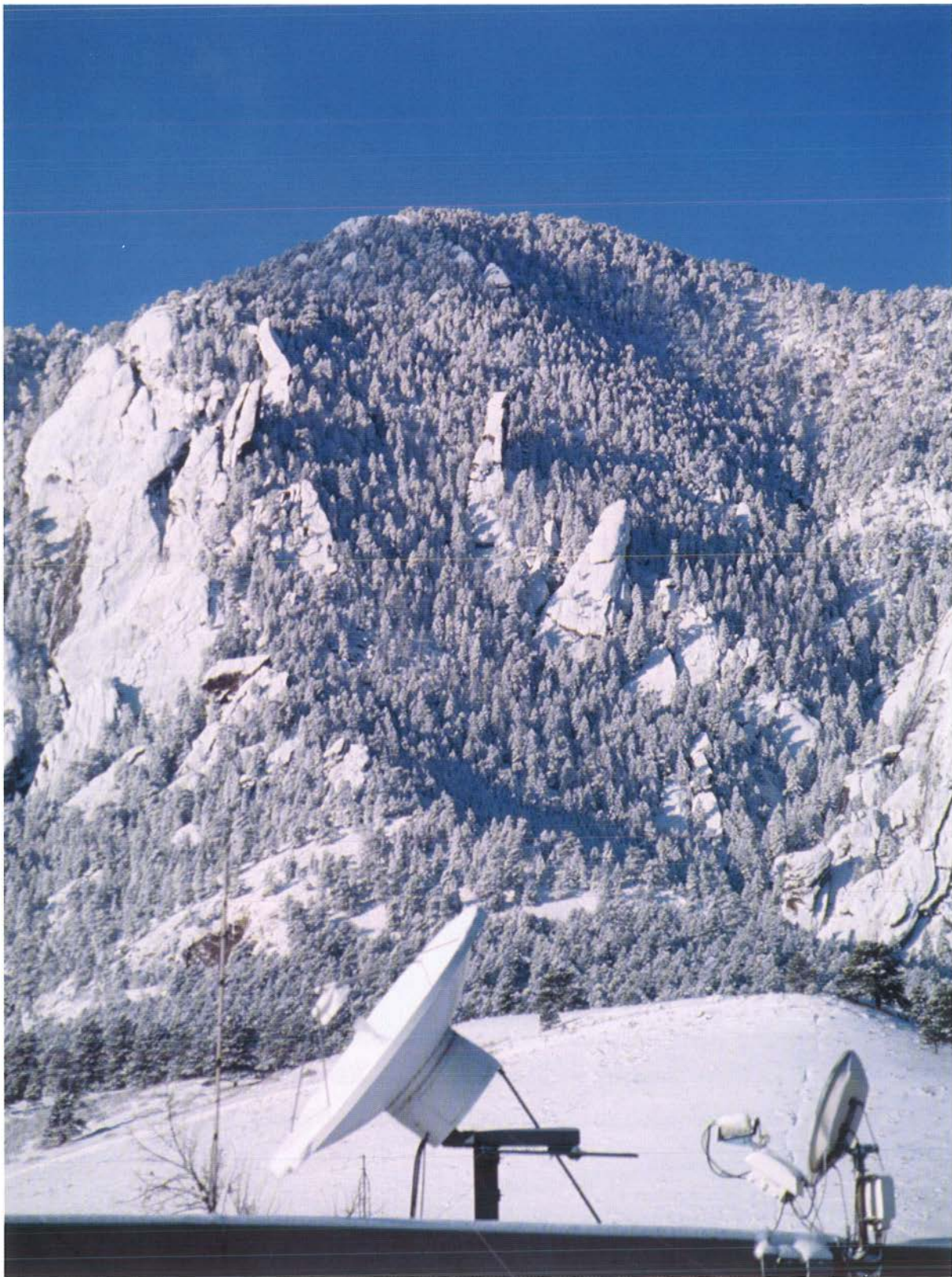
The C/Ku band antenna (left) and Advanced Communications Satellite Technology antenna (right) are used for performance testing of satellite systems and the voice, video, and data services they transport (photograph by D.J. Atkinson).
