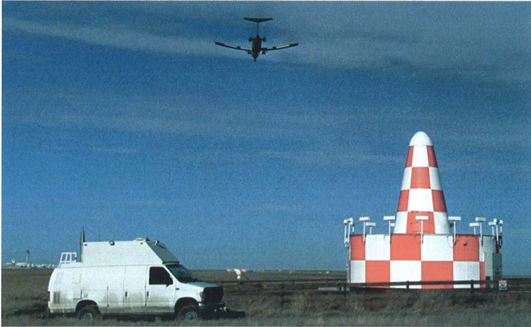
Figure 1. RFIMS van at an FAA navigation beacon facility. RFIMS van used four-wheel drive capability to negotiate deep mud and bring the measurement system to this location (photograph by F.H. Sanders).
