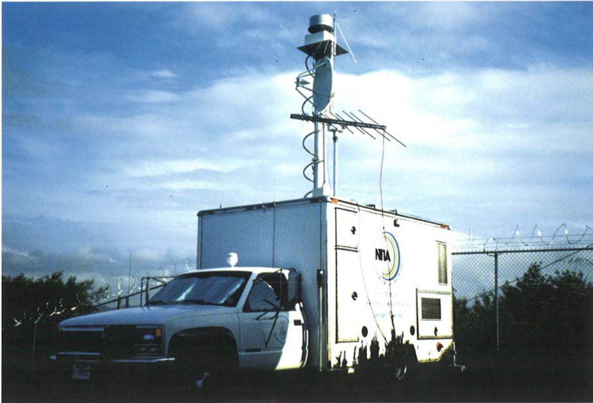
Measurements being performed while the ITS radio spectrum measurement system is transmitting simulated spaceborne radar signals into an air-traffic control radar (photograph by F.H. Sanders).
