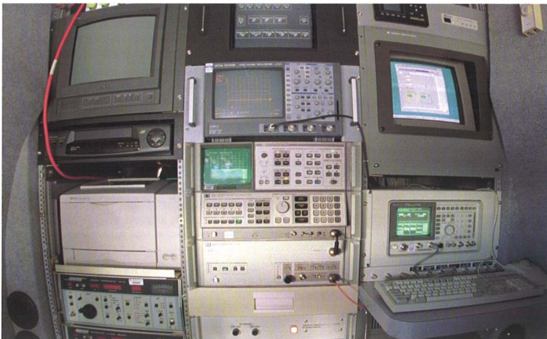
Figure 2. The interior of the RFIMS van, showing the layout of the integrated electronics package monitoring equipment mounted in three 6-ft racks (photograph by F.H. Sanders).
