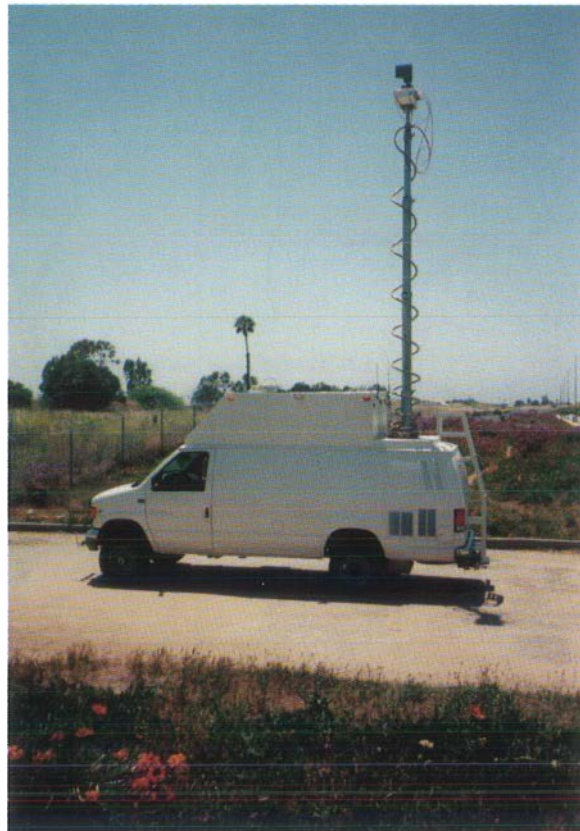
Figure 1. Prototype RFIMS at Los Angeles International Airport (photograph by P. Raush).
