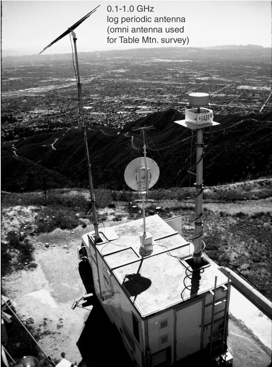
Figure 5. Illustration of the RSMS with telescoping masts raised and antennas mounted for a broadband spectrum survey such as was performed at the Table Mountain NRQZ.
