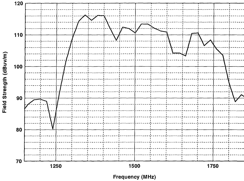
Figure D.B.5. Device B, radiated peak field strength at 1 m, \Delta f = 20 MHz.
