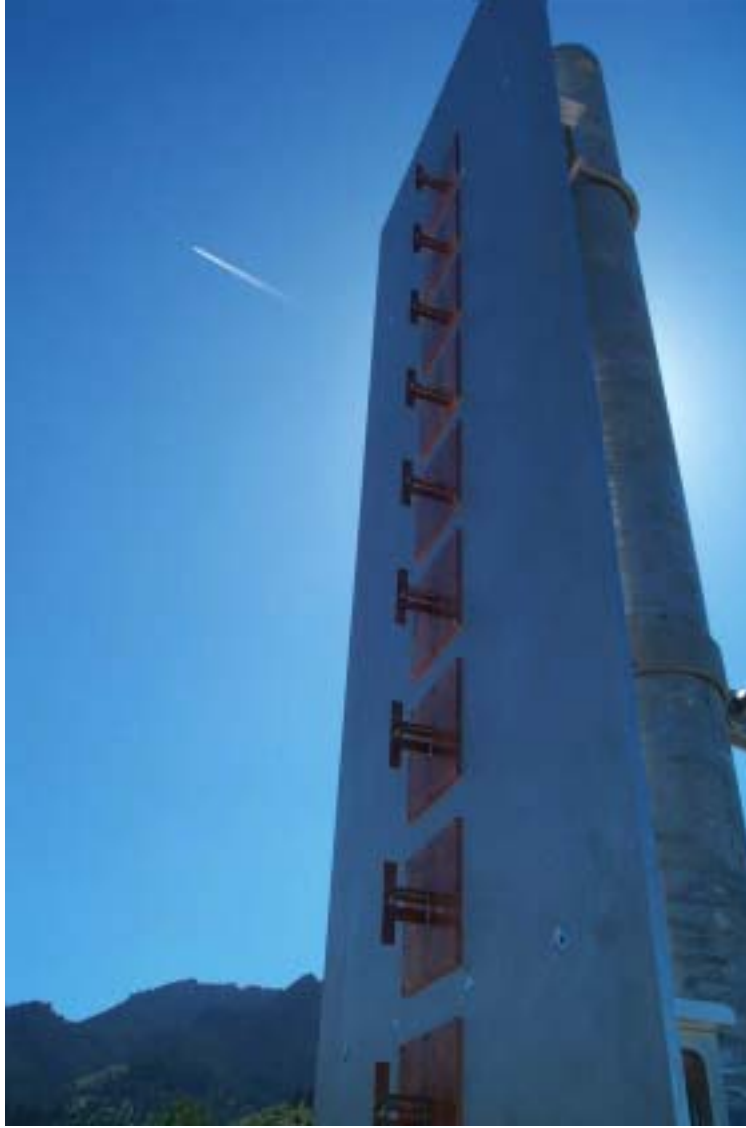
Figure 8. Dipole antenna elements in vertical array.
