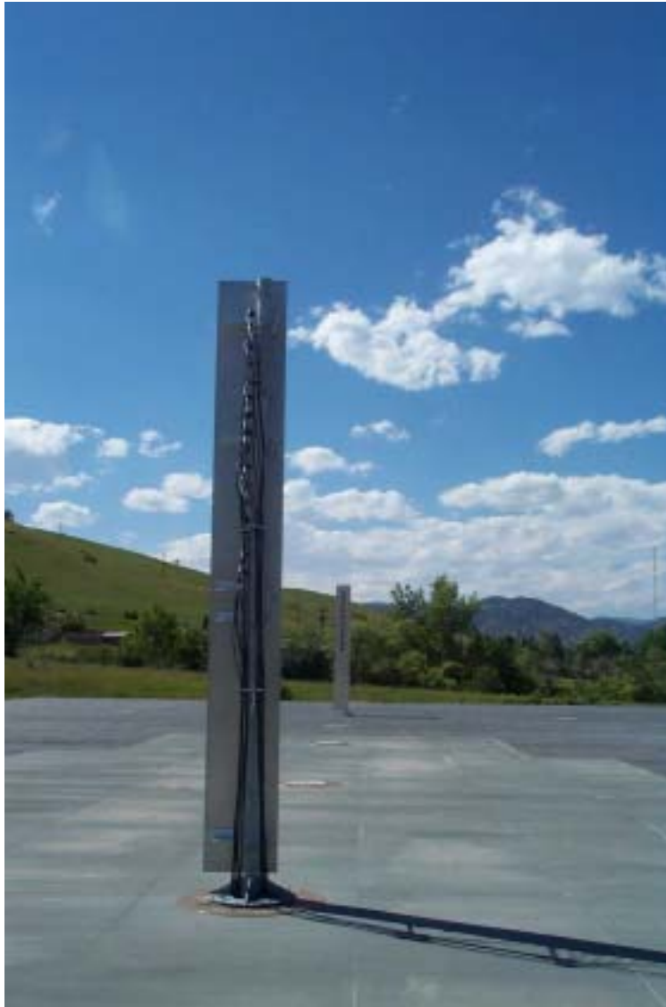
Figure 7. Antenna arrays on ground plane, the closer array is the receiving antenna. The antenna elements are shown in Figure 8.
