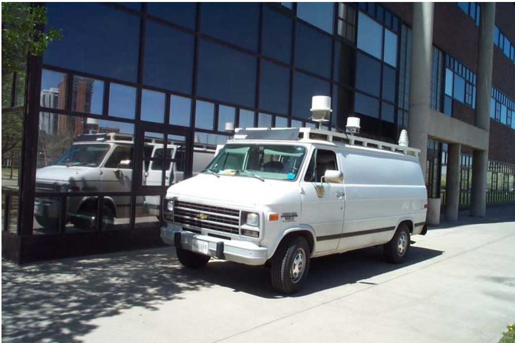
Figure 6. The measurement van, ground plane and receiving antennas.
