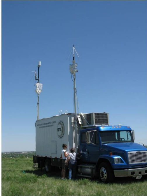
Figure B-1. RSMS-4 measurement truck with mast-mounted antennas and preselector units.
