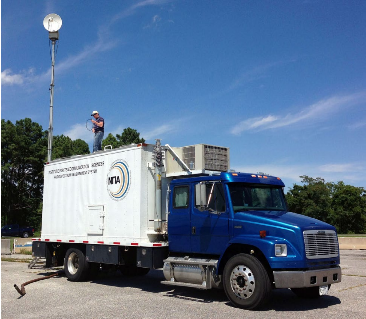
Figure 2. NTIA RSMS-4 measuring Shipborne Radar 1 radiated emissions in Maryland.
