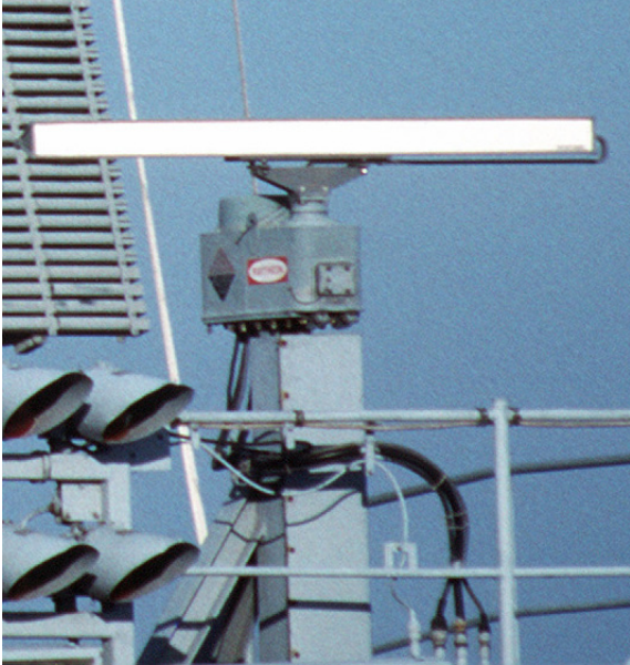
Figure 1. Marine radar slotted array antenna (white bar) mounted on motor which spins it.
