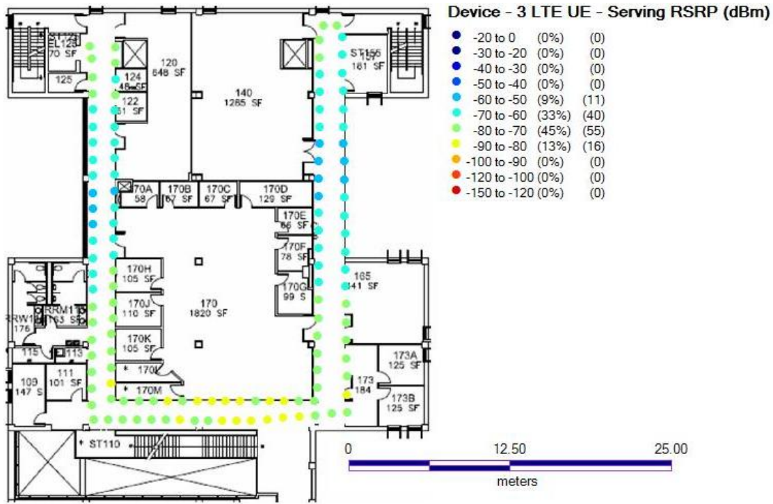
Figure 84. Level 1 reference signal received power (RSRP) for a TCP downlink data flow with a small cell feeding a four-antenna DAS system. The direction of top of the floor plan is north.
