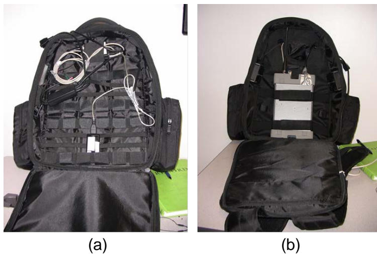
Figure 12. Backpack walk testing system with (a) LTE modem and (b) a scanner/receiver.
