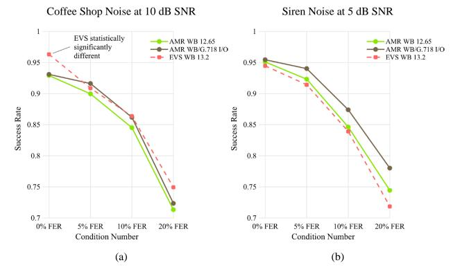
Figure 1. Word success rates for three codec modes in (a) coffee shop noise at 10 dB SNR and (b) siren noise at 5 dB SNR.
