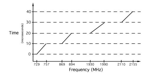
Figure 1. Jammer LFM behavior. The complete chirp sequence, across all bands, was repeated every 40 microseconds. Frequencies are plotted to a non-fixed scale.
