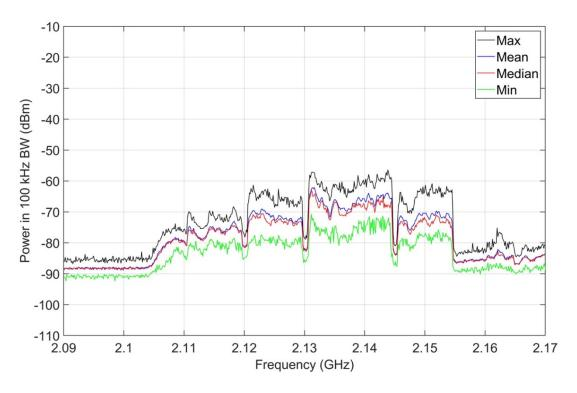
Figure 26. M4 statistics, jammer on, 2090-2170 MHz, outdoor location O-2.
