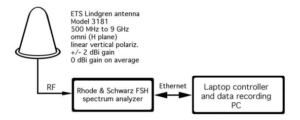
Figure 3. Block diagram schematic of the jammer emission measurement system used at Broad River Correctional Institution.
