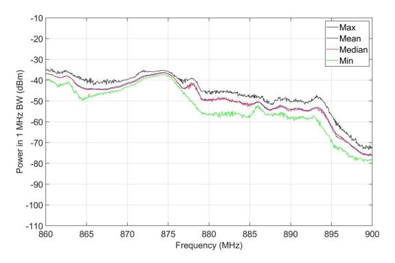
Figure A-19. M4 statistics, jammer on, 860-900 MHz, outdoor location O-2.
