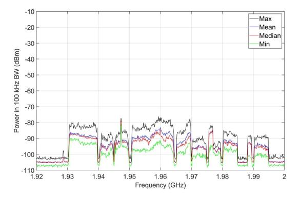
Figure 9. M4 statistics, jammer off, 1920-2000 MHz, inside targeted prison housing block.
