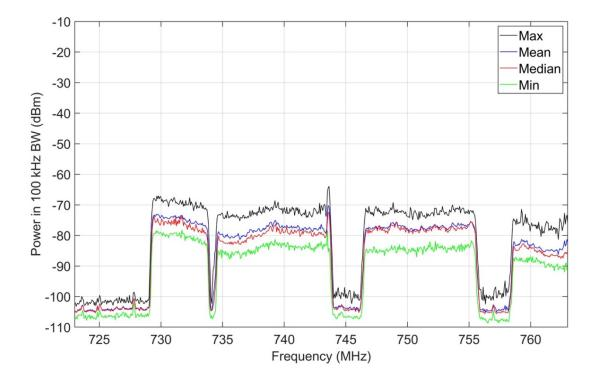
Figure 5. M4 statistics, jammer off, 723-763 MHz, inside targeted prison housing block.
