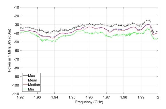
Figure A-5. M4 statistics, jammer on, 1920-2000 MHz, inside targeted housing unit.
