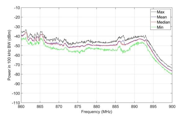
Figure 6. M4 statistics, jammer on, 860-900 MHz, inside targeted prison housing block.
