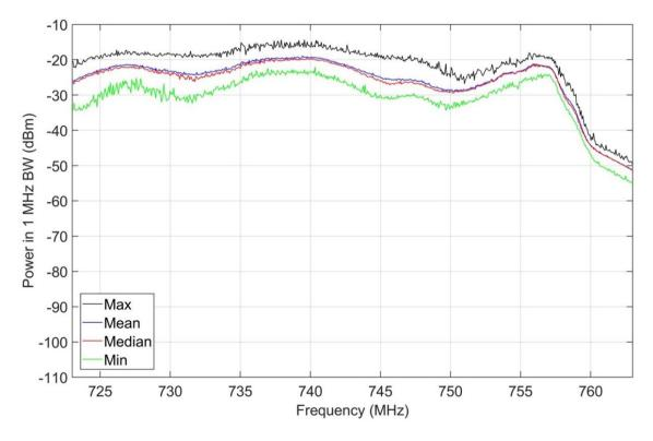
Figure A-1. M4 statistics, jammer on, 723-763 MHz, inside targeted housing unit.
