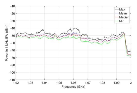
Figure A-13. M4 statistics, jammer on, 1920-2000 MHz, outdoor location O-1.
