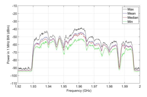
Figure A-14. M4 statistics, jammer off, 1920-2000 MHz, outdoor location O-1.
