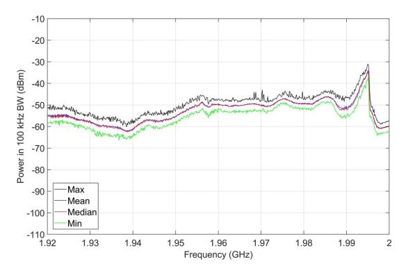
Figure 8. M4 statistics, jammer on, 1920-2000 MHz, inside targeted prison housing block.
