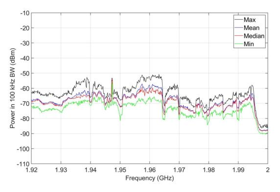
Figure 16. M4 statistics, jammer on, 1920-2000 MHz, outdoor location O-1.
