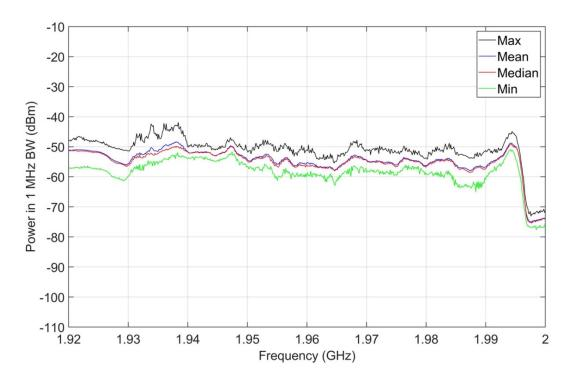
Figure A-21. M4 statistics, jammer on, 1920-2000 MHz, outdoor location O-2.
