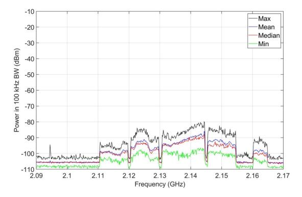
Figure 11. M4 statistics, jammer off, 2090-2170 MHz, inside targeted prison housing block.
