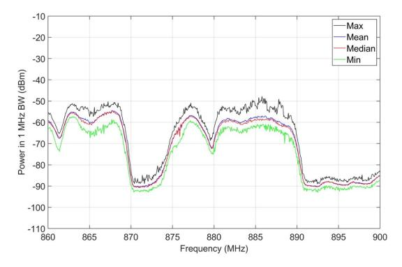
Figure A-12. M4 statistics, jammer off, 860-900 MHz, outdoor location O-1.
