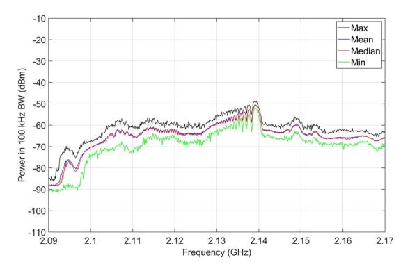
Figure 10. M4 statistics, jammer on, 2090-2170 MHz, inside targeted prison housing block.
