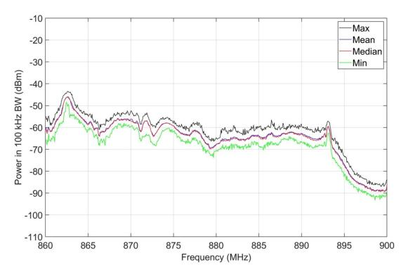
Figure 14. M4 statistics, jammer on, 860-900 MHz, outdoor location O-1.
