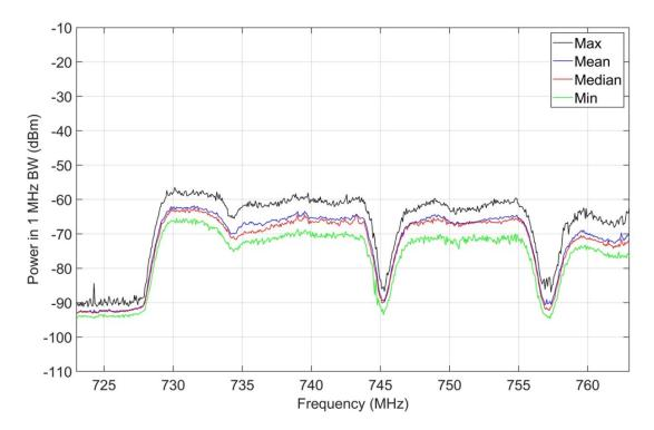
Figure A-2. M4 statistics, jammer off, 723-763 MHz, inside targeted housing unit.
