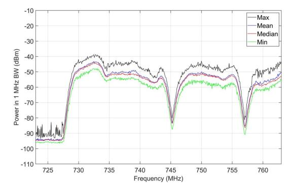
Figure A-18. M4 statistics, jammer off, 723-763 MHz, outdoor location O-1.
