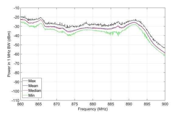
Figure A-3. M4 statistics, jammer on, 860-900 MHz, inside targeted housing unit.
