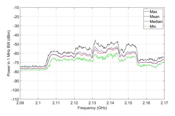
Figure A-23. M4 statistics, jammer on, 2090-2170 MHz, outdoor location O-2.
