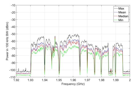
Figure 25. M4 statistics, jammer off, 1920-2000 MHz, outdoor location O-1.
