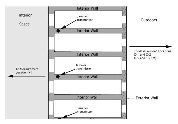
Figure 2. The Broad River jammer installation top view, approximately scaled. Seven jammers were spaced every other cell, in utility shafts, on each of two floors. Only one jammer on the ground floor was operated for the measurements.
