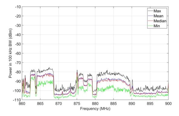
Figure 7. M4 statistics, jammer off, 860-900 MHz, inside targeted prison housing block.
