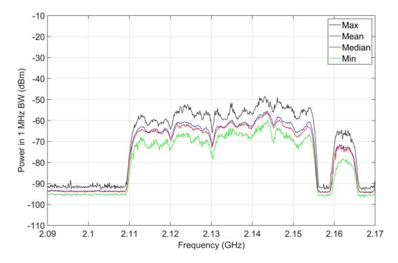
Figure A-24. M4 statistics, jammer off, 2090-2170 MHz, outdoor location O-1.
