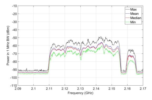
Figure A-16. M4 statistics, jammer off, 2090-2170 MHz, outdoor location O-1.
