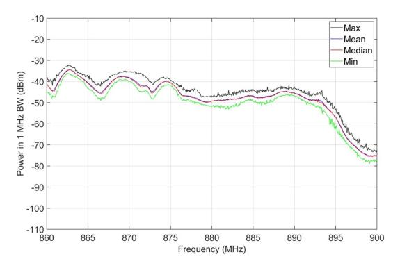
Figure A-11. M4 statistics, jammer on, 860-900 MHz, outdoor location O-1.
