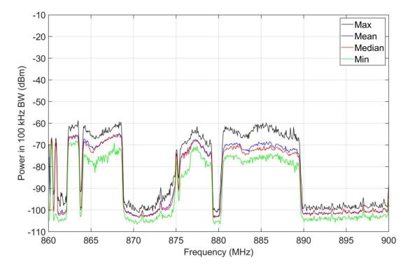
Figure 15. M4 statistics, jammer off, 860-900 MHz, outdoor location O-1.
