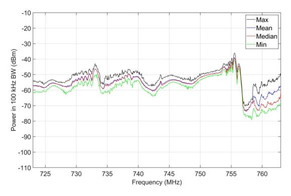
Figure 12. M4 statistics, jammer on, 723-763 MHz, outdoor location O-1.
