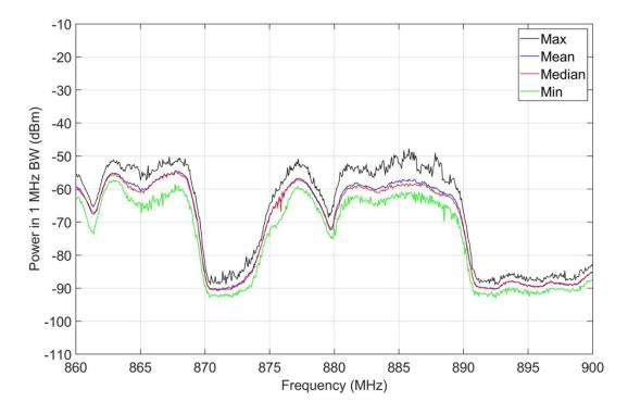
Figure A-20. M4 statistics, jammer off, 860-900 MHz, outdoor location O-1.
