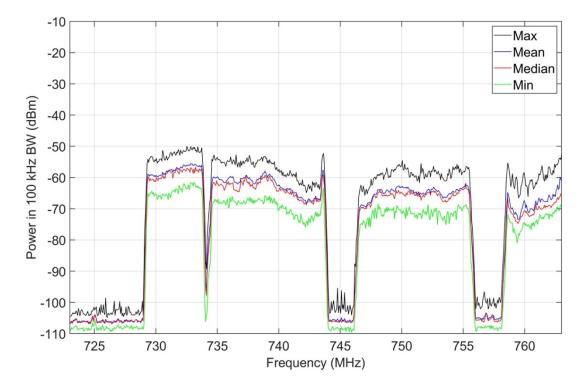
Figure 21. M4 statistics, jammer off, 723-763 MHz, outdoor location O-1.
