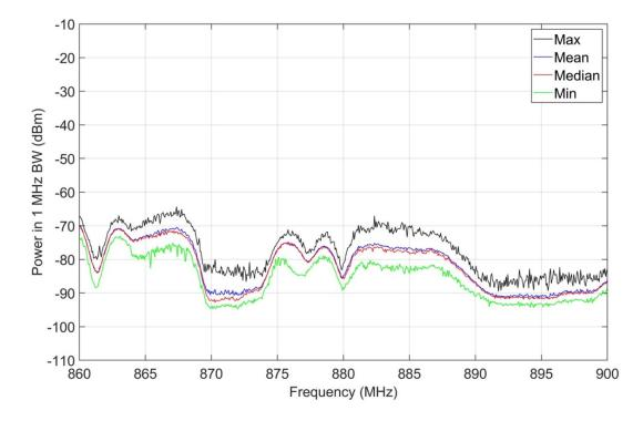
Figure A-4. M4 statistics, jammer off, 860-900 MHz, inside targeted housing unit.
