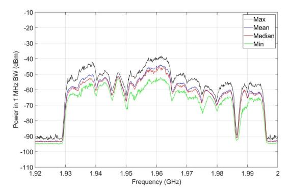
Figure A-22. M4 statistics, jammer off, 1920-2000 MHz, outdoor location O-1.
