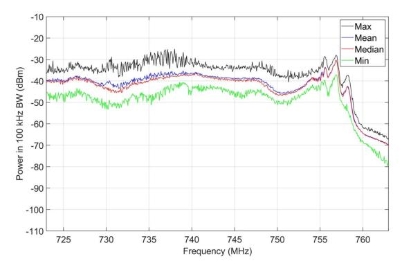
Figure 4. M4 statistics, jammer on, 723-763 MHz, inside targeted prison housing block.
