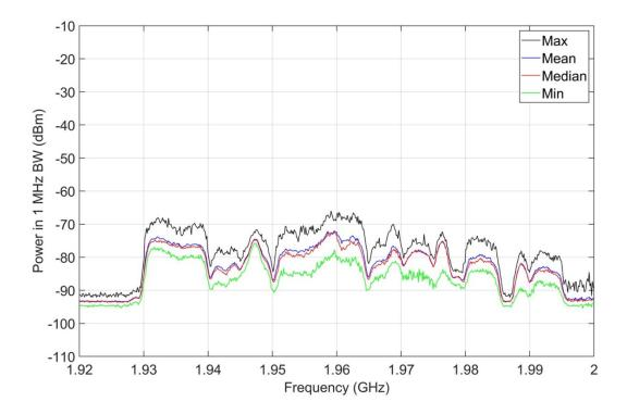
Figure A-6. M4 statistics, jammer off, 1920-2000 MHz, inside targeted housing unit.
