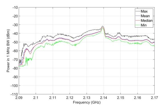
Figure A-7. M4 statistics, jammer on, 2090-2170 MHz, inside targeted housing unit.
