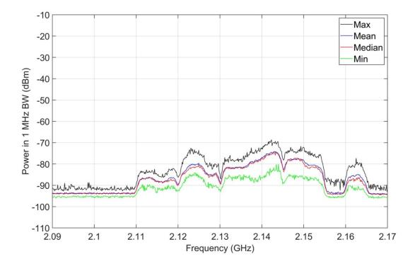
Figure A-8. M4 statistics, jammer off, 2090-2170 MHz, inside targeted housing unit.
