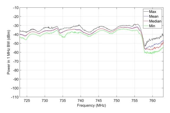
Figure A-9. M4 statistics, jammer on, 723-763 MHz, outdoor location O-1.
