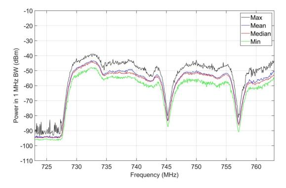
Figure A-10. M4 statistics, jammer off, 723-763 MHz, outdoor location O-1.
