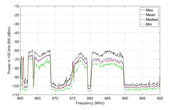
Figure 23. M4 statistics, jammer off, 860-900 MHz, outdoor location O-1.
