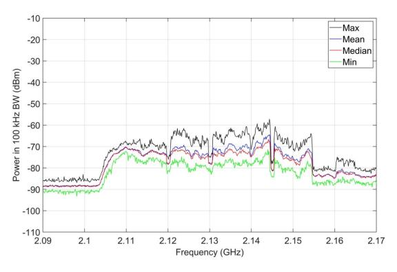
Figure 18. M4 statistics, jammer on, 2090-2170 MHz, outdoor location O-1.
