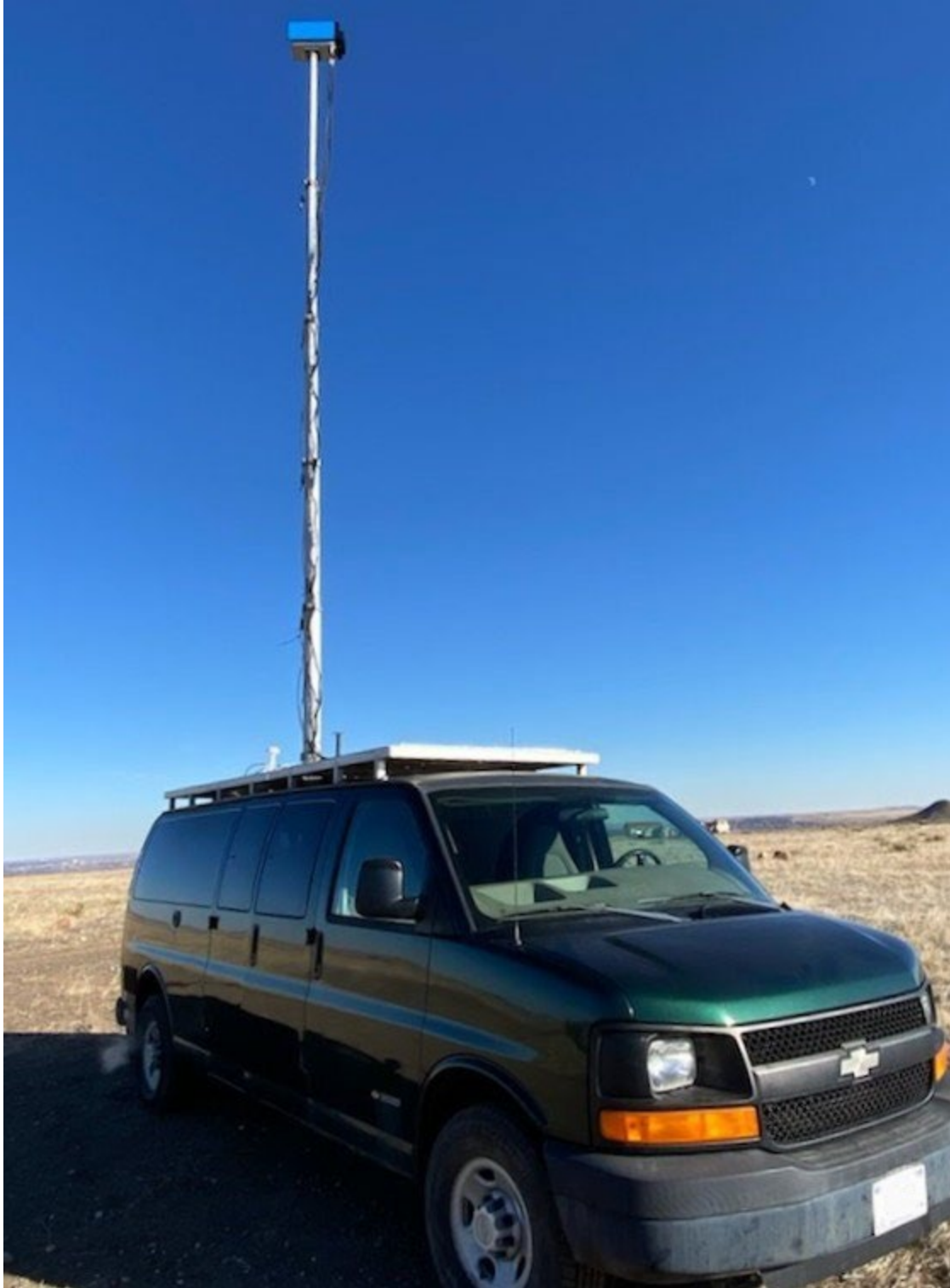
Figure 2. Measurement system transmitter vehicle: ITS modified Chevrolet Express 3500 extended cargo van with 9 m (30 ft.) telescoping mast.
