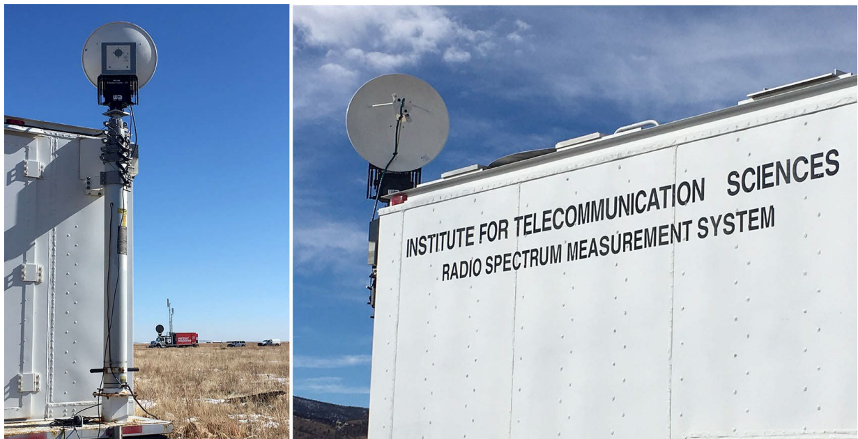
Figure 38. RSMS-5G measurement antenna (front & back) with a target 5G MIMO CoLT in the background, at 161 m distance. RSMS antenna heights were between 4 m (13 ft) and 5.8 m (19 ft) AGL, depending on circumstances. MIMO arrays were at ~10 m (33 ft) AGL. (A UE is on the rear platform at the base of the mast.)
