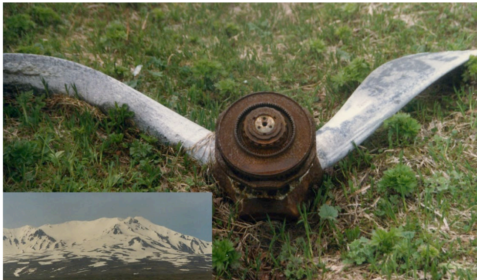
Figure 2. Propeller of a WW II aircraft that flew, under control, into Mt. Moffett (inset), Adak, Alaska in low visibility conditions where height-above-ground information was lacking (no radalt), according to records of the 1990 Adak Naval Air Station historian. Photos by F. Sanders.
