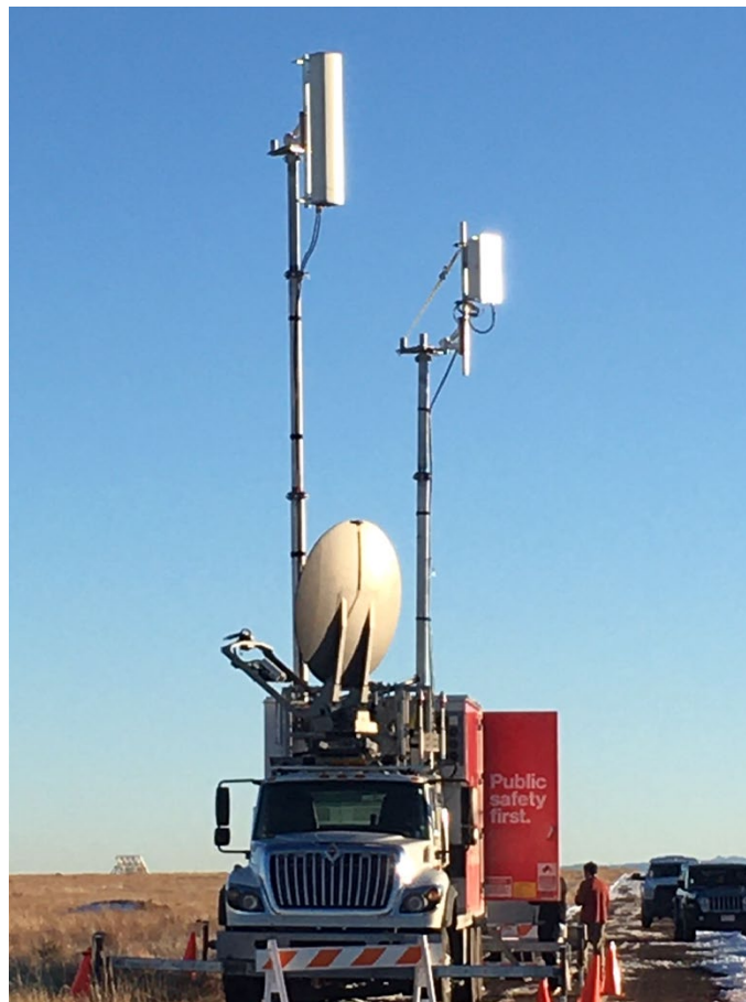
Figure 30. An upper C-band (3700–3980 MHz) CoLT deployed at Table Mtn. The US 5G n77 band MIMO array is at right. Support links are a Ku-band (14 GHz) satellite dish and a UHF (700 MHz) LTE panel (upper left).
