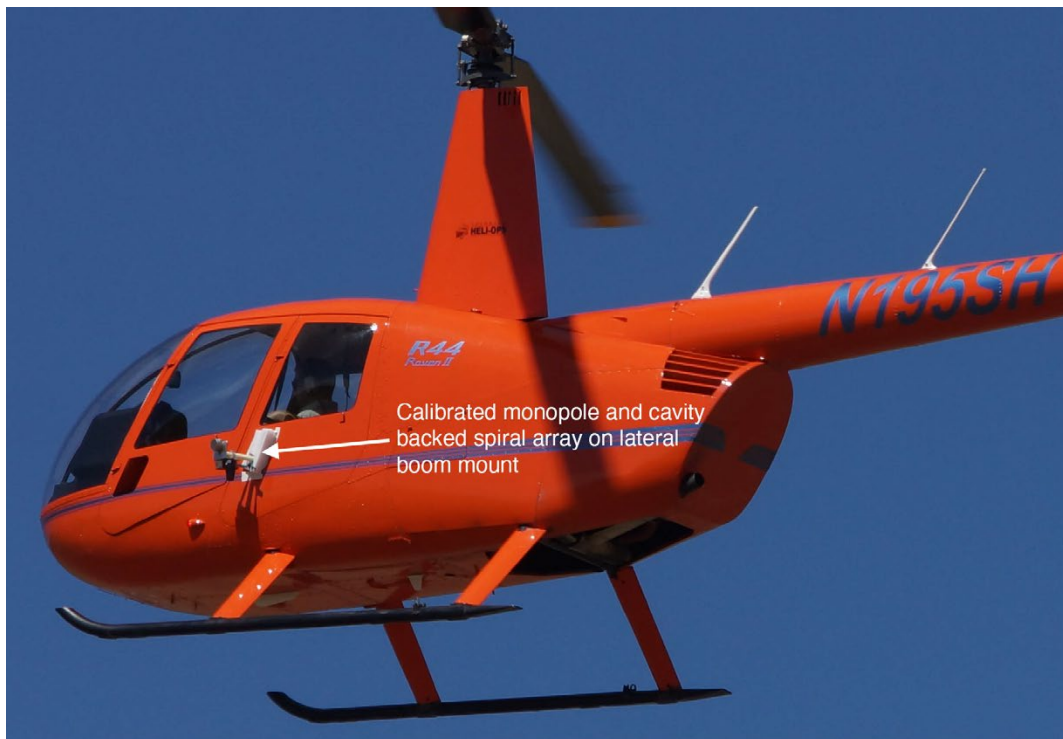
Figure 42. Measurement antenna configuration on Raven R-44 for 5G airborne field strength measurements on Radios 2–4 (upper C-band MIMO arrays).
