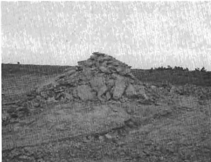
Figure 46. Site A, test 7. The antenna is covered by 1.0 m of broken rock.
