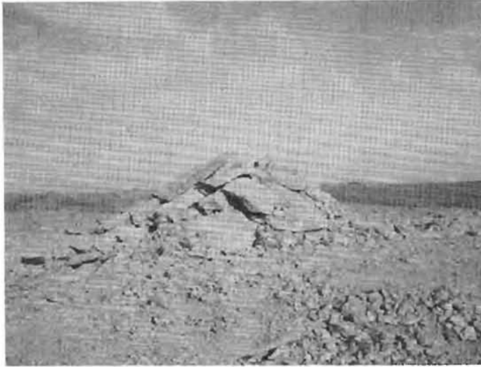
Figure 45. Site A, test 7. The antenna is covered by 0.6 m of broken rock.
