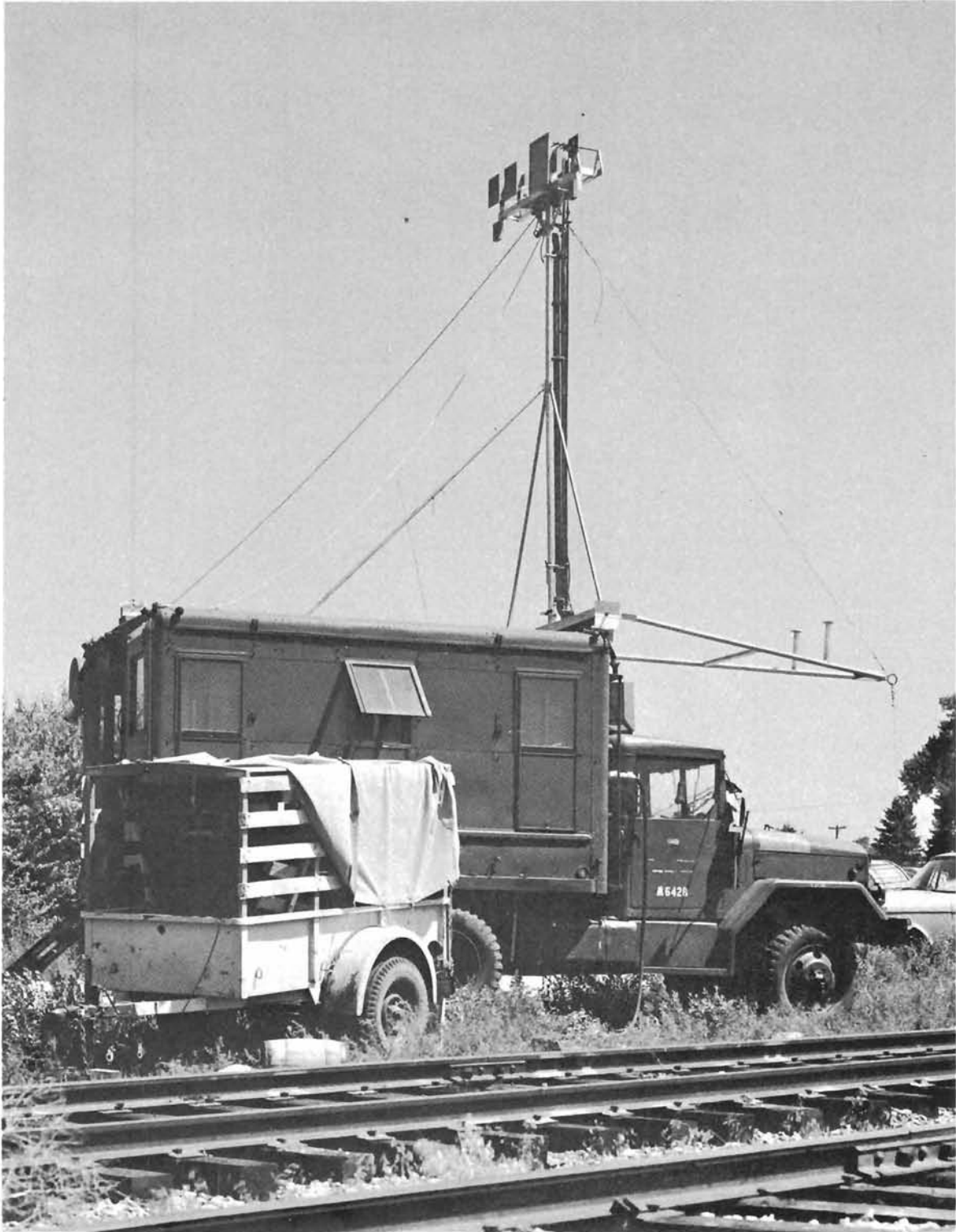
Figure 9. Upper frequency group transmitting unit.
