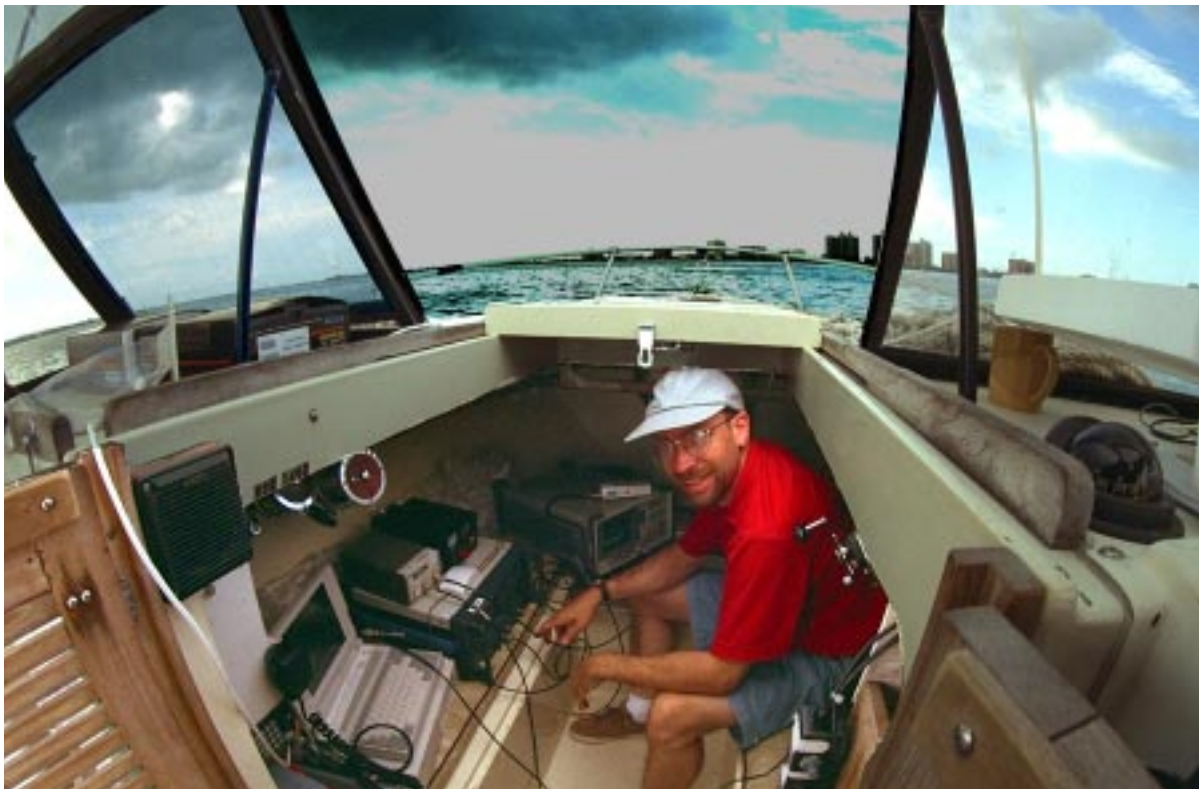
Figure 1. Electromagnetic compatibility measurements in progress on board a boat in Tampa Bay. The measurements determined interference characteristics of new maritime radios that operate with channels only half as wide as currently available radios (photograph by F.H. Sanders).
