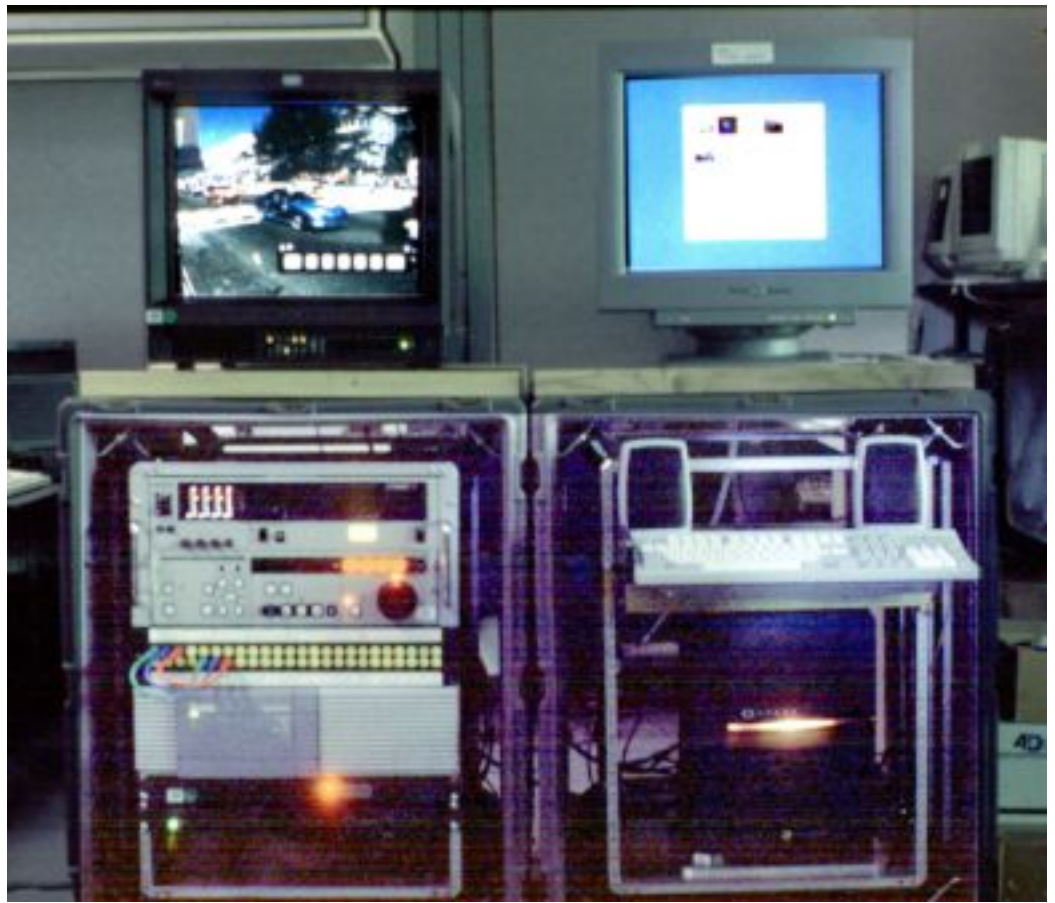
Figure 2. Transportable Video Quality Measurement System (TVQMS) ready to perform digital video quality measurements.
