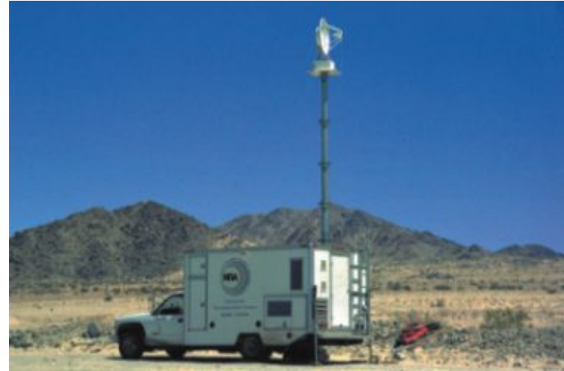
Figure 1. ITS Radio Spectrum Measurement System (RSMS) van at Twentynine Palms, CA, performing emission spectrum measurements on Marine Corps TPS-59 radar transmitter. Radar is approximately one-quarter mile away; measurement antenna is raised on telescoping mast to avoid nearby terrain and structural obstacles (photograph by F.H. Sanders).
