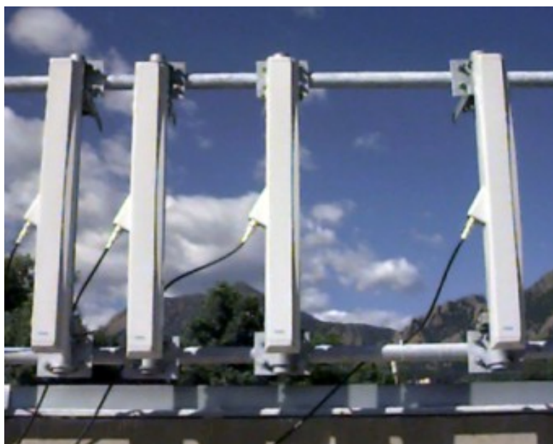
Figure 1. A four element antenna array. The elements are spaced 2, 5, and 10 \lambda with respect to the left end element (photograph by F.H. Sanders).
