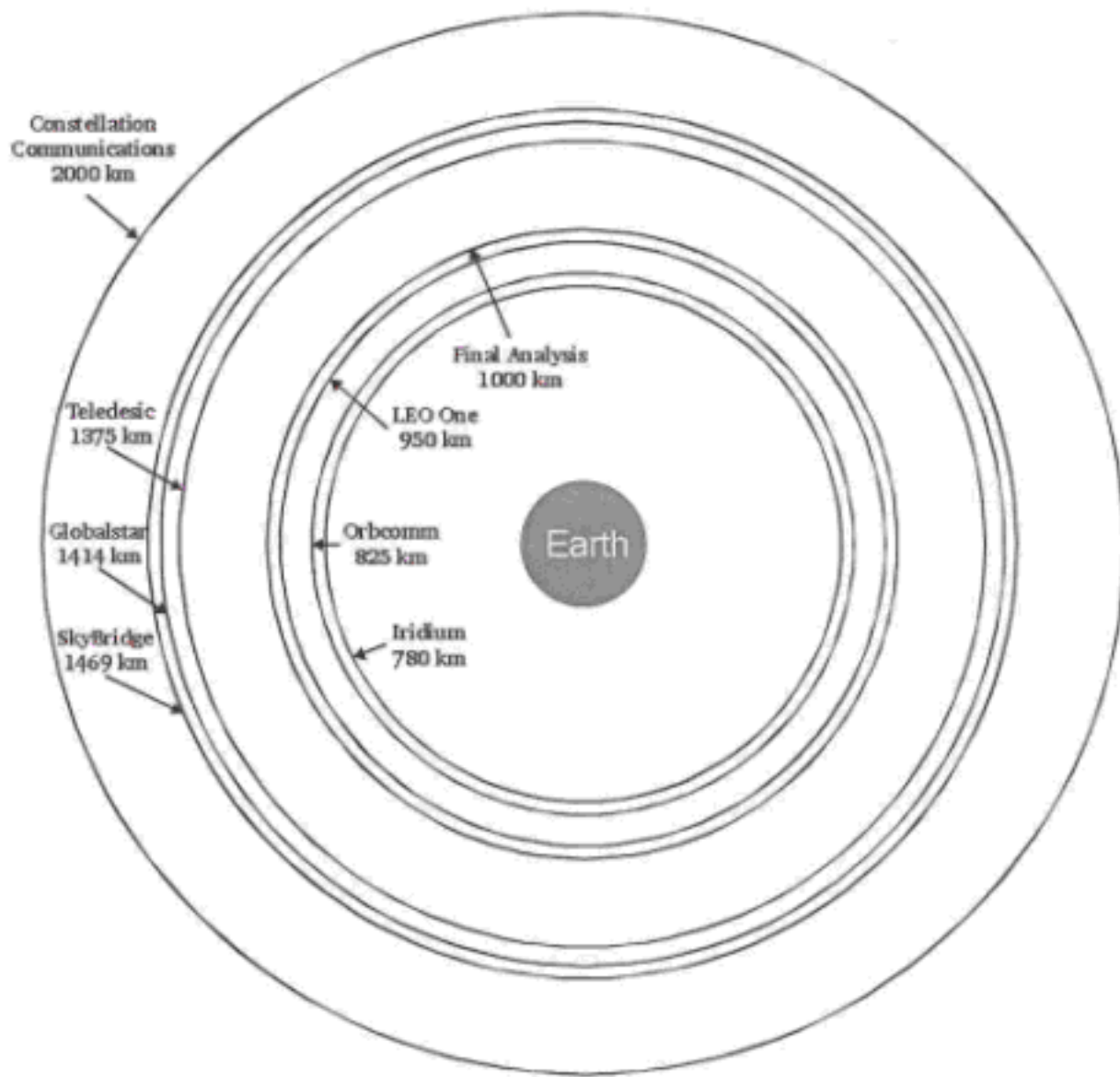
Figure 2. Orbital altitudes of some commercial low earth orbit (LEO) satellite systems.
