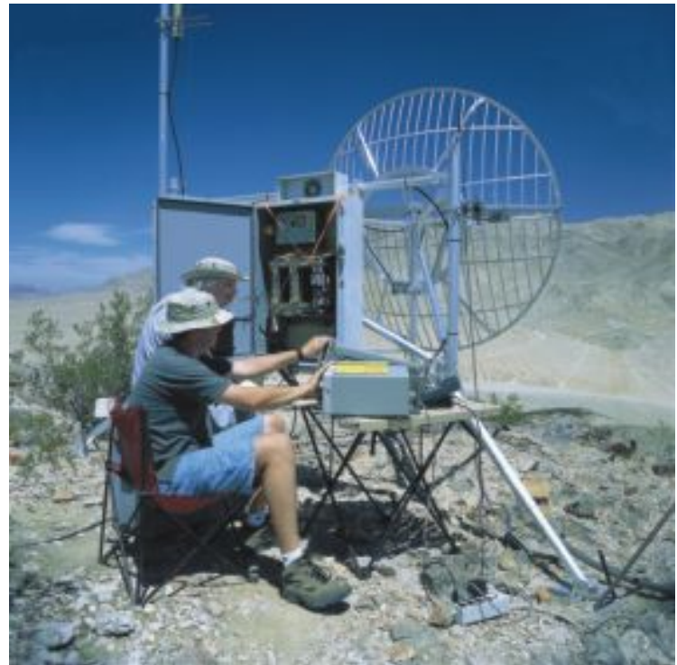
ITS engineers perform measurements on a radio communication link at a remote desert location in southern California. These measurements were intended to isolate reported interference to the link from cellular telephone transmitters (photograph by F.H. Sanders).
