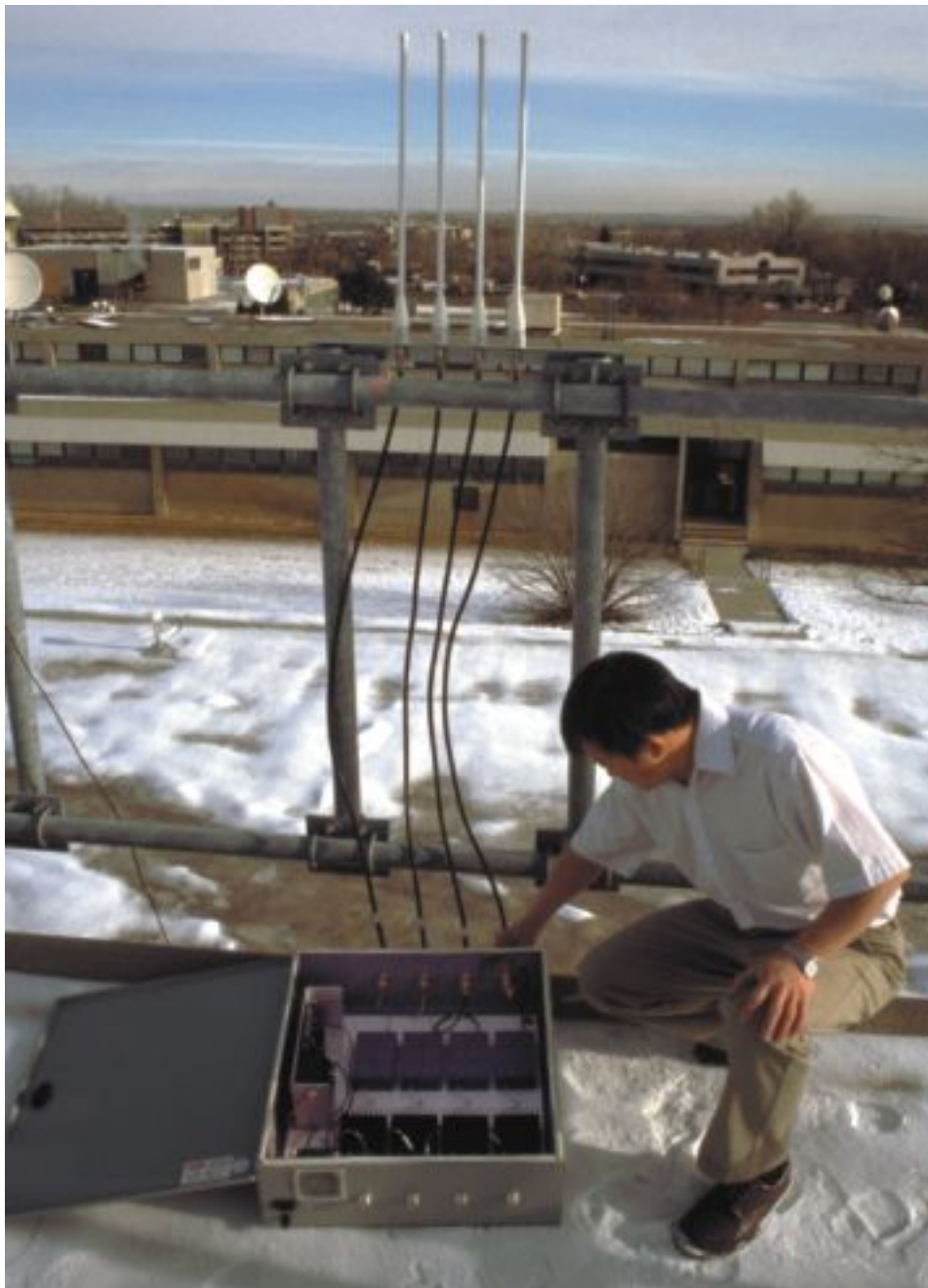
An ITS engineer adjusts a four-channel preselector-preamplifier box used as part of the ITS antenna testbed (photograph by F.H. Sanders).
