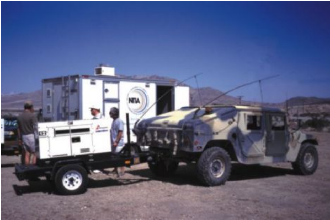
Figure 3. Convoy of ITS RSMS van, U.S. Army high mobility multipurpose wheeled vehicle (HMMWV), and towed power-supply generator prepares to leave base area at Ft. Irwin, CA for a measurement location in the desert. The RSMS crew camped on the range with the van and performed broadband spectrum occupancy measurements during a week-long military exercise at that facility (photograph by F.H. Sanders).
