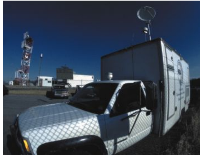
The ITS Radio Spectrum Measurement System (RSMS) transmitting simulated satellite-radar signals into a nearby air traffic control (ATC) radar at Linthicum, MD. These tests determined levels at which such satellite signals would interfere with ATC radar operations (photograph by F.H. Sanders).
