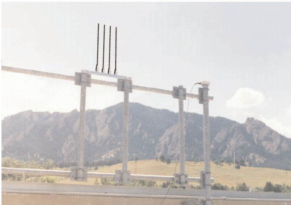
Figure 1. A four element antenna array. The elements are spaced at \lambda/2 intervals (photograph by P. Papazian and E. Gray).
