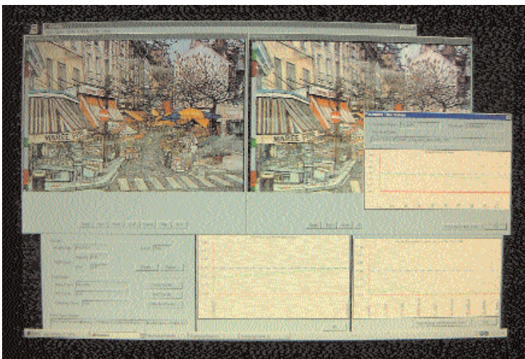
Figure 4. User display presented by Windows-based video quality measurement system (photograph by F.H. Sanders).
