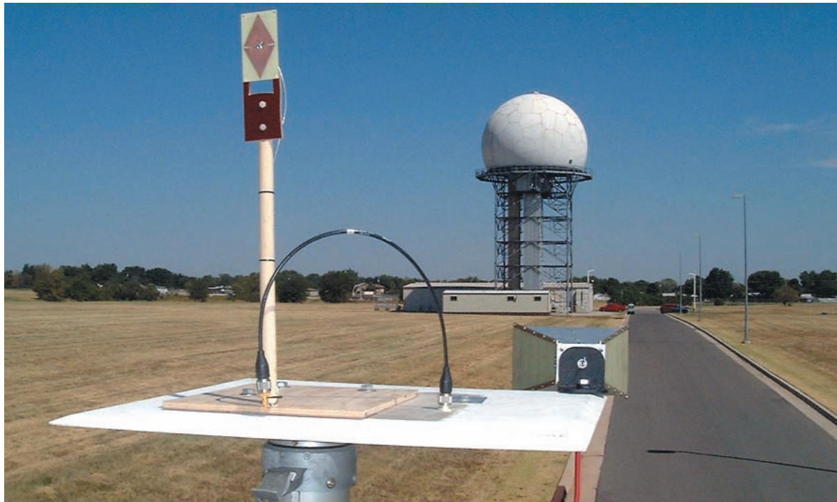
Figure 1. An ultrawideband (UWB) transmitter antenna mounted on top of a mast on the Radio Spectrum Measurement System (RSMS) van with an ARSR-4 radar tower in the background. The UWB transmitter emission effects were monitored at the ARSR-4 receiver (photograph by F.H. Sanders).
