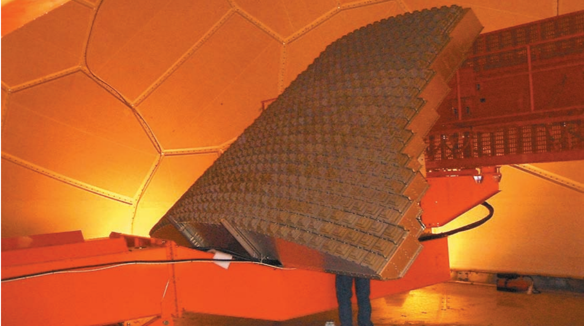
Figure 2. The ARSR-4 radar antenna feed, which received the UWB emissions transmitted from the RSMS system shown in Figure 1 (photograph by F.H. Sanders).
