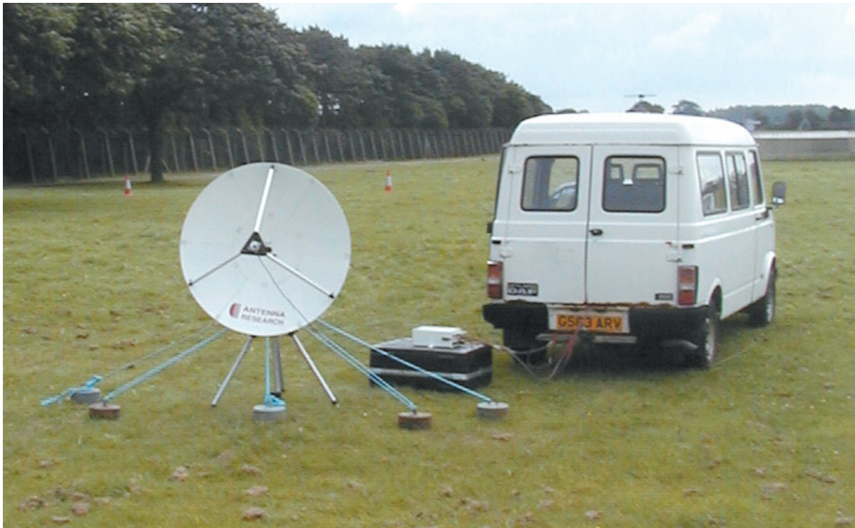
Figure 1. ITS measurements in progress on maritime surface-search and navigation radars at a Ministry of Defense facility at Funtington, UK. A suitcase version of the Radio Spectrum Measurement System (RSMS) was used inside the loaned van. The collapsible parabolic antenna is trained on radars, located about 1/8 mile away (photograph by F.H. Sanders).
