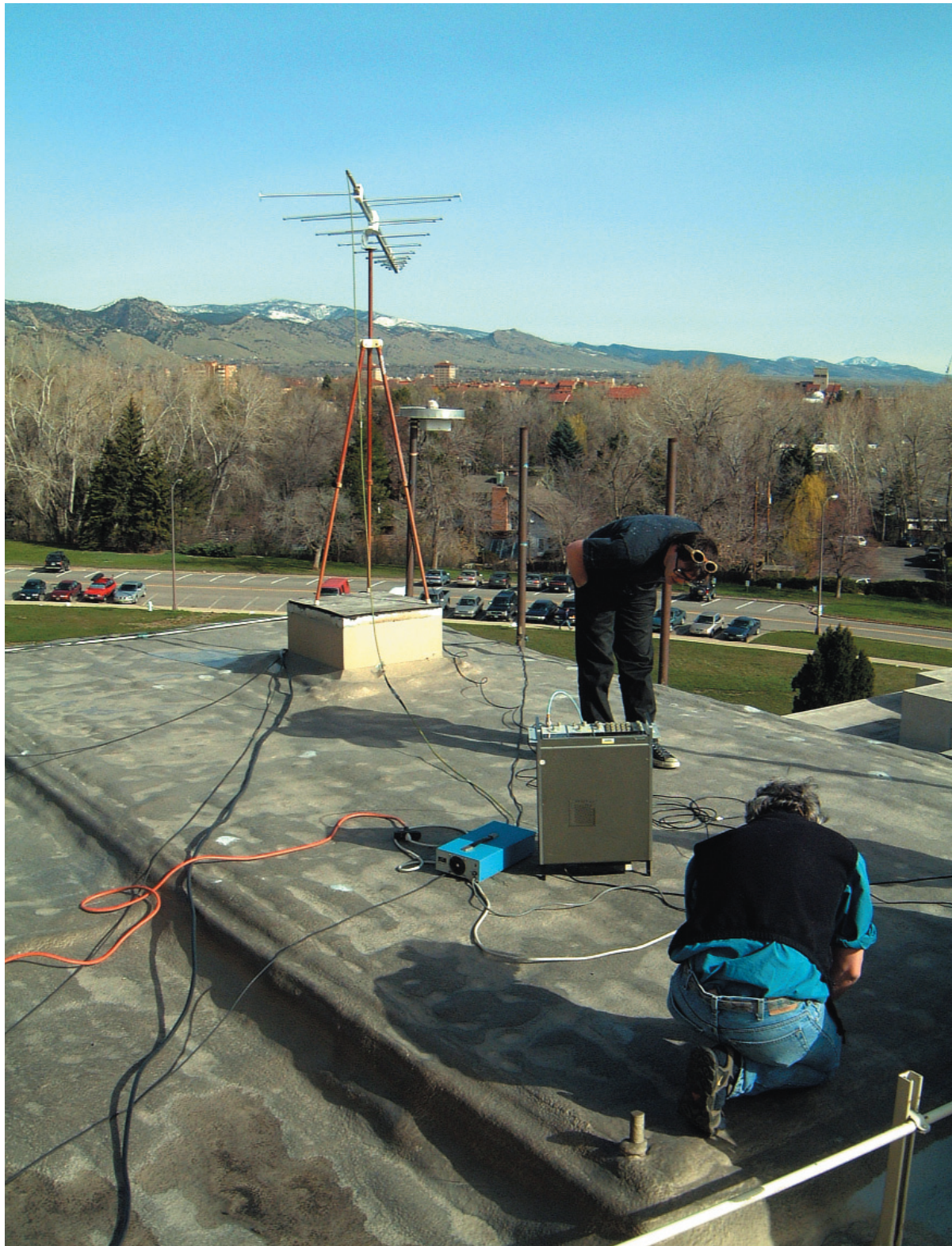
Measurements performed on the roof of the main building at the DOC Boulder Laboratories. Researchers are testing the effects of various E-field strengths on GPS receivers (photograph by F.H. Sanders).
