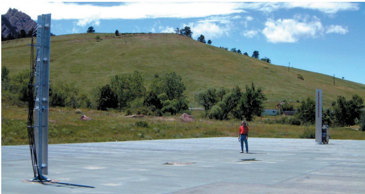
Figure 1. 16-element transmit and receive arrays used for multiple input, multiple output (MIMO) testing at the NIST open area test site (photograph by F.H. Sanders).
