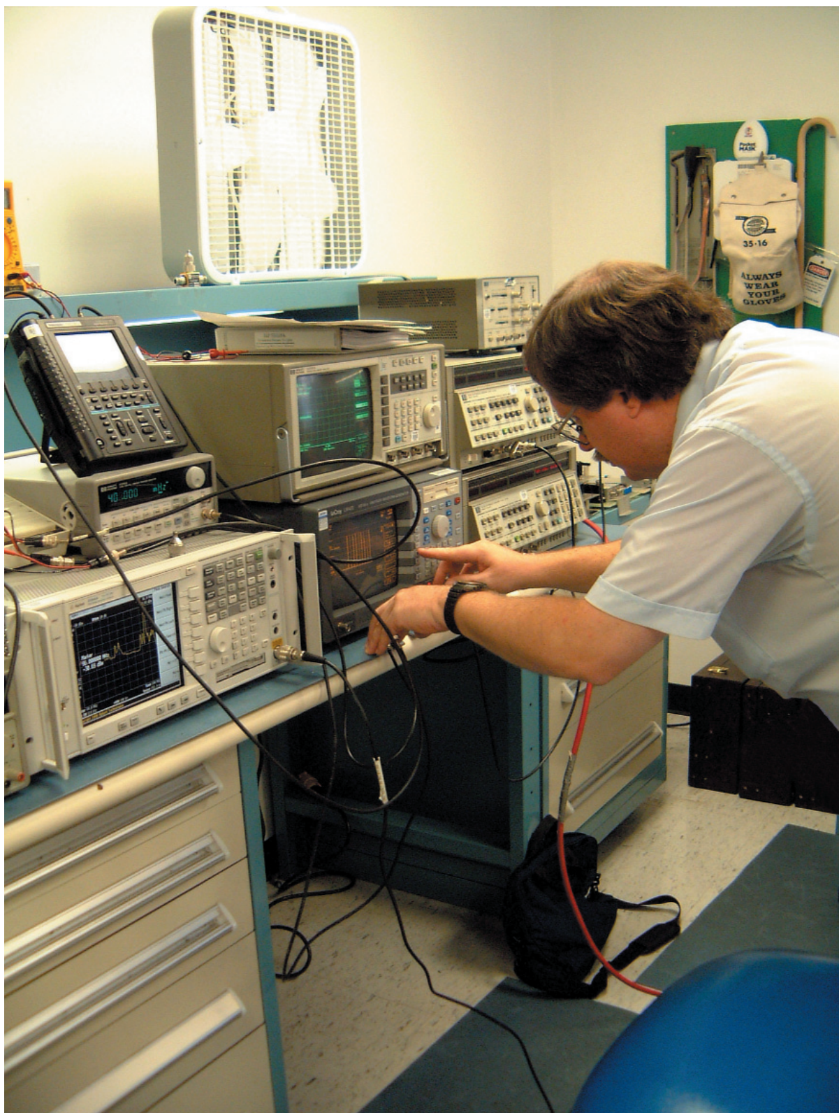
ITS engineer operating suitcase system designed to inject interference into maritime radar receivers at Curtis Bay Coast Guard Station, Maryland (photograph by F.H. Sanders).
