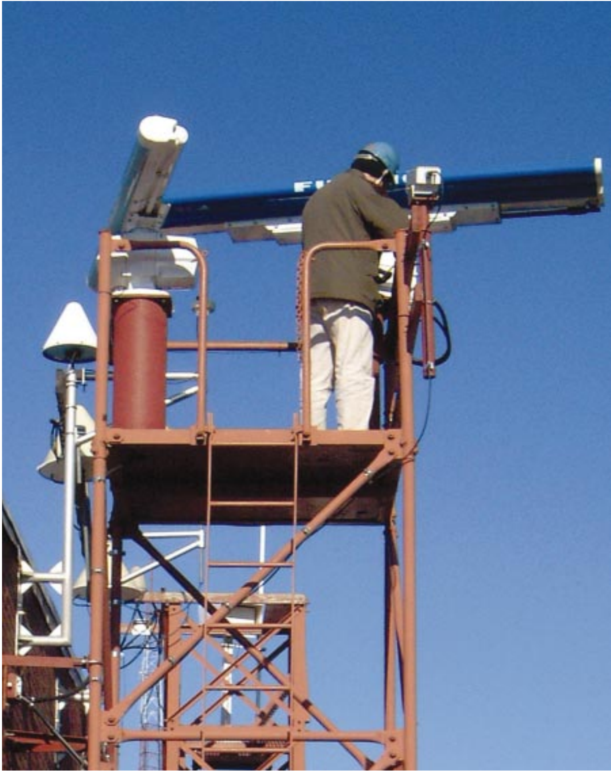
An NTIA engineer prepares a radar for interference injection during ITS-OSM measurements at Curtis Bay, MD (photograph by F.H. Sanders).
