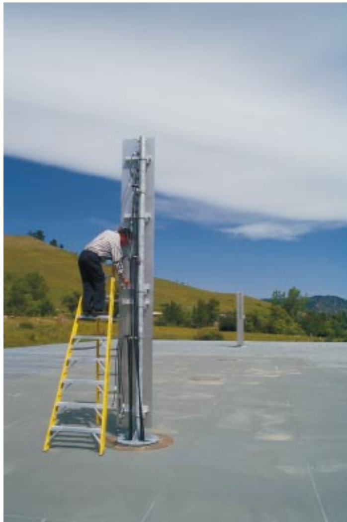
Figure 1. 16-element transmit and receive arrays used for MIMO testing at the NIST open area test site (photograph by P. Papazian).
