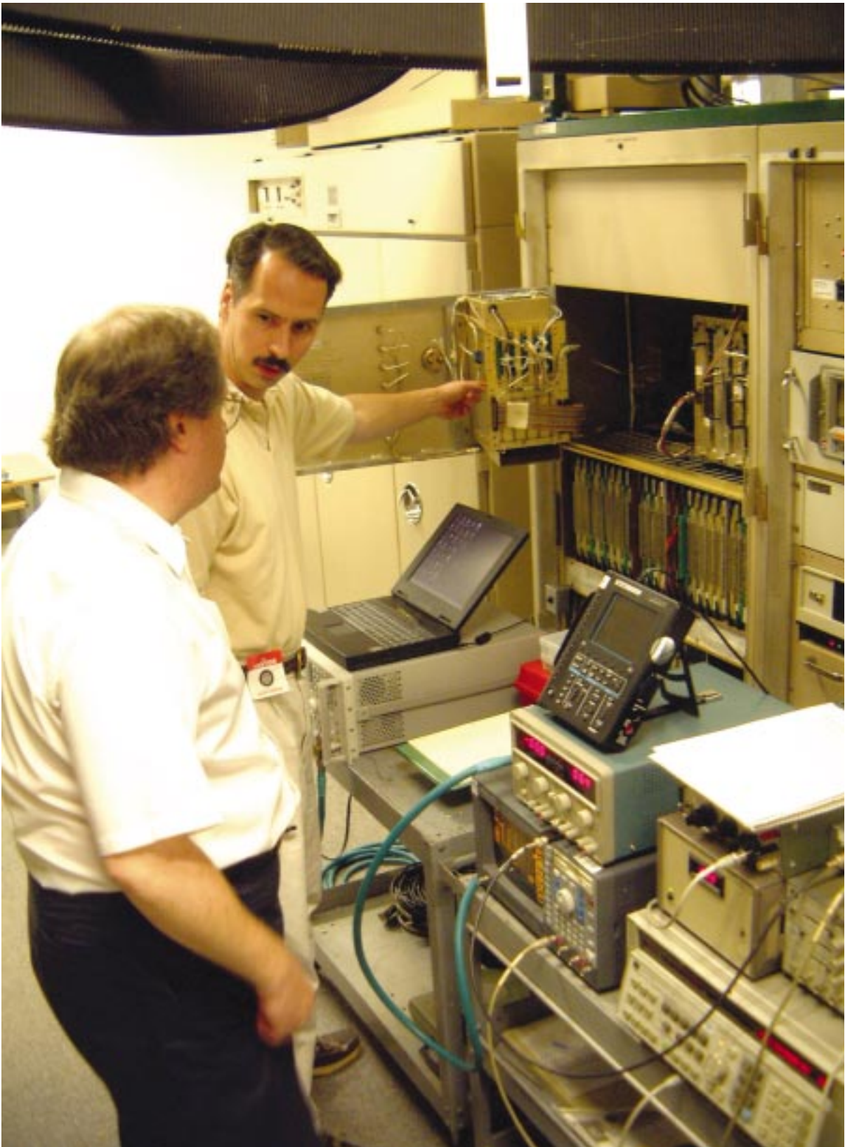
NTIA engineers from ITS and OSM set up equipment for injection of interference signals into an air traffic control radar (photograph by F.H. Sanders).
