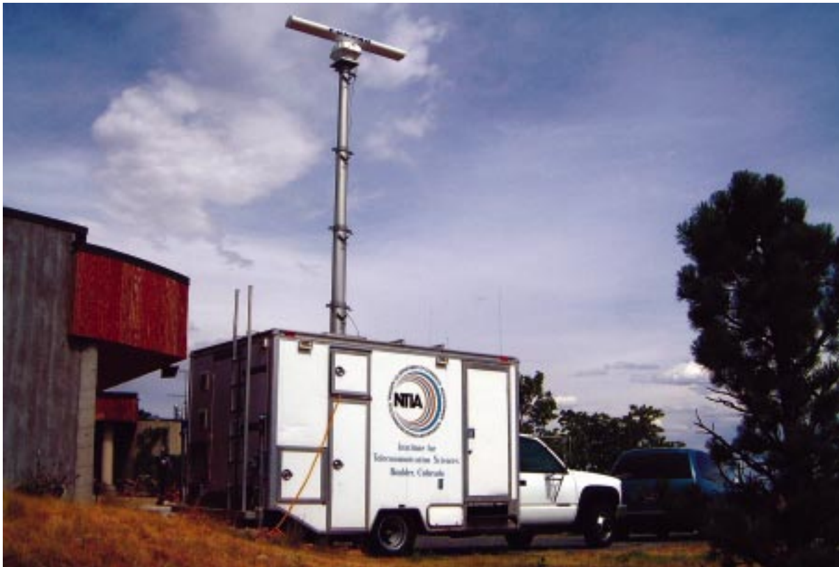
The RSMS transmits radar signals during demonstration of U.S. spectrum measurement techniques for the ITU-R Radar Correspondence Group in Boulder (photograph by F.H. Sanders).
