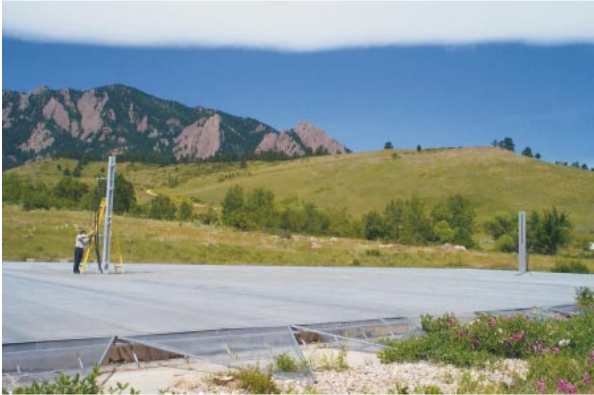
Testing the BLAST antenna system above a ground plane (photograph by P.B. Papazian).
