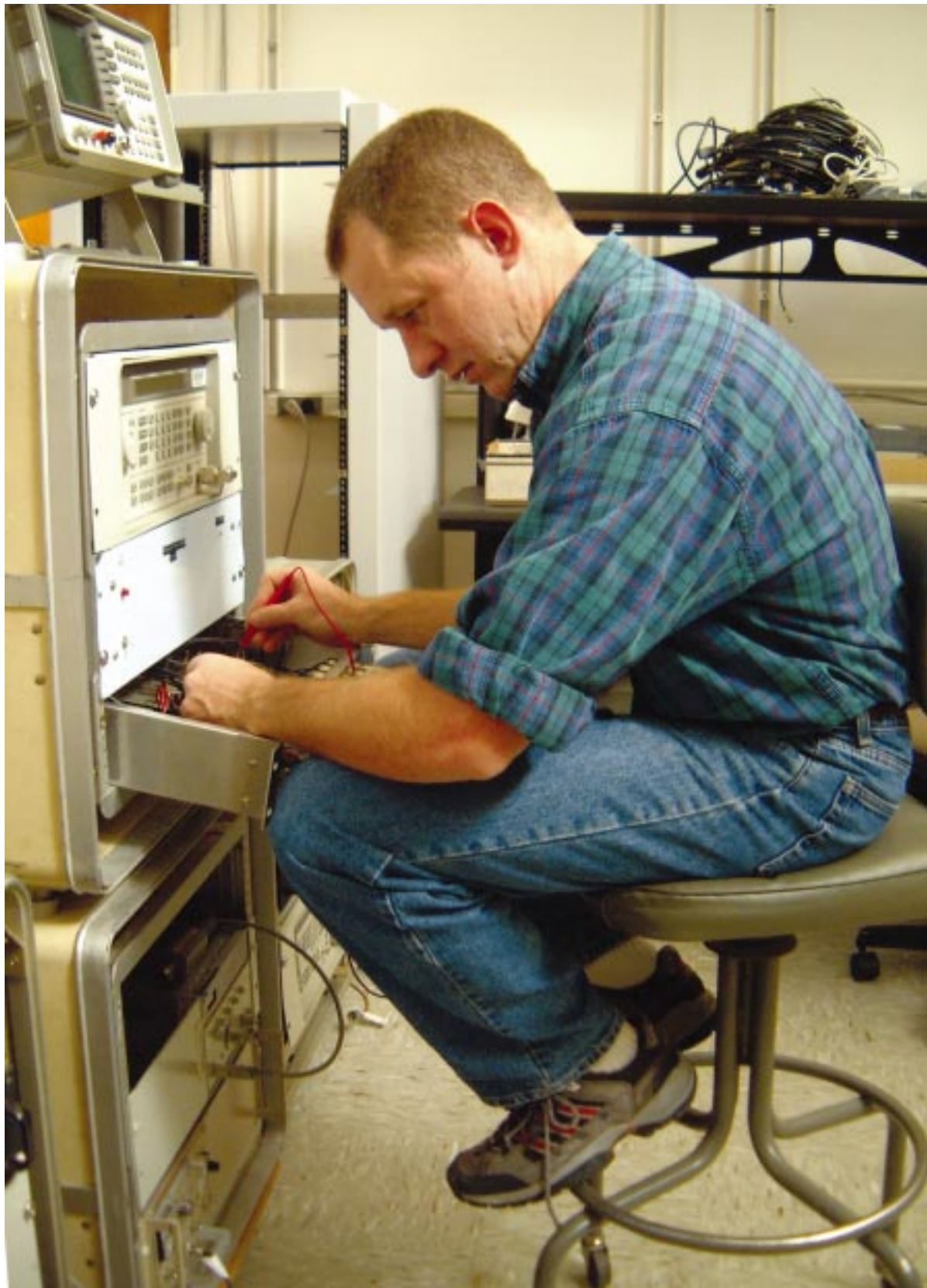
ITS engineer checking for correct voltages on the ITS digital sampling channel probe. (photograph by F.H. Sanders).
