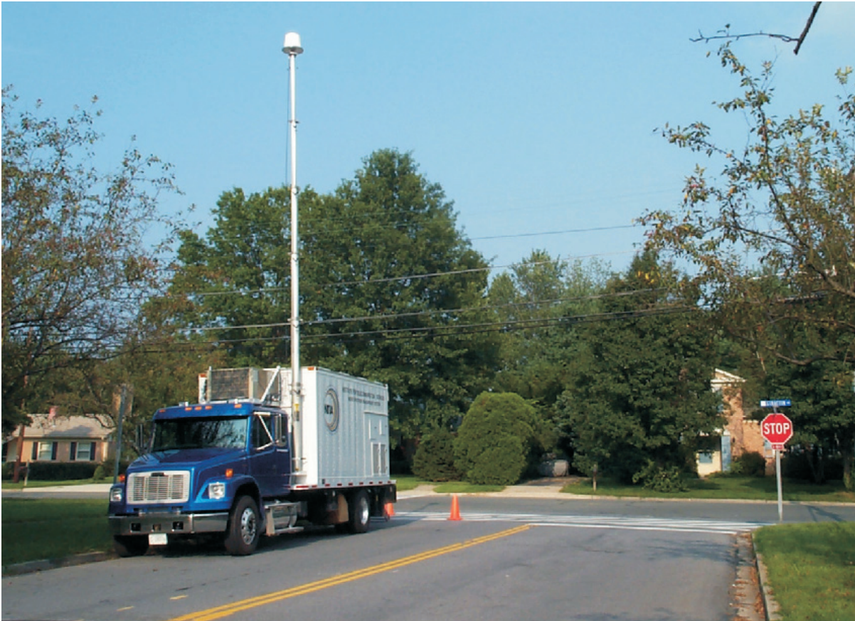
RSMS-4 performing measurements of broadband over power line in a residential neighborhood in September 2003 (photograph by B. Bedford).
