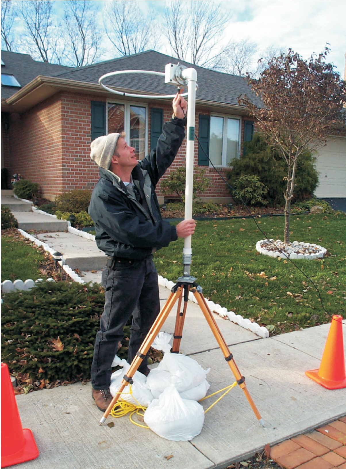
An ITS technician preparing an antenna for the RSMS broadband over power line measurement task in a residential neighborhood (photograph by B. Bedford).
