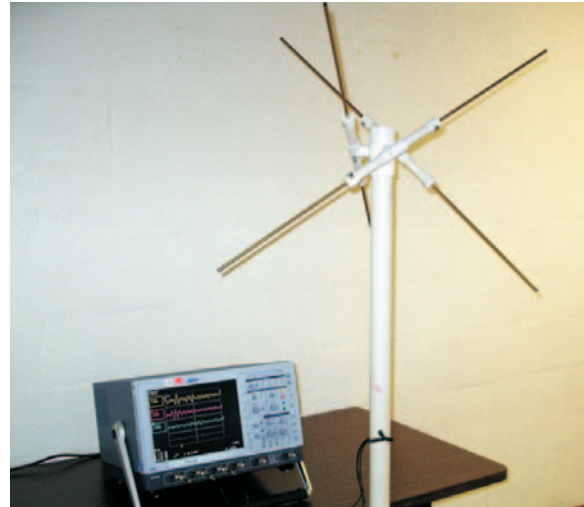
Figure 2. Prototype 3-axis antenna (photo by F.H. Sanders).
