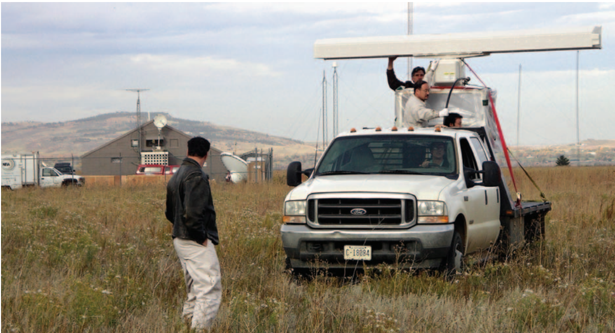
Figure 1. Set-up for a joint US-Japan maritime radar emission spectrum measurement at the ITS Table Mountain facility near Boulder. The measurements were performed using new ITU Recommendation techniques primarily authored by an ITS engineer (photo by F.H. Sanders).
