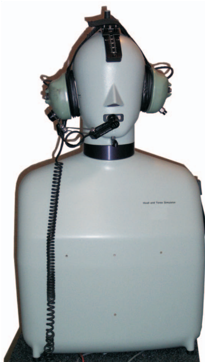
Head and torso simulator with public safety headset and microphone installed (photograph by D.J. Atkinson).
