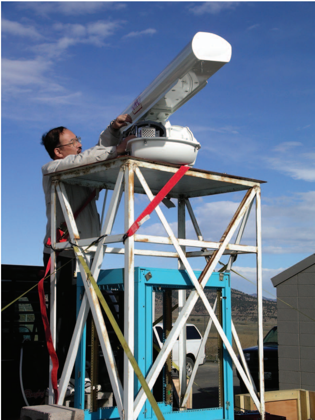
Engineer from the Japanese Administration preparing to perform joint US-Japan maritime radar emission spectrum measurements at the Table Mountain field site (photograph by F.H. Sanders).
