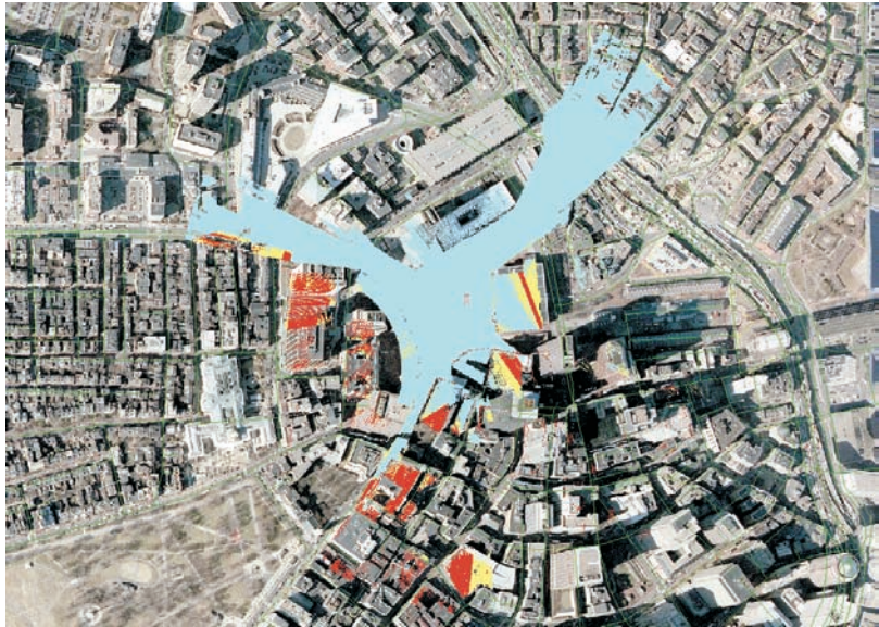
Figure 3. Signal to interference analysis with red indicating significant interference.
