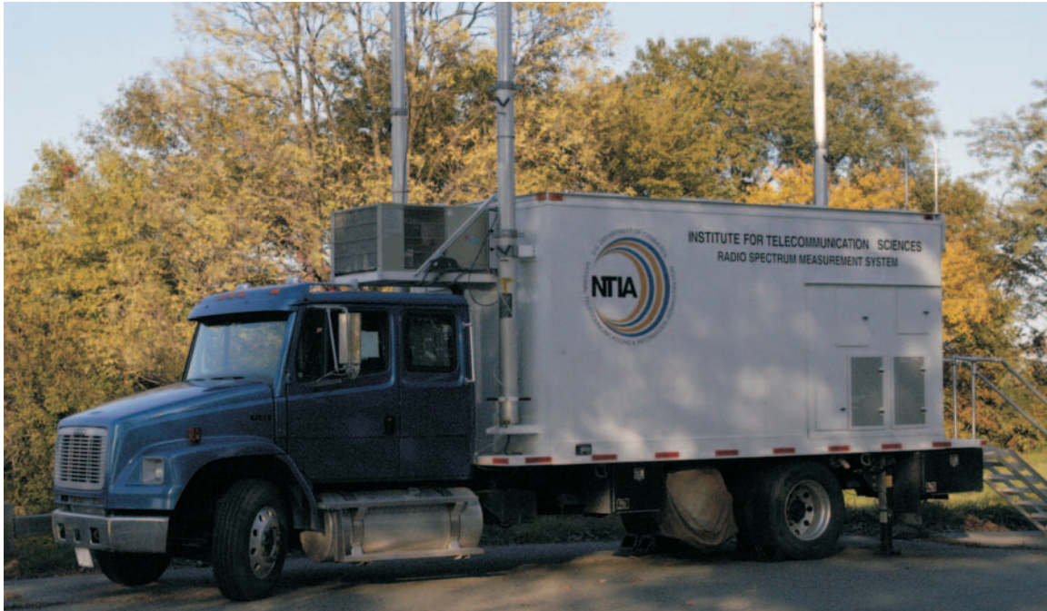
Radio Spectrum Measurement System (RSMS) 4th generation vehicle performing Land Mobile Radio channel occupancy measurements in the Washington DC area. (photograph by B.L. Bedford).
