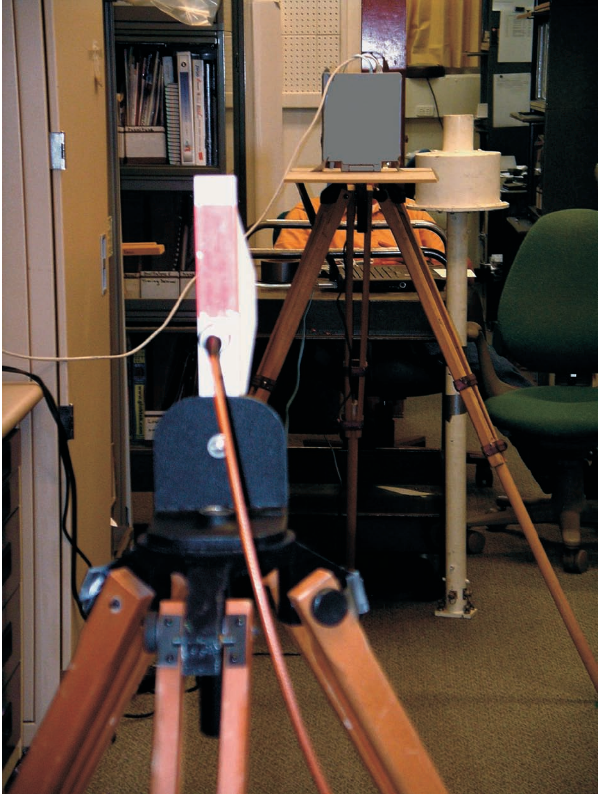
A transmitter antenna (foreground) exposes a 5-GHz wireless access system (WAS) device (gray, center) to radar pulses during tests at ITS. An antenna behind the WAS antenna (white, right) monitors and verifies the presence of the radar pulses (photograph by F.H. Sanders).
