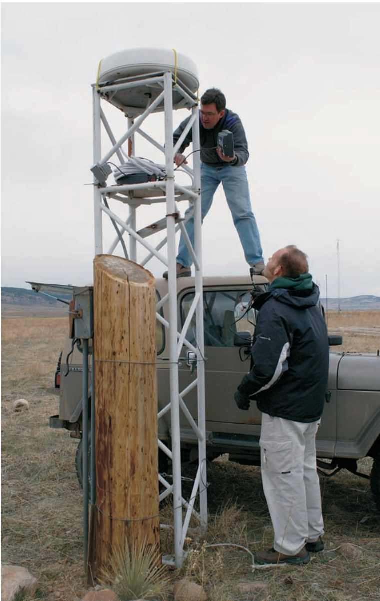
ITS and RF Metrics staff at the Table Mountain field site, preparing to measure the characteristics of the electromagnetic emissions from a newly developed X-band radar (photograph by F.H. Sanders).
