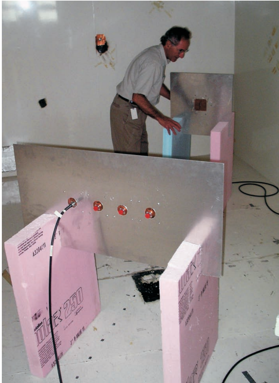
Figure 2. MIMO test setup in NIST reverberation chamber. Antennas configured for single input single output measurement (photograph by F.H. Sanders).
