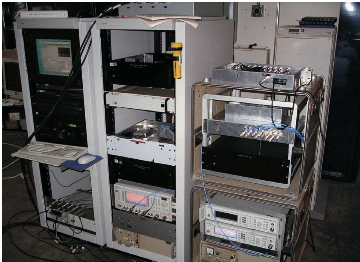
Figure 1. Test equipment configured for 4 channel operation at 2.4 GHz for NIST reverberation chamber characterization (photograph by F.H. Sanders).
