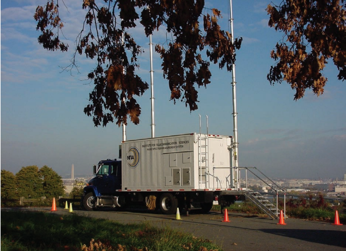
RSMS truck on site for the Land Mobile Radio measurements in Washington D.C. (photograph by I.L. Tobias).
