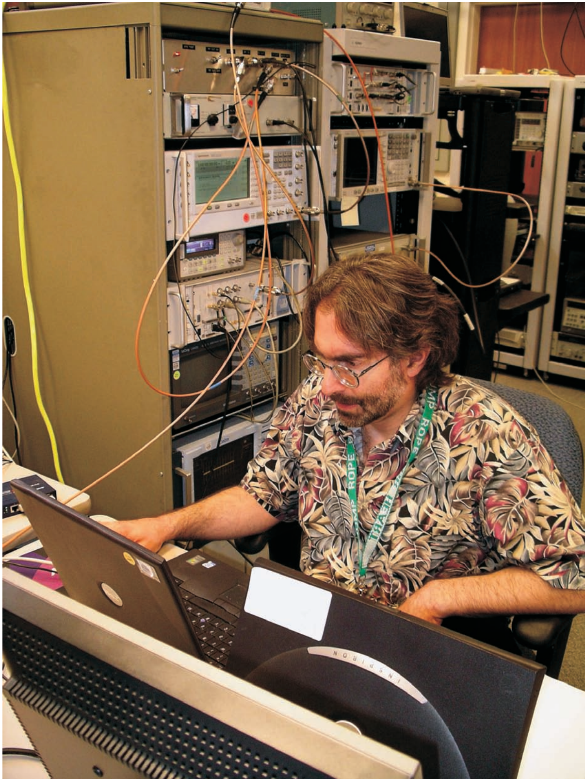
An ITS engineer operates a custom-designed radar transmitter during tests of a prototype 5 GHz dynamic frequency selection (DFS) device at the ITS laboratory (photograph by F.H. Sanders).
