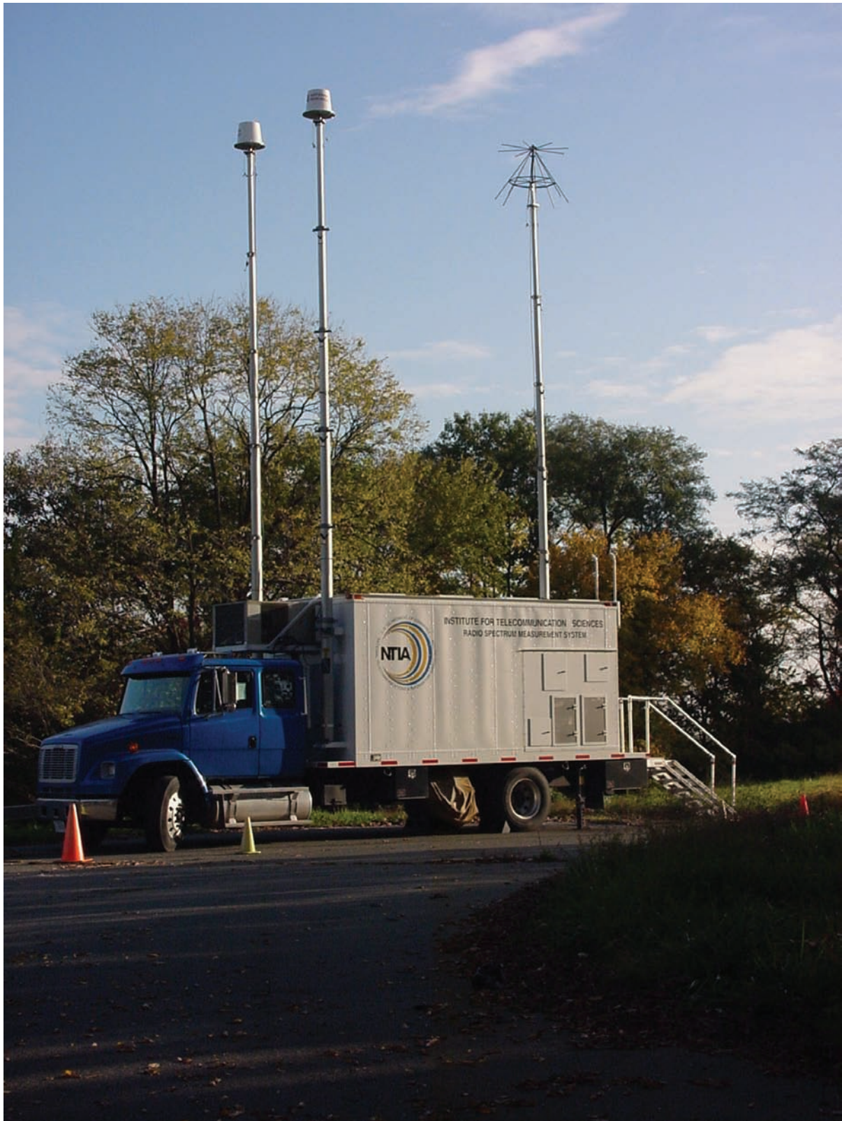
Radio Spectrum Measurement Science (RSMS) truck on site for the Land Mobile Radio measurements in Washington, DC (photograph by I.L. Tobias).
