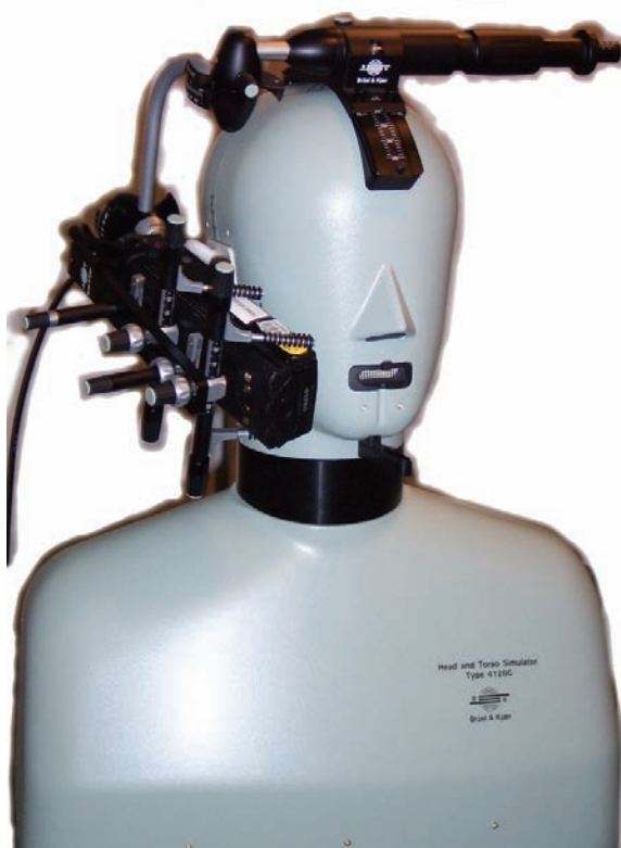
Head and torso simulator configured as a “listener” with a hand-held public safety radio (photograph by D.J. Atkinson).
