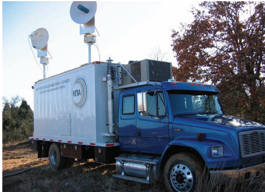
Radio Spectrum Measurement Science (RSMS) vehicle performing measurements in the field (photograph by J.R. Hoffman).
