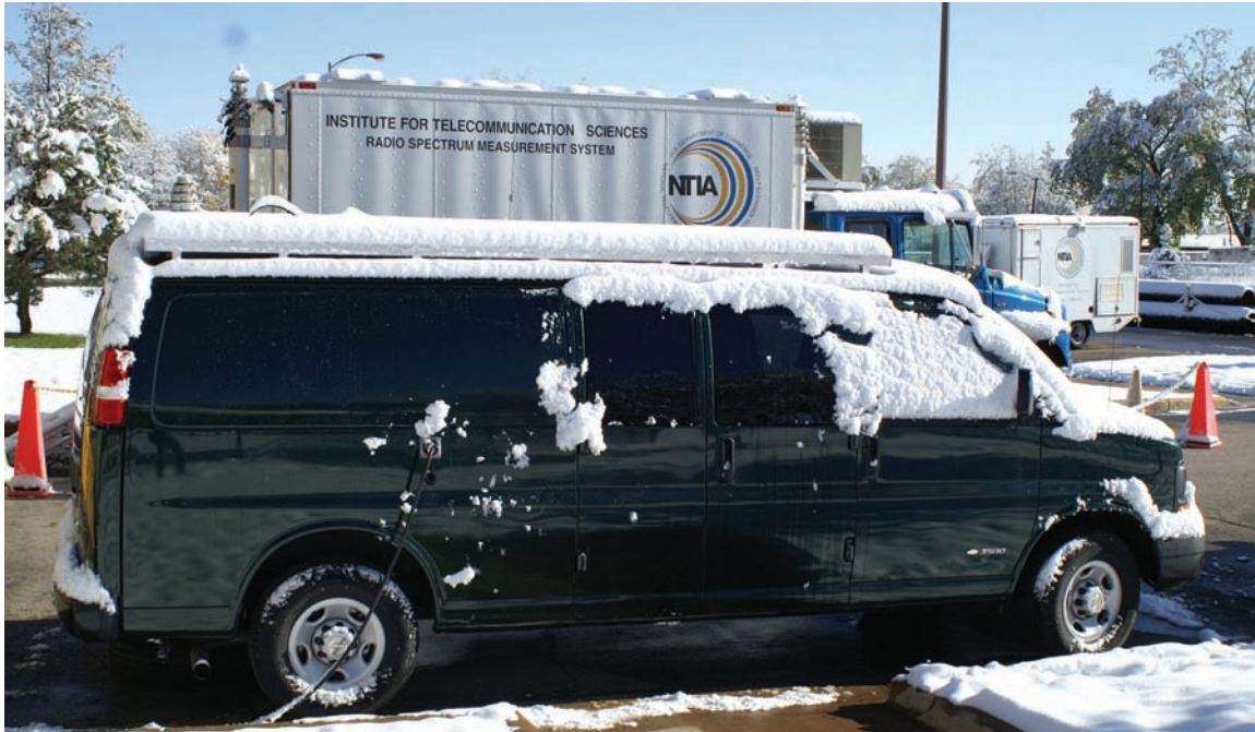
Figure 2. Exterior view of the ITS propagation measurement receiver vehicle (foreground). The rear of the propagation transmitter vehicle is visible at the far right, with an NTIA logo (photograph by F.H. Sanders).
