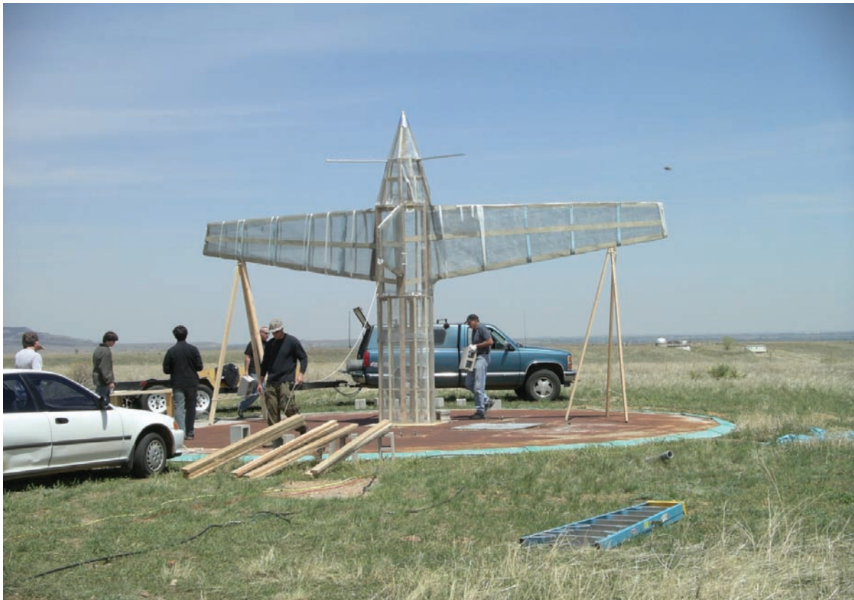
Testing the pattern of antennas mounted on a mock-up of an unmanned aerial vehicle (UAV) at the Table Mountain field site, part of the cooperative research and development agreement (CRADA) between ITS and Johnson's Jobs (photograph courtesy of Russ Johnson, Johnson's Jobs).
