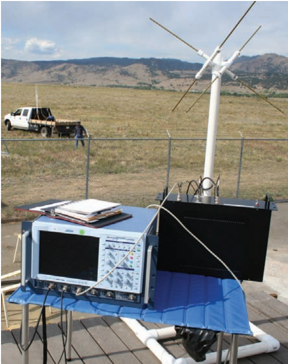
Set-up for testing of 3-axis antenna at Table Mountain field site (photograph by R.N. Statz).
