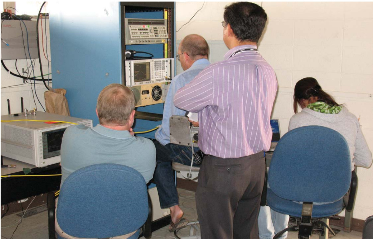
Figure 2. AWS measurement participants examining the spectrum of a prototype wireless device (photograph by J. Carroll).
