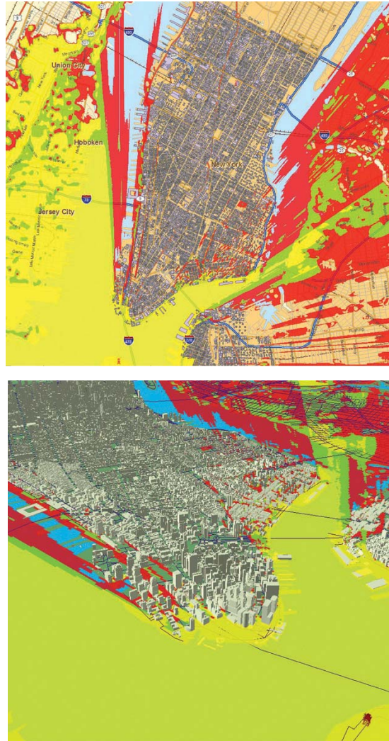
Figure 1. A CSPT-VHF study for New York showing both 2D (top) and 3D (bottom) results.
