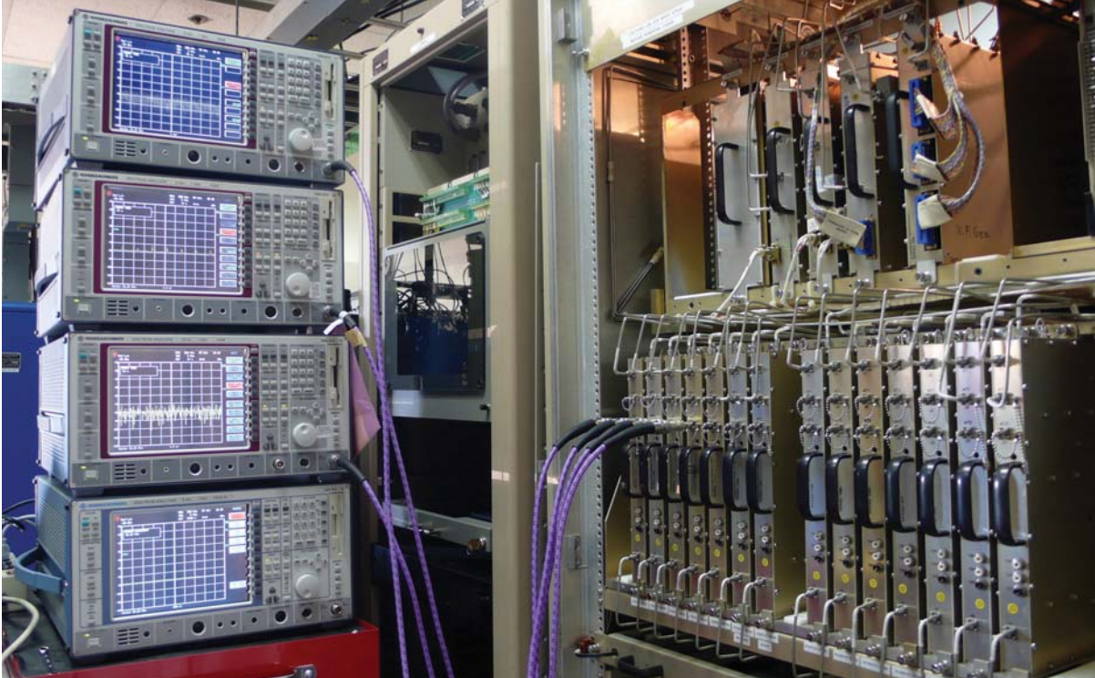
Examining the electromagnetic compatibility of a radar and a Radionavigation Satellite Services (RNSS) signal (photograph by F.H. Sanders).
