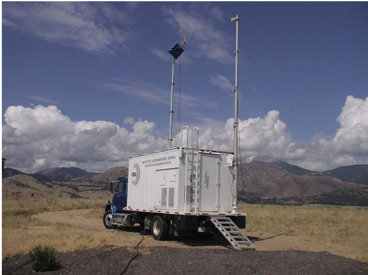
Figure 1. Physical setup used for antenna polarization mismatch loss measurements (photo by B. Bedford).
