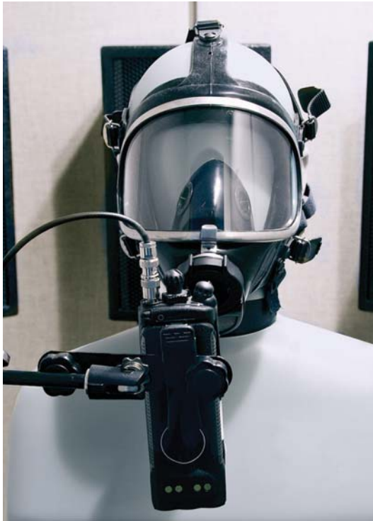
At ITS' Public Safety audio labs, an ITU-Standard Head and Torso Simulator "speaks" through a fireman's self-contained breathing apparatus (SCBA) mask into a radio.
