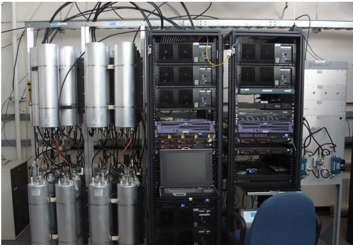
A P25 radio base station at the ITS laboratory (photograph by F.H. Sanders).
