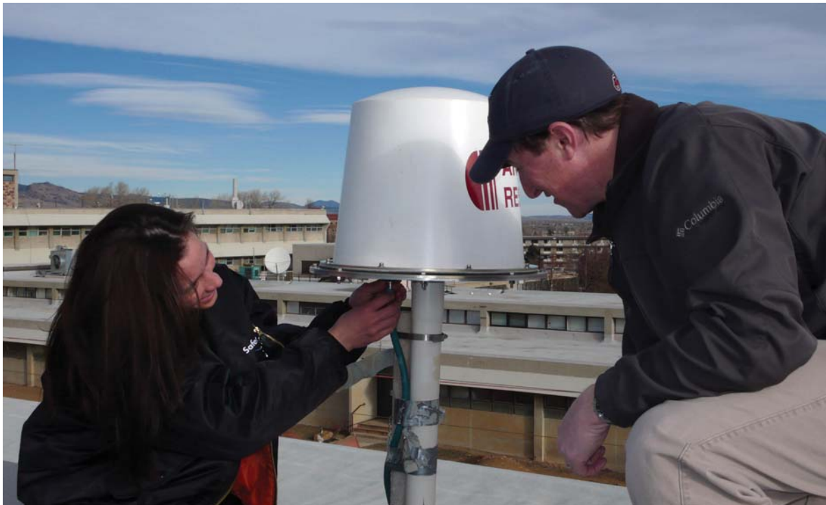
Two ITS engineers prepare an antenna on the laboratory rooftop prior to a set of spectrum occupancy measurements (photograph by F.H. Sanders).
