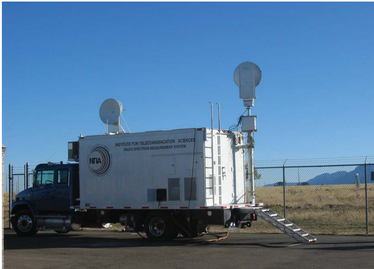
The ITS Radio Spectrum Measurement Science (RSMS) vehicle set up to perform measurements at the Table Mountain Field Site (photograph by J.W. Allen).
