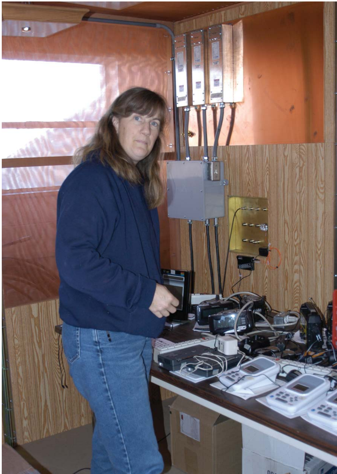
An ITS engineer performing tests of NOAA Weather Radios at the Table Mountain Field Site (photograph by J.W. Allen).
