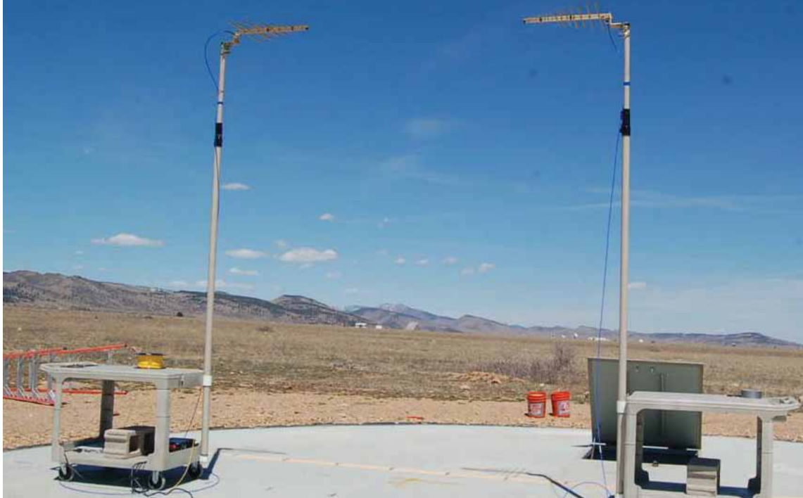
Figure 2. Field uniformity transmission measurement with two log-periodic antennas 3.5 m above the Table Mountain turntable (photograph by R.T. Johnk).
