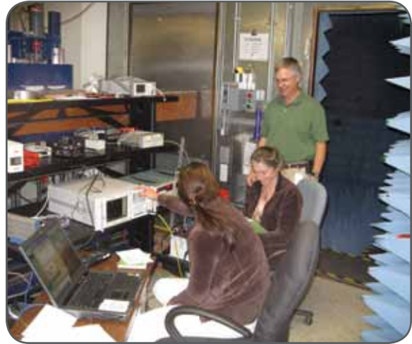
ITS staff members performing system verification tests in preparation for radiated emissions measurements of Land Mobile Radios (photograph by J.R. Hoffman).
