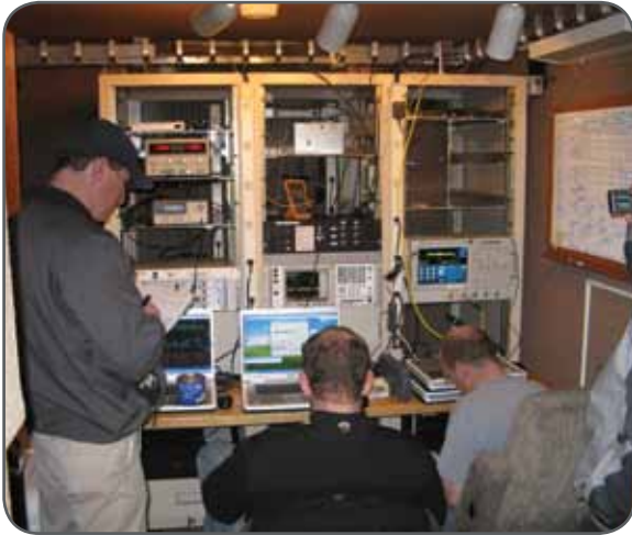
ITS staff members performing Radar Spectrum Engineering Criteria (RSEC) compliance measurements within the RSMS 4 mobile RF shielded enclosure (photograph by J.R. Hoffman).
