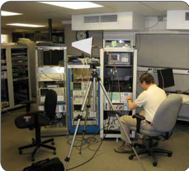
An ITS staff member setting up the ITS Dynamic Frequency Selection test system in preparation for product surveillance testing for the Spectrum and Propagation Measurements Division (photograph by J. Carroll).
