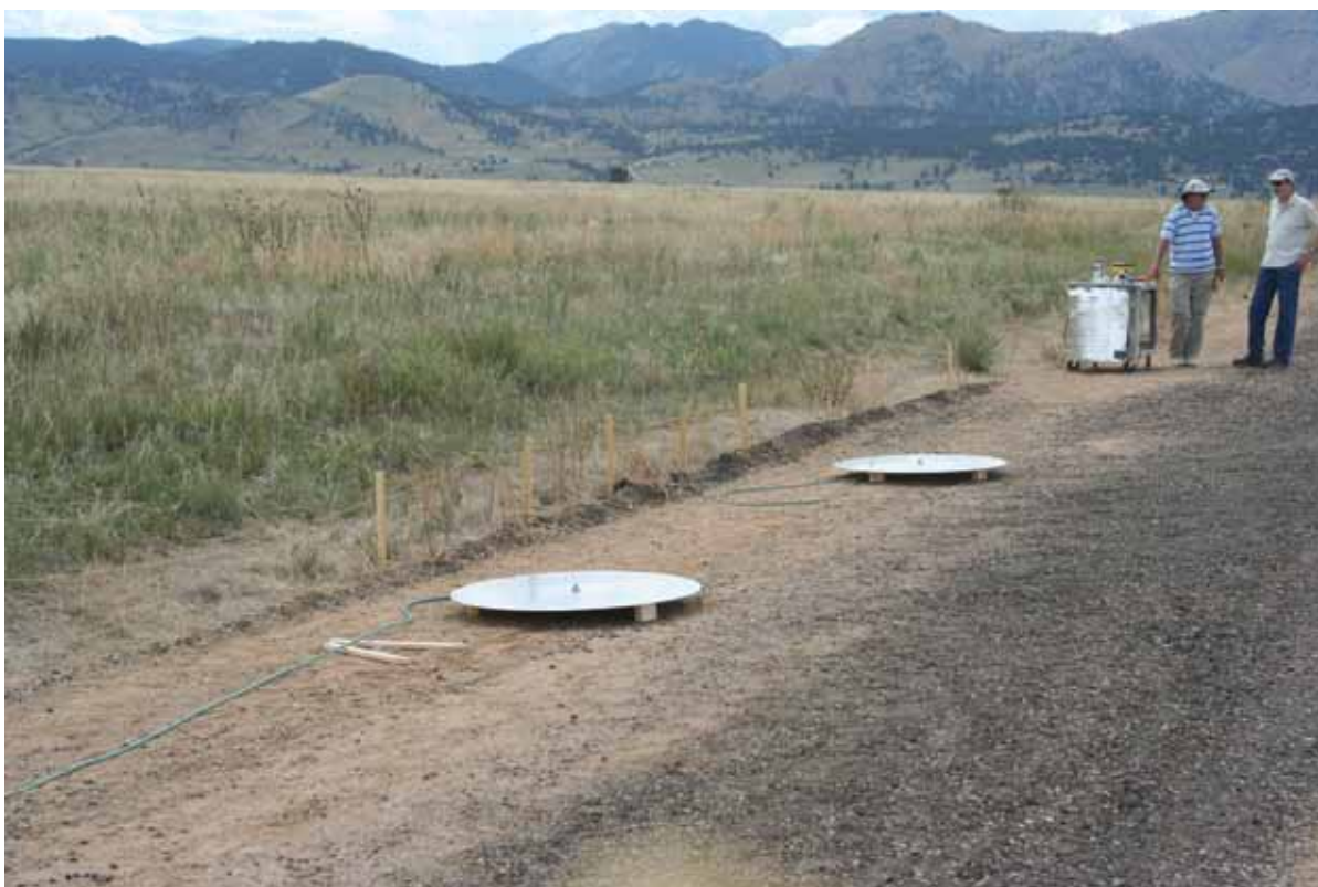
The two monopole-on-a-ground plane antennas are positioned at a height of zero meters for a close-in distance and ultra-low antenna height measurement (photograph by S. Carroll).
