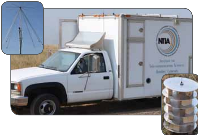
In FY 2009, Telecommunications Engineering, Analysis, and Modeling Division engineers conducted a series of field measurements in order to develop new propagation models with specific applications like very low antenna heights and short distances. The field measurement campaign was extensive, including several types of environments and unique path characteristics (photographs by S. Carroll).
