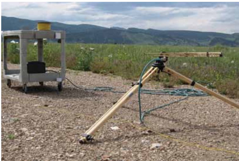
Figure 1. Log-periodic receiving antenna used to perform field uniformity measurements of the Table Mountain turntable (photograph by R.T. Johnk).
