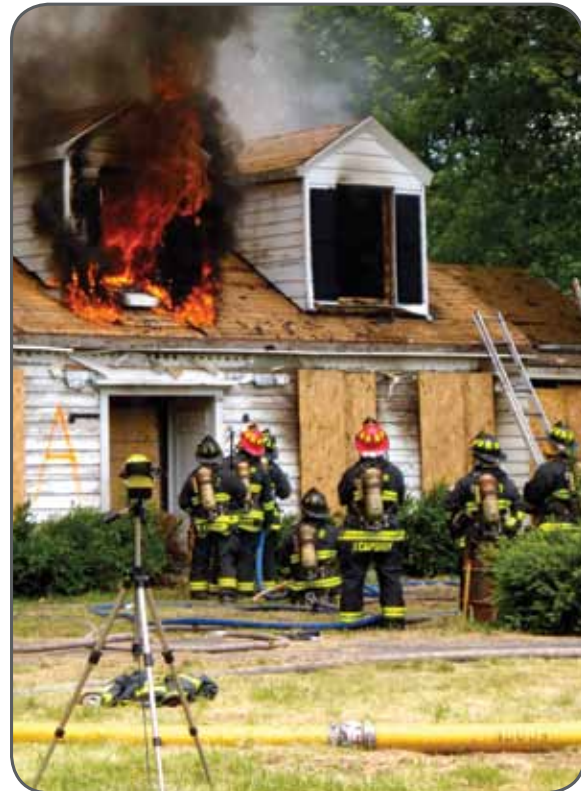
An ITS video camera records an exercise burn. Incident controllers can use video to analyze a fire based on smoke color and density, as well as flame intensity (photograph by D.J. Atkinson).
