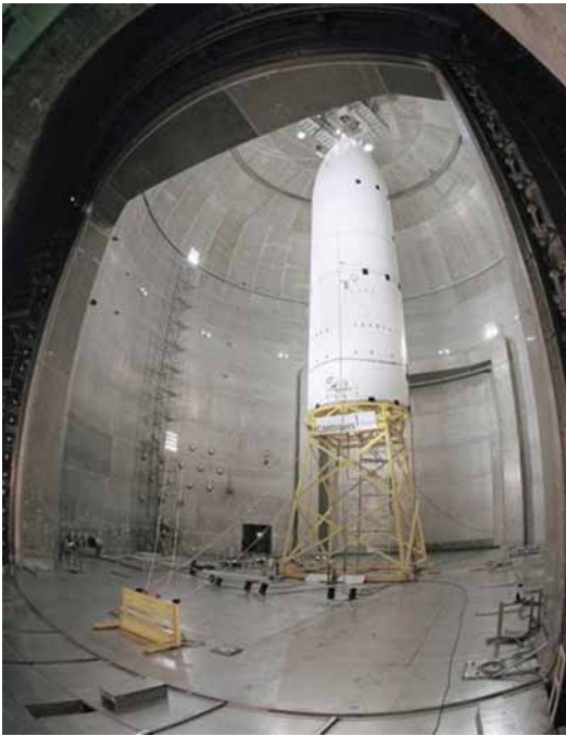
Figure 1. The SPF vacuum chamber with typical test article. Note the large access door and buttresses in front of and behind the rocket.
