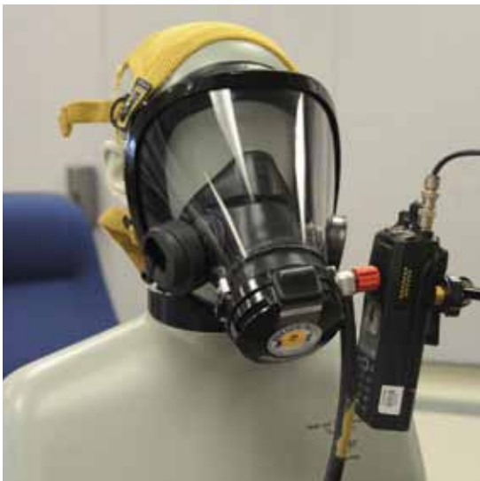
A head and torso simulator (HATS) simulating voice distortion through SCBA field equipment.
