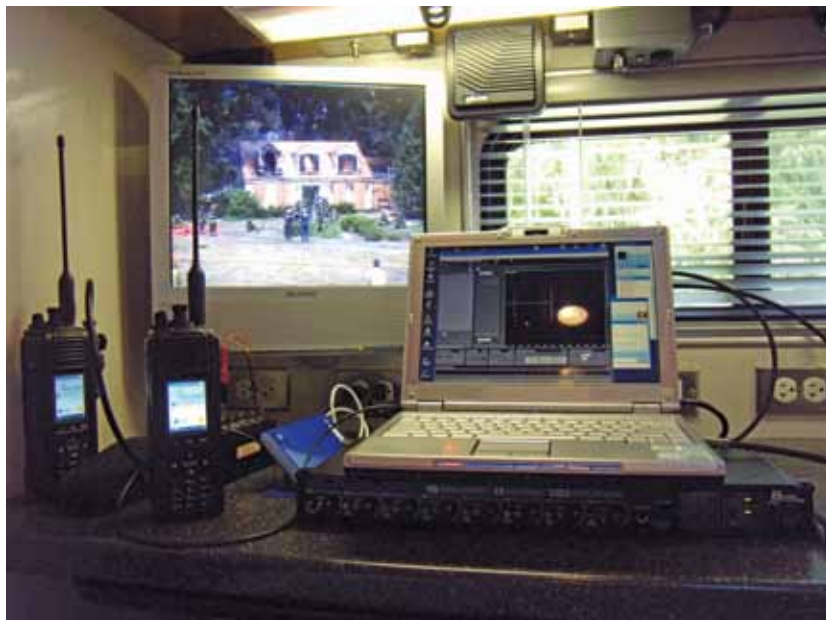
Figure 1. Field equipment recording audio from radio channels as well as microphones embedded in a burning house (photograph by D.J. Atkinson).
