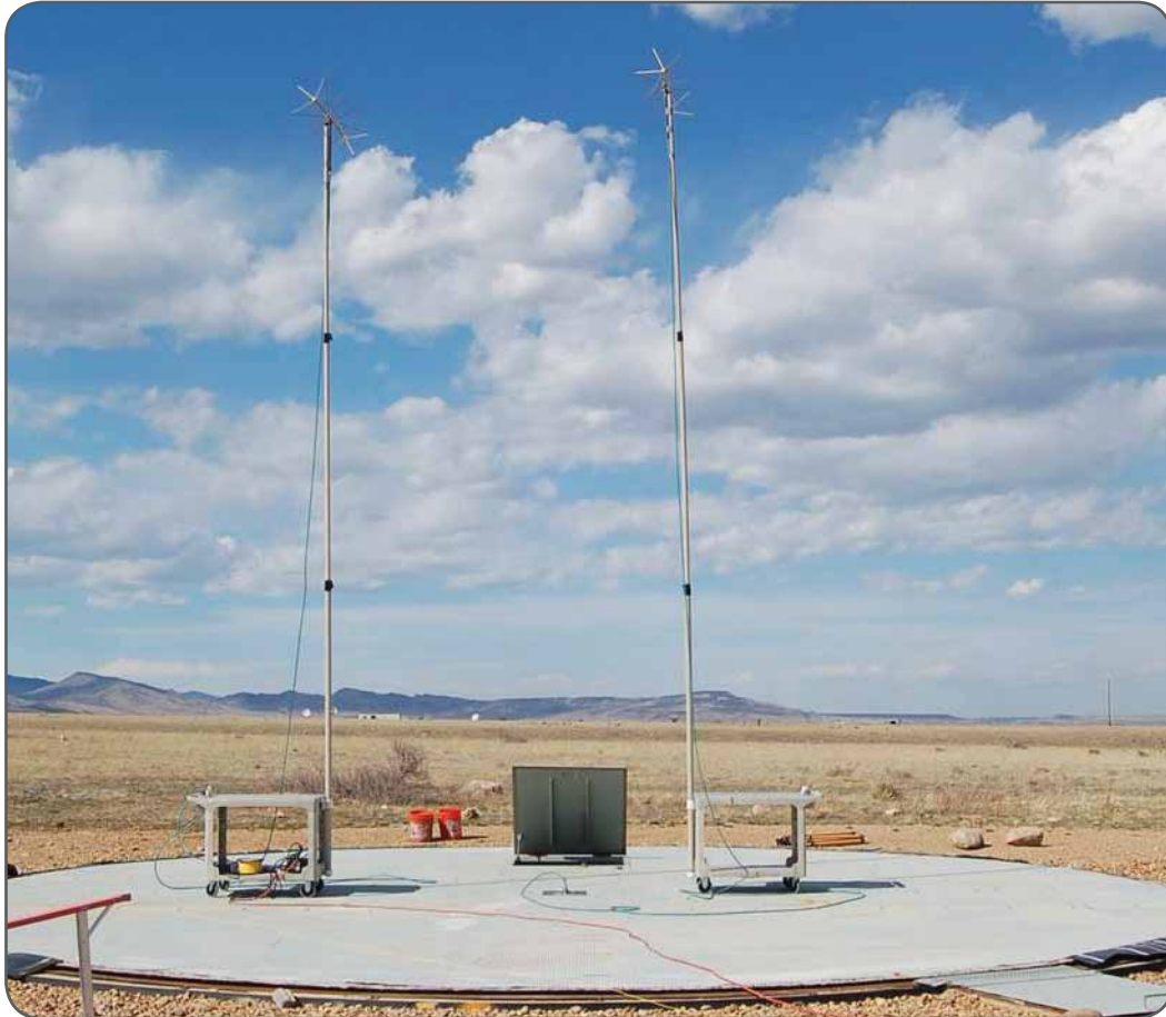
ITS maintains the Table Mountain Field Site's buildings and resources, like this turntable, for telecommunications research (photograph by J.W. Allen).
