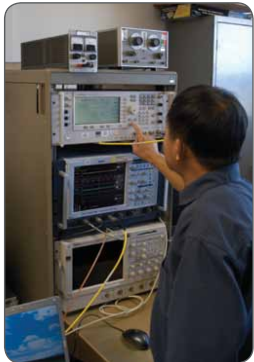
An ITS staff member adjusting instrument settings while evaluating the detection sensitivity of a Dynamic Spectrum Access device (photograph by I. Tobias).
