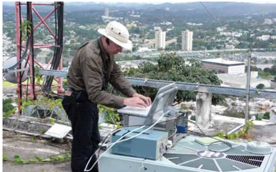
Figure 2. An ITS engineer performing rooftop measurements to study the electromagnetic compatibility between a weather radar and nearby wireless devices (photograph by J.E. Carroll).
