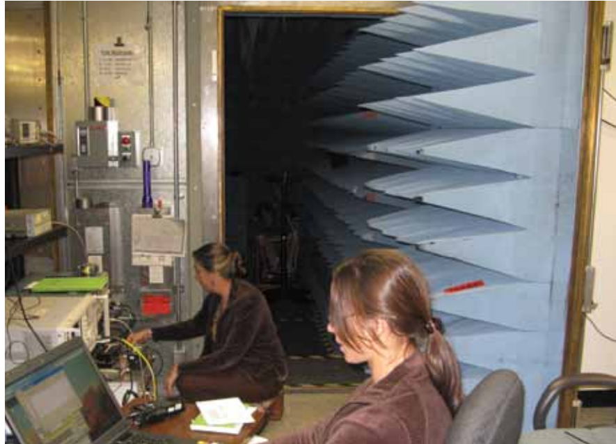
Figure 1. ITS engineers performing harmonic measurements on Land Mobile Radio systems in an anechoic chamber (photograph by J.R. Hoffman).
