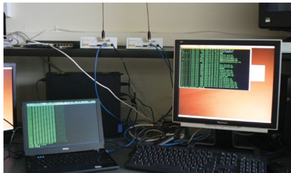
Bit error statistic measurement system. The transmitter and receiver are software-defined radios enclosed in the white boxes with the attached whip antennas. The laptop computer displays received bits and the desktop display shows the directory of codes written for this application (photograph by M.A. McFarland).
