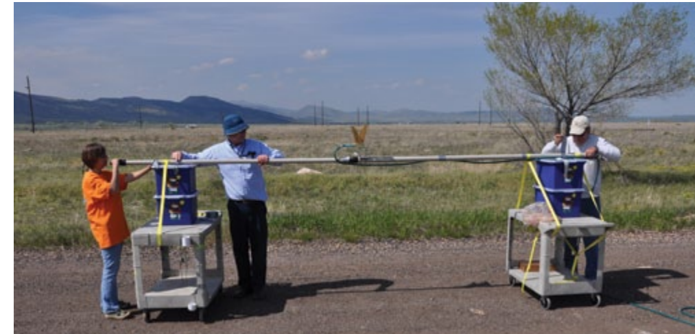
Figure 2. Calibrating the experimental ground constant measurement system (photograph by R.T. Johnk).
