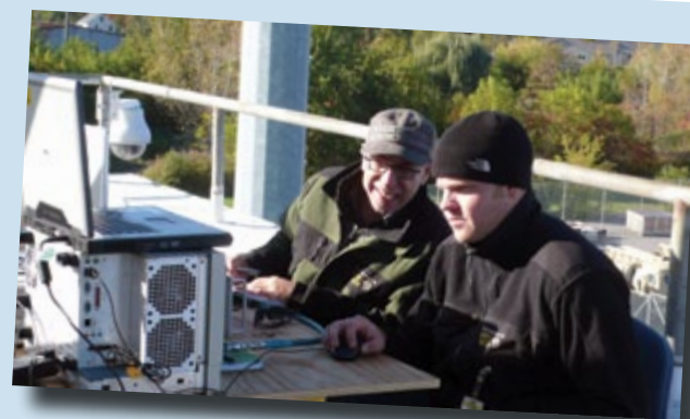
Two ITS engineers measuring radar emissions from an air search radar (TPS-79) on a rooftop during a CRADA project to verify compliance with the Radar Spectrum Engineering Criteria (RSEC) (photograph courtesy of Lockheed Martin).
