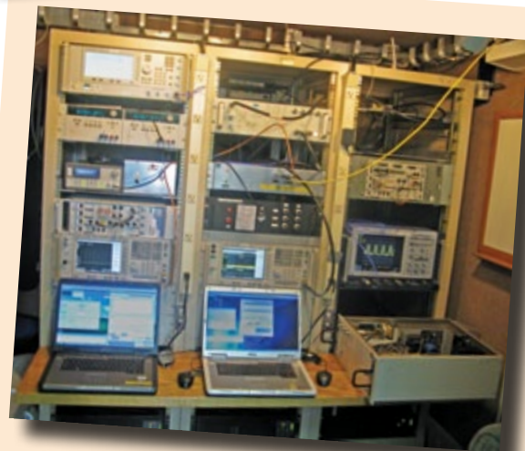
An automated spectrum measurement is in progress inside the RSMS truck (photograph by J.R. Hoffman).
