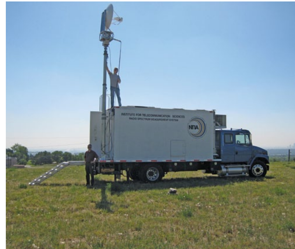
Figure 2. The RSMS 4G truck deployed to a nearby high site for a spectrum survey. An ITS staff member is preparing a dish antenna on a rotatable mount (photograph by H. Ottke).
