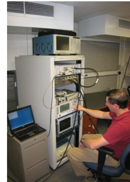
Figure 2. An ITS engineer verifying simulated TDWR radar signals (photograph by J.E. Carroll).
