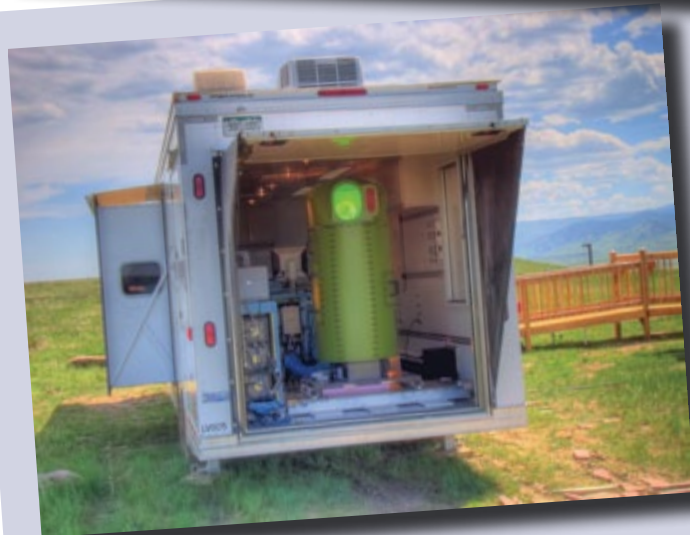
The PROWL system is able to detect chemical and biological hazards using LIDAR techniques. Here, the Lockheed Martin system is shown being tested against benign targets at the Table Mountain Field Site (photograph courtesy of Lockheed Martin Coherent Technologies).
