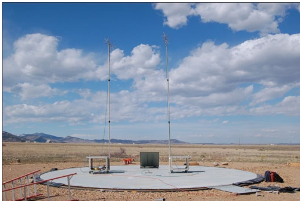
Figure 1. Free-Space reference obtained with biconical antennas at the Table Mountain Field Site.
