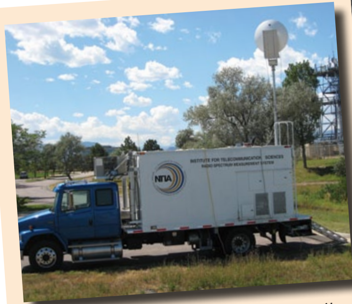
The RSMS vehicle deployed to a field site to measure out of band emissions of a WiMAX base station (photograph by J.E. Carroll).
