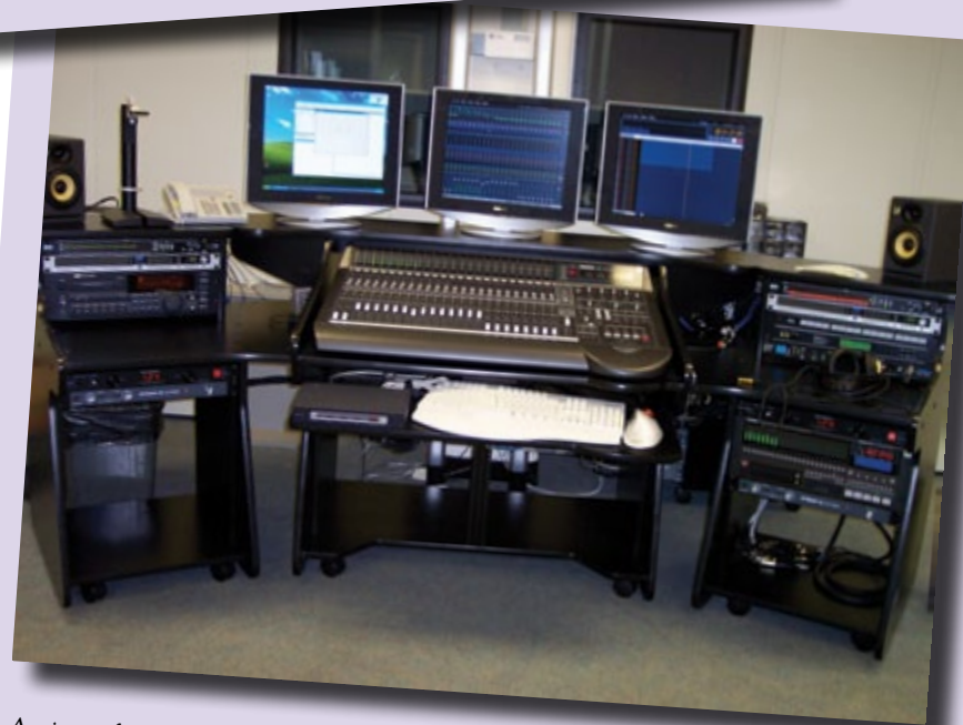
A view of the Public Safety Audio Laboratory (PSAL) showing some of the digital audio mixing, distribution, storage, and filtering equipment used in the investigation of the voice and video quality of public safety communication systems in harsh environments (photograph by D.J. Atkinson).
