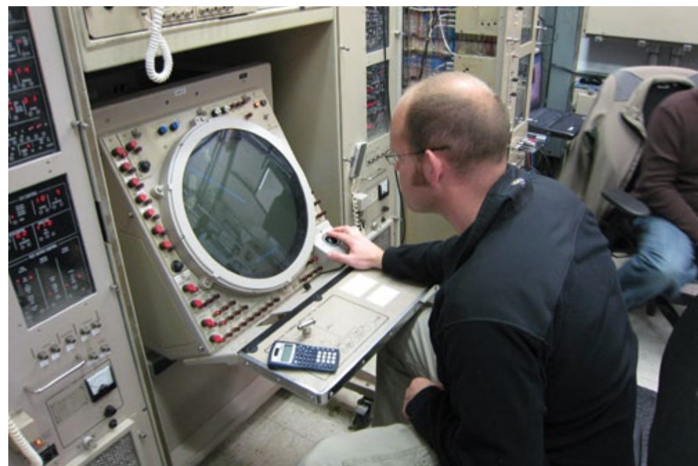
Figure 1. An ITS engineer examining the output of a radar plan position indicator (photograph by G.A. Sanders).
