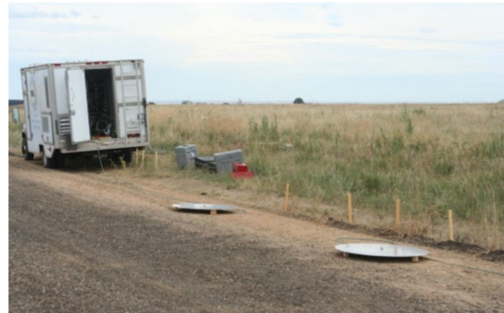
The two monopole-on-a-ground plane antennas are positioned at a height of zero meters for a close-in distance and ultra-low antenna height measurement (photograph by S.Carroll).
