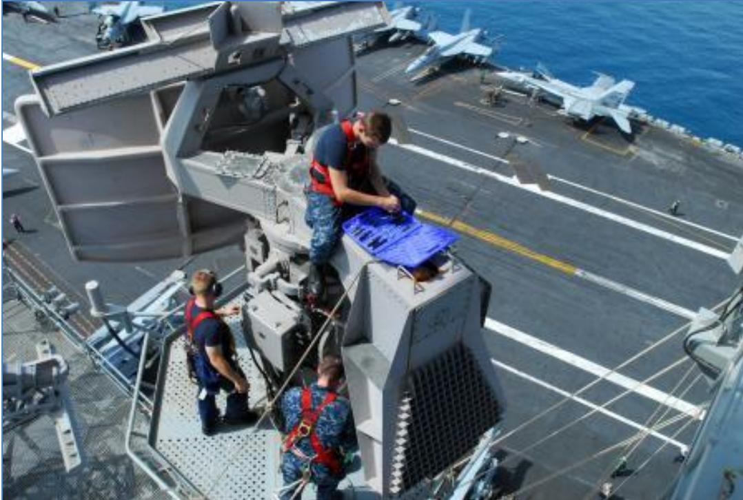
Figure 47. SPN-43C naval ATC (navigation) radar (courtesy: Defense video and imagery).
