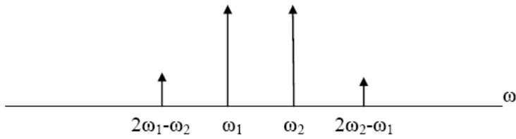
Figure 30. Example of intermodulation products for a two-tone input signal.
