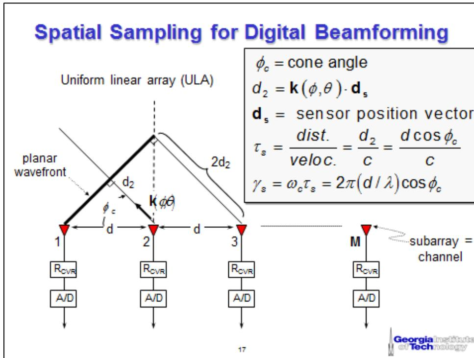
Figure 16. Spatial sampling for digital beamforming.
