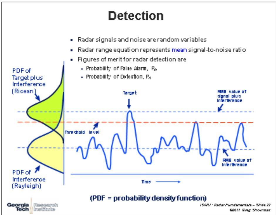
Figure 5. Illustration of radar amplitude detection.
