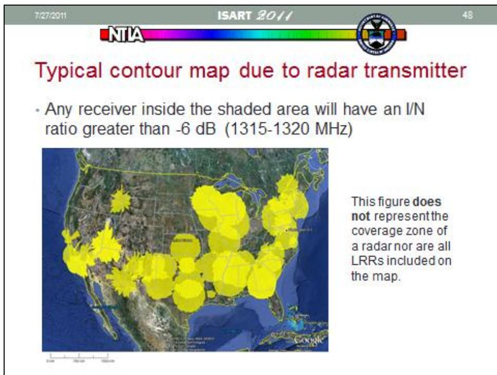
Figure 43. Typical L-band contour map (NTIA/OSM).
