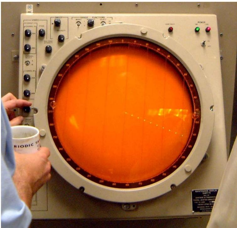
Figure 45. ASR plan position indicator display.
