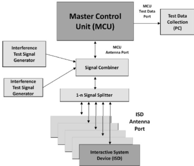
Figure 7. Test Set-Up.
