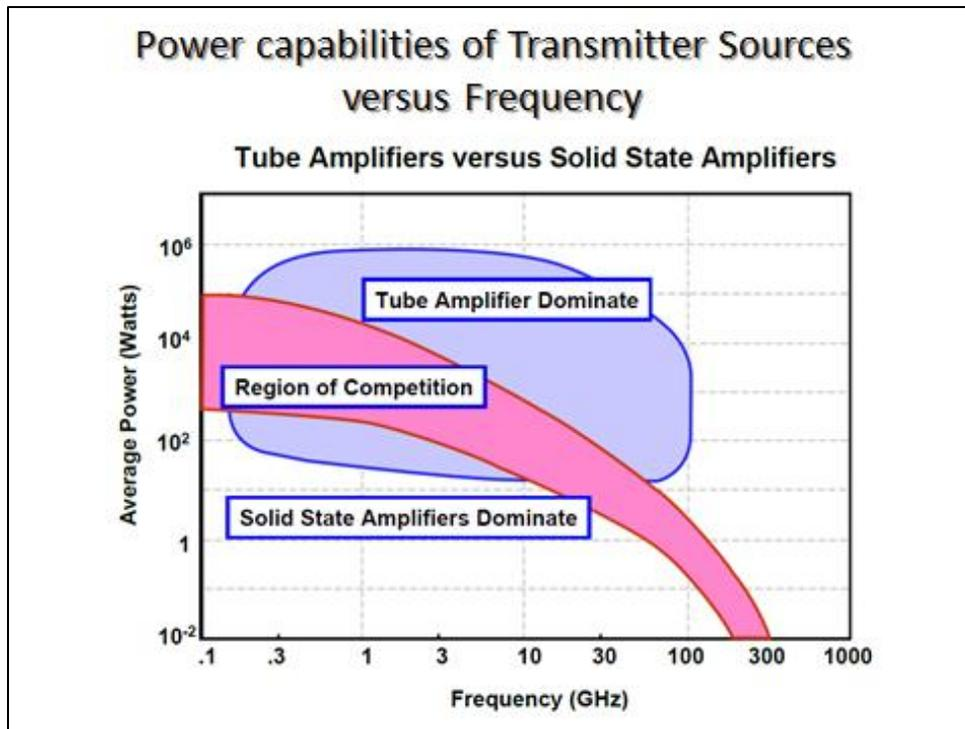
Figure 29. Tube versus solid state amplifier regions in terms of power and frequency.
