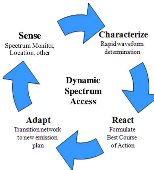
Figure 1. Dynamic Spectrum Access (DSA) Technology
