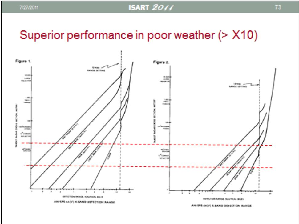
Figure 49. Performance comparison of X- to S-band maritime radar systems operating in different weather conditions.
