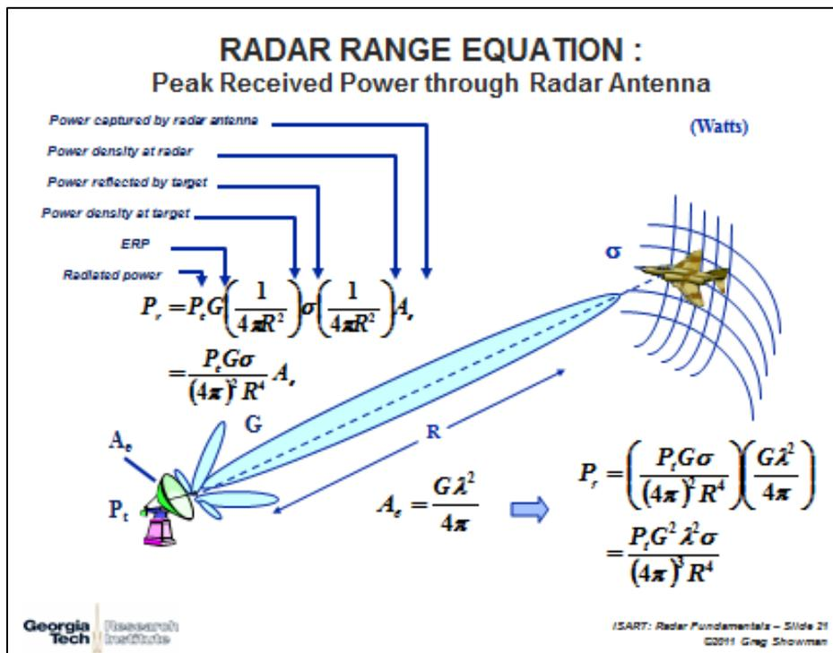
Figure 3. Radar range equation.
