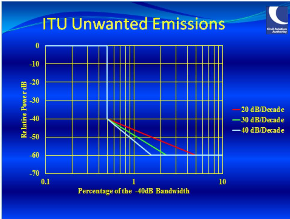
Figure 57. ITU radar emission limits.
