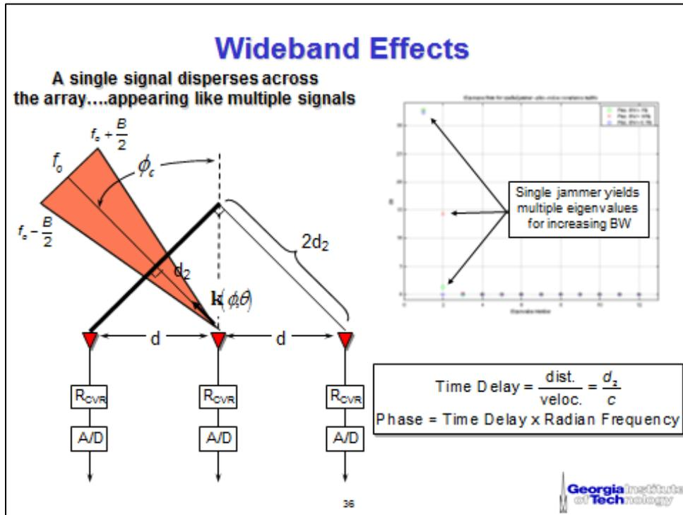
Figure 26. Interference effects on a wideband receive array.
