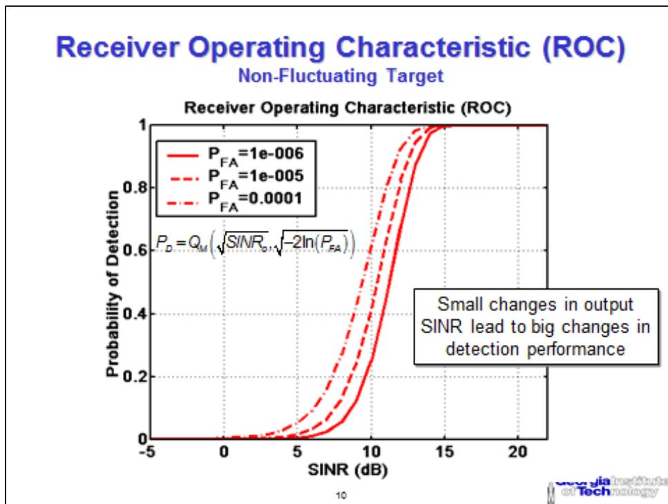
Figure 14.  $P_d$  versus  $SINR$  for a non-fluctuating target.
