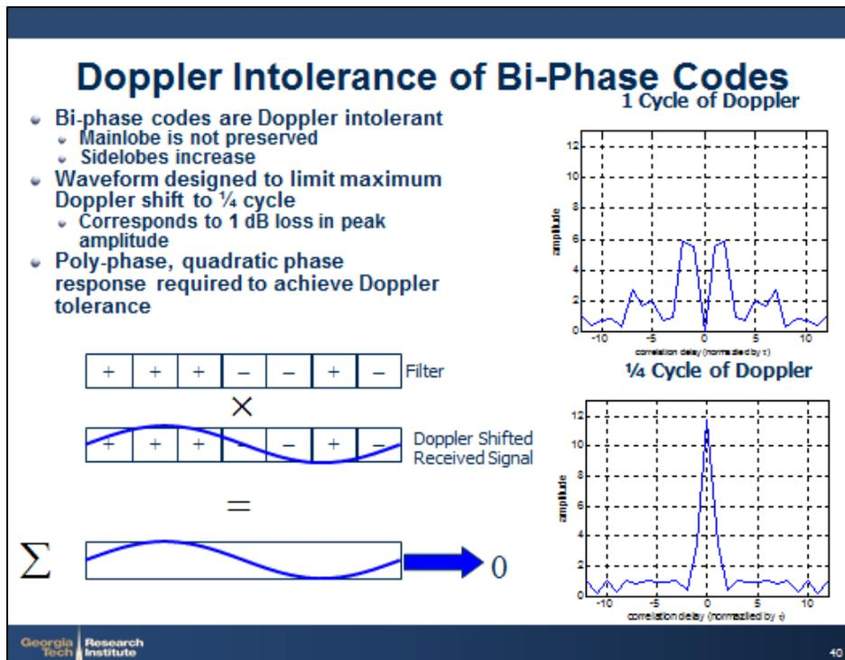
Figure 9. Doppler intolerance of bi-phase codes.
