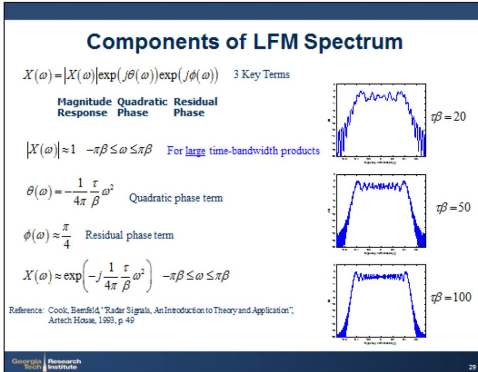
Figure 7. Frequency characteristics of LFM waveforms.
