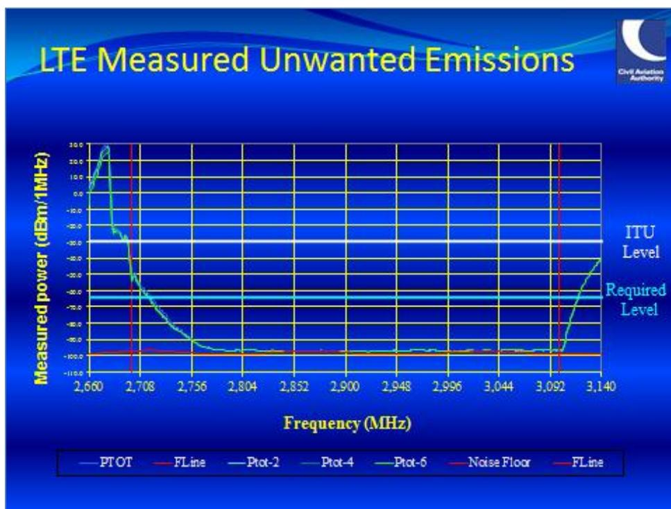
Figure 60. Measured WiMAX/LTE emissions with current ITU and CAA required OOB limits.
