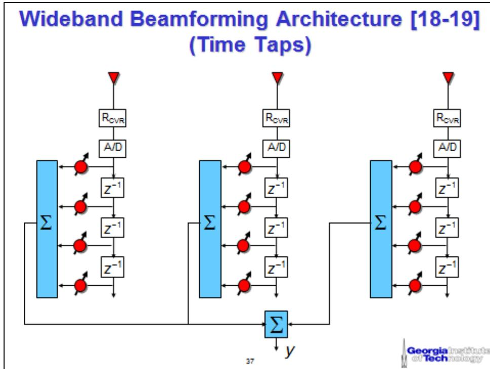
Figure 27. Wideband beamforming architecture used for STAP.
