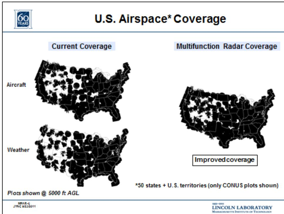
Figure 66. Improved overall coverage if MPAR replaced weather and aircraft surveillance radars.
