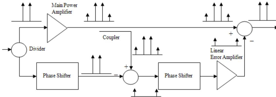
Figure 31. Feedforward approach to subtracting out IMPs.
