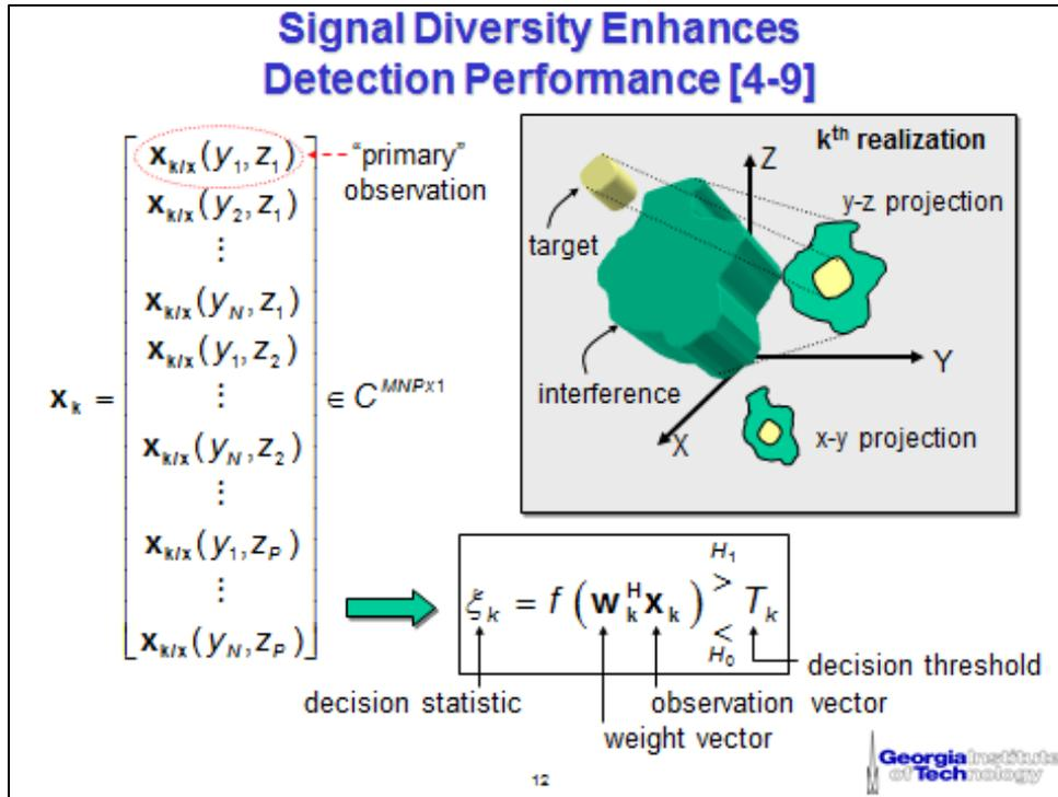
Figure 15. Signal diversity enhancements to detection performance—references in slide refer to [12], [13], [14], [15], [16], and [17].
