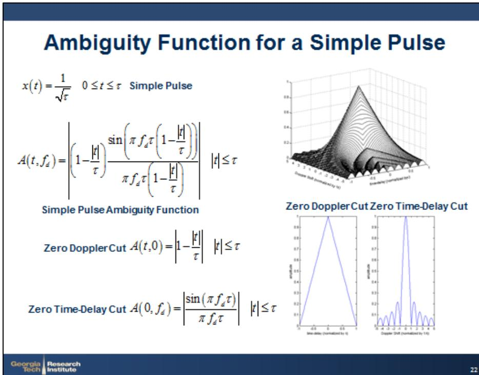
Figure 6. Ambiguity function for a rectangular pulse.
