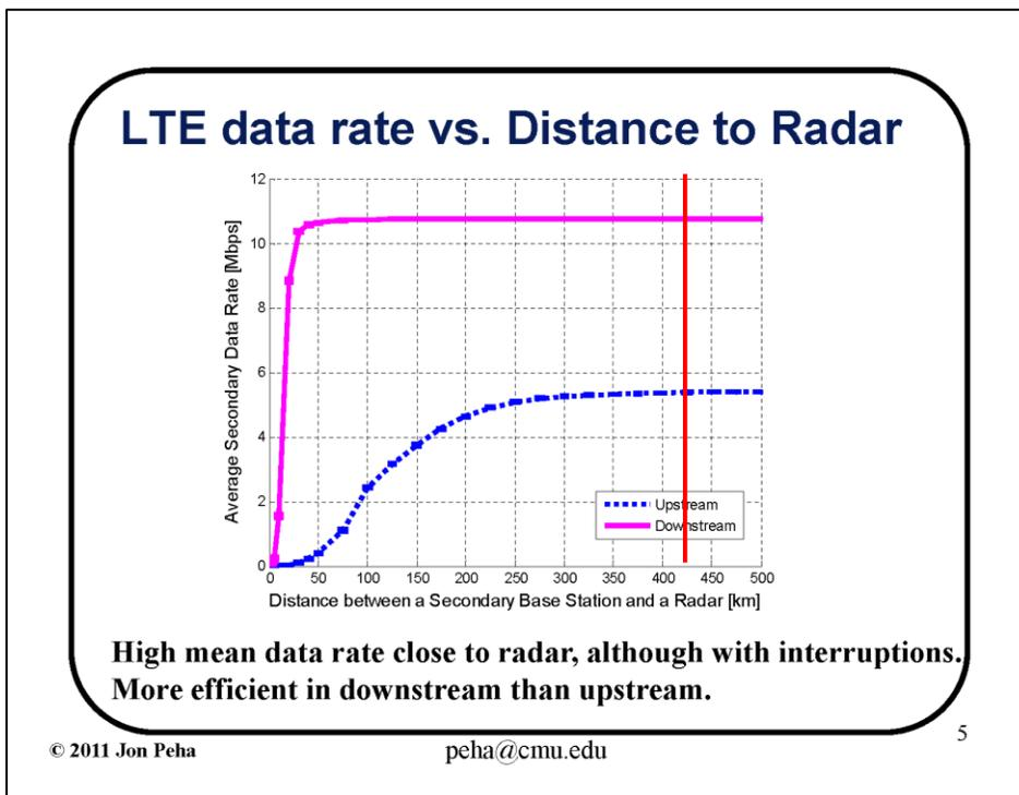
Figure 72. LTE performance versus radar-LTE separation.
