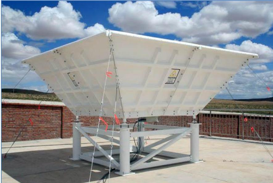
Figure 40. Lower L-band wind profiler radar.
