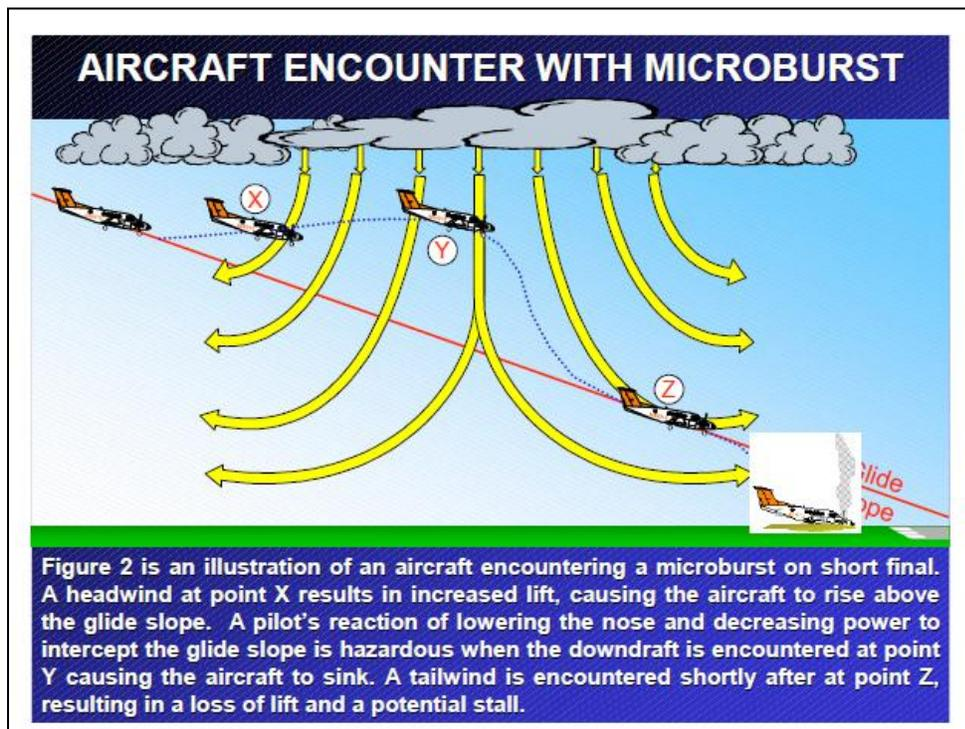
Figure 52. Aircraft microburst encounter.
