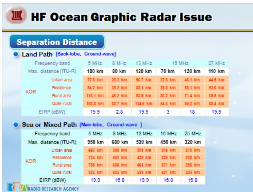
Figure 63. HF OGR separation distances to avoid interference.
