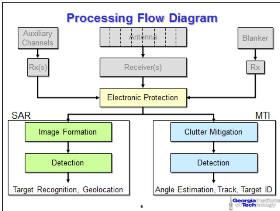
Figure 13. Processing flow diagram for a generalized radar receiver.
