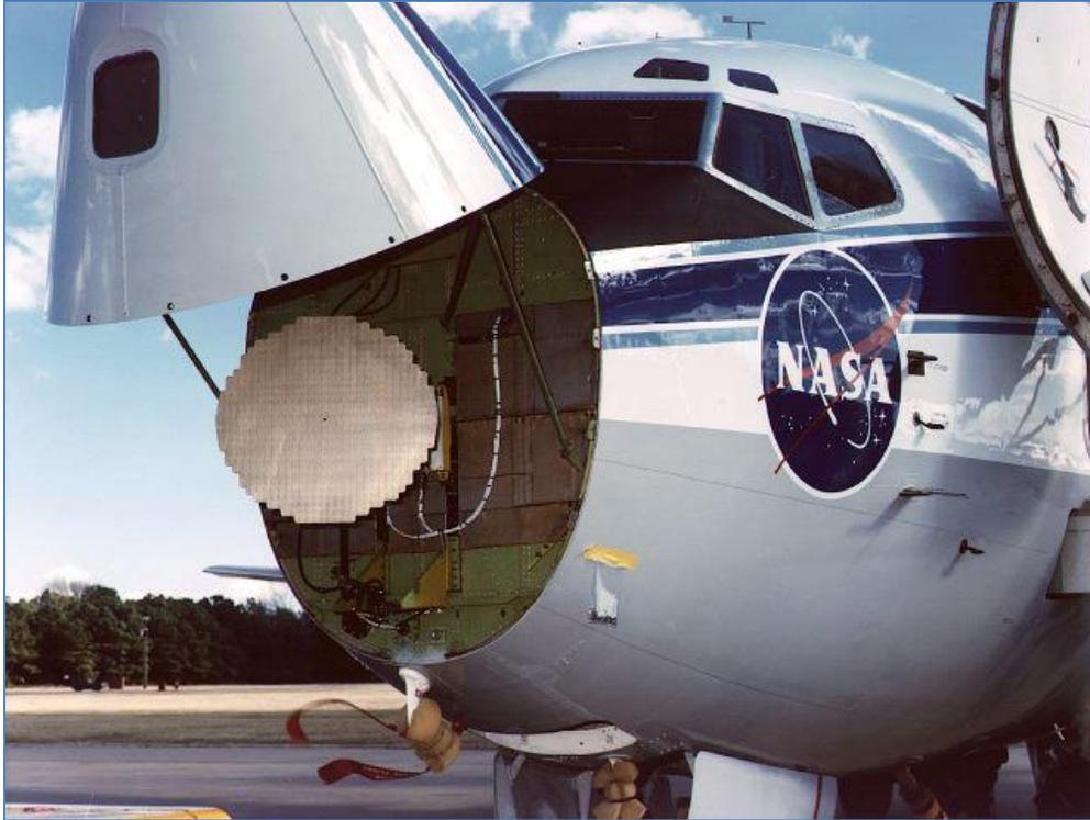
Figure 51. Airborne weather radar used in airliners.
