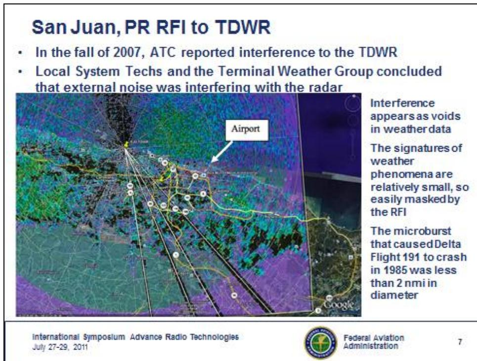
Figure 61. Example of RFI interference to TDWR from U-NII DFS devices.
