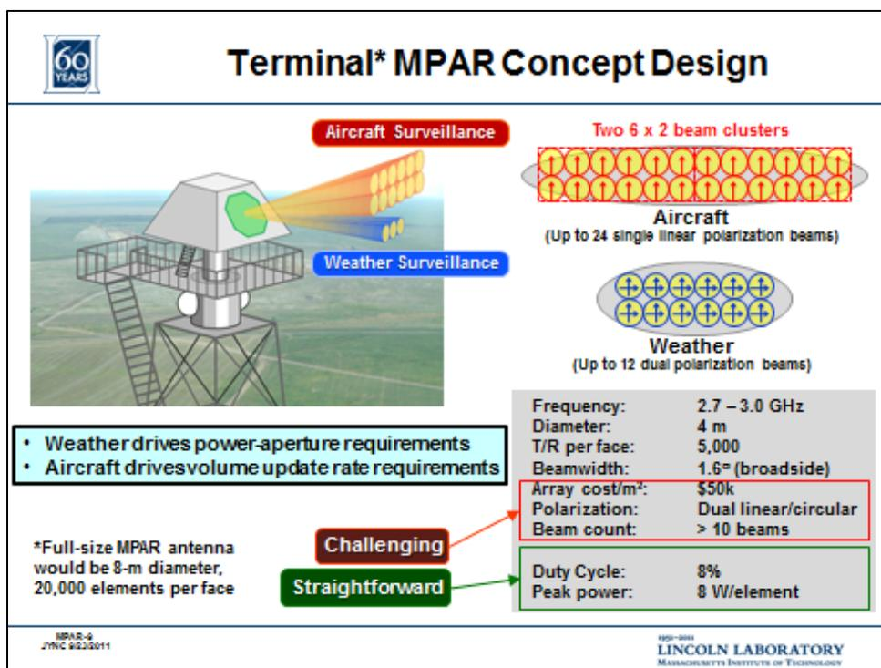
Figure 67. Terminal MPAR concept design.
