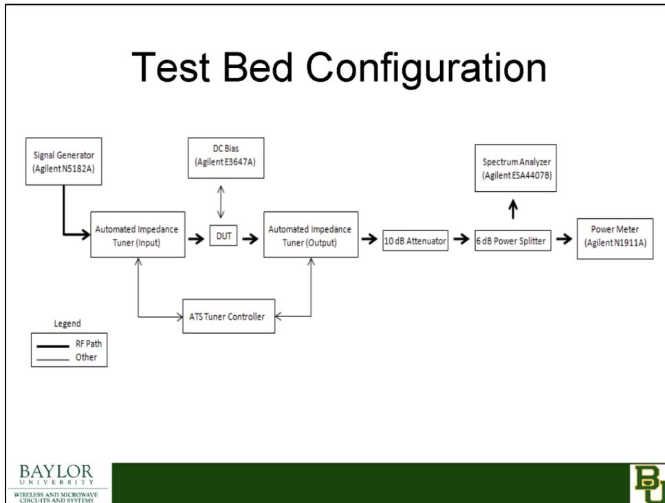
Figure 65. Waveform/Impedance optimization test bed configuration.
