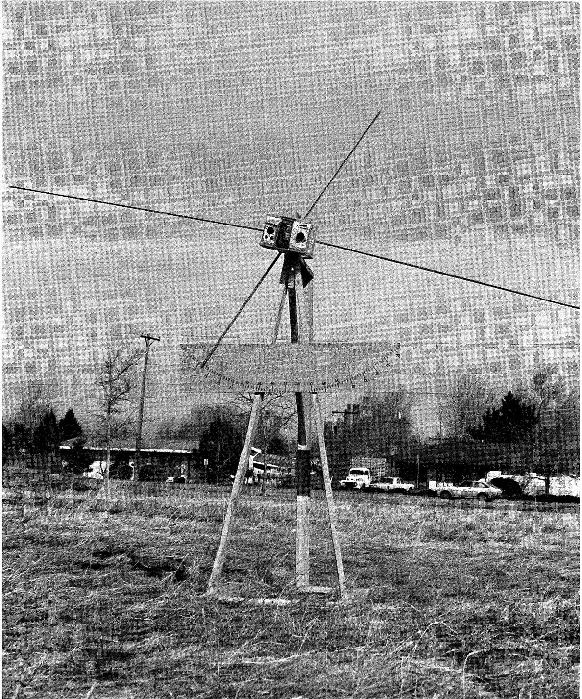
Figure B-5. Photograph of wave-tilt system--front view with antenna oriented for minimum E-field measurement.
