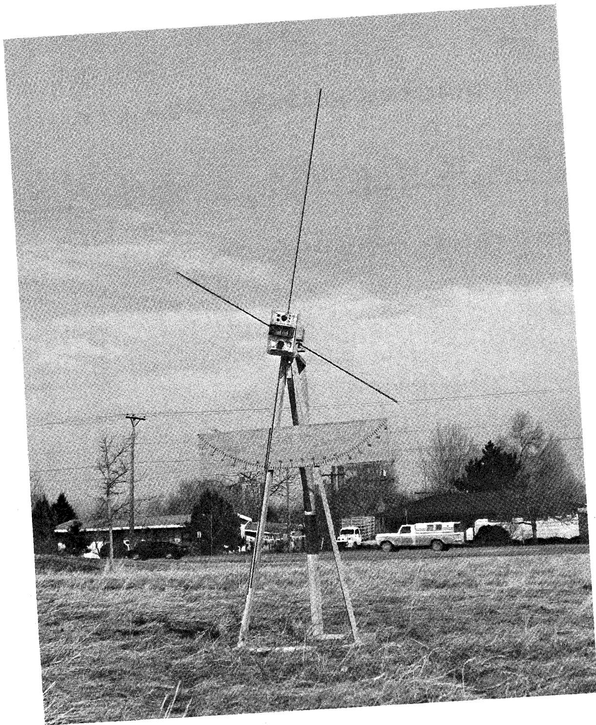
Figure B-6. Photograph of wave-tilt system--front view with antenna oriented for maximum E-field measurement.
