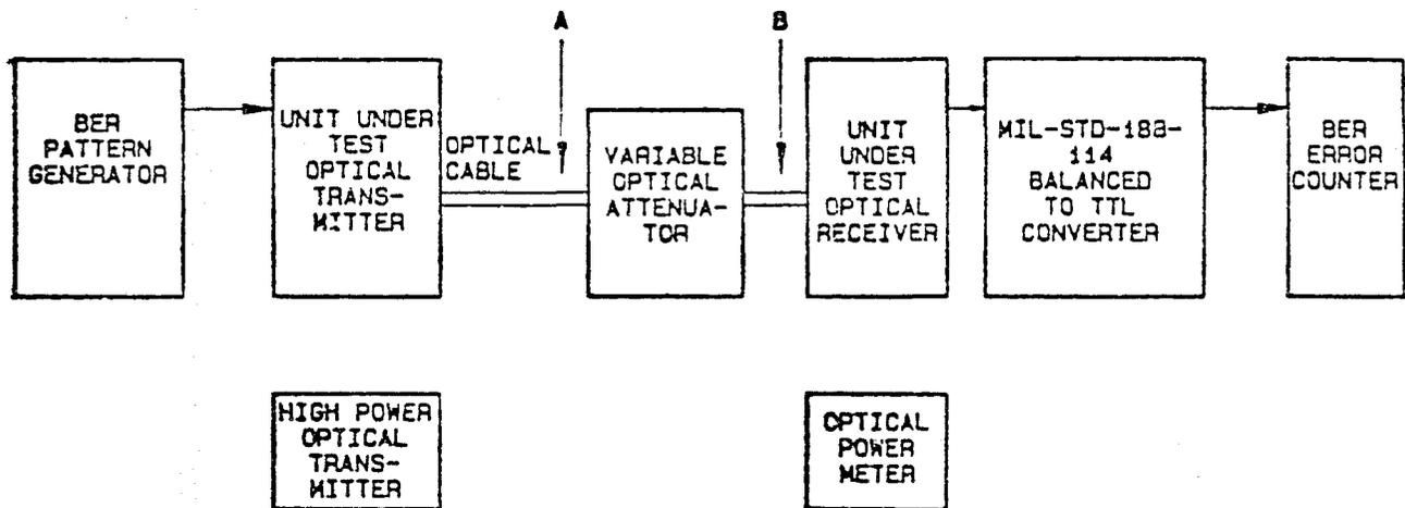
NOTE: A TTL-to-balanced converter may be used in lieu of test equipment providing a MIL-STD-188-114 interface.
