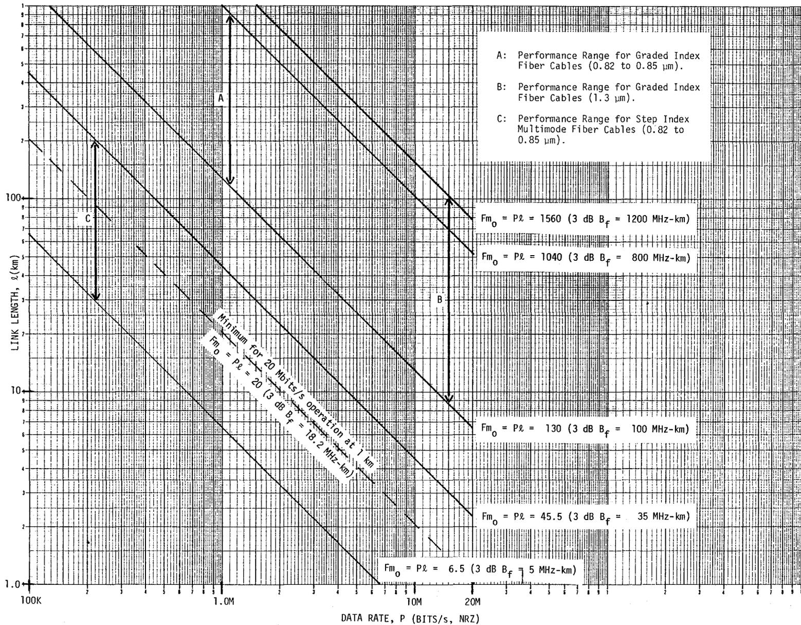
Figure 5. Figure of merit plots for distortion limits of typical step index and graded index optical fiber cables. (See Table 5 for additional fiber parameter values.)
