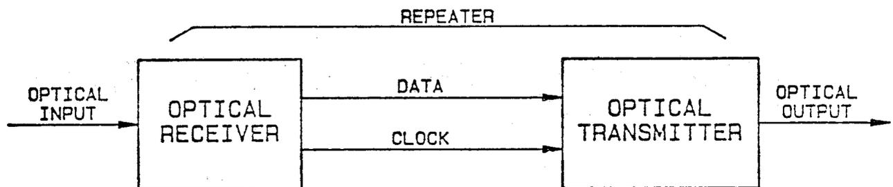
FIGURE 5. Recovered clock used as a transmit clock in repeater applications.
