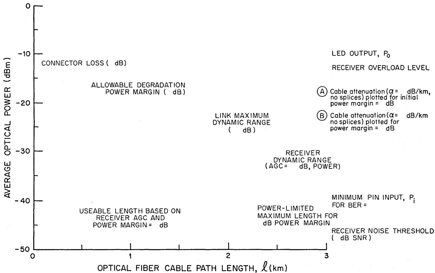
Figure 3. Graphic work sheet for short-haul optical fiber link power budget calculation.
