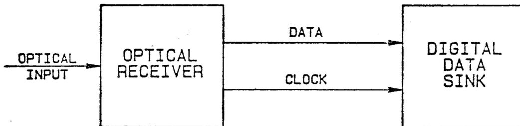
FIGURE 4. Clock recovered at optical receiver used as a data sink receive clock.
