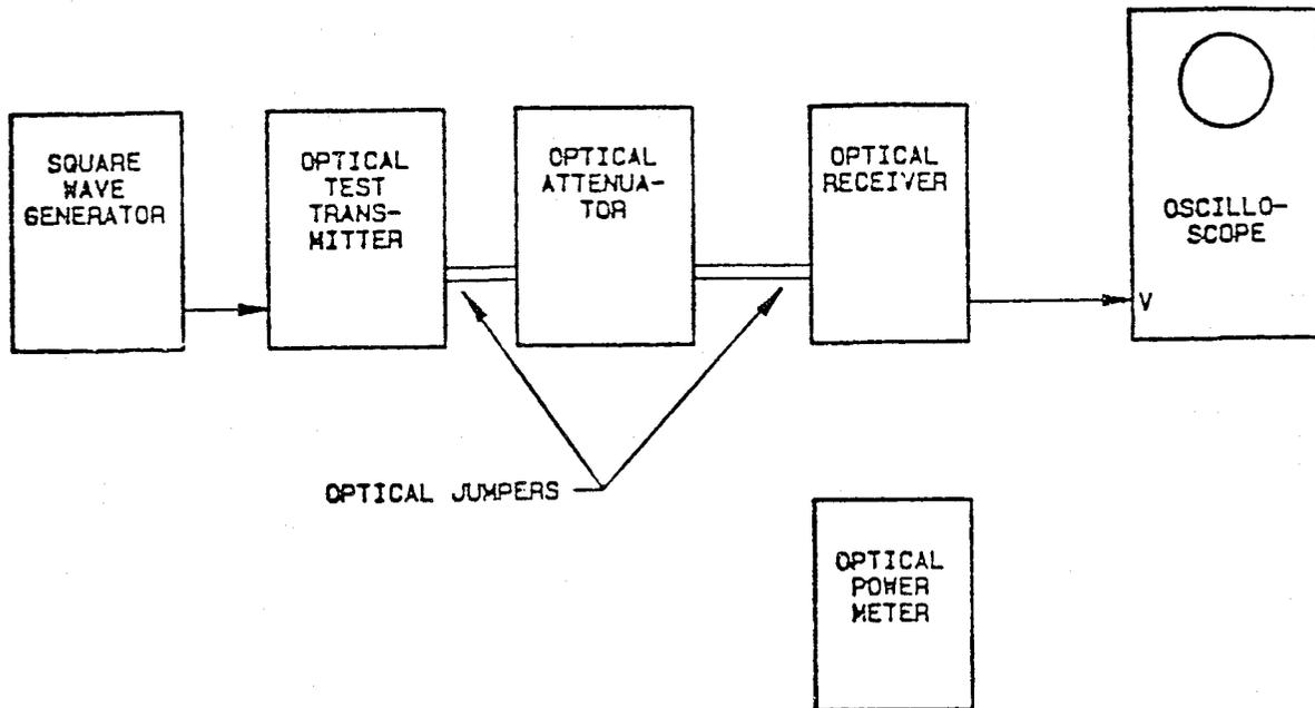
NOTE: A TTL-to-balanced converter may be used in lieu of test equipment providing a MIL-STD-188-114 interface
