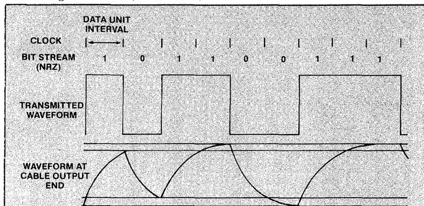
Fig. 1a Signal timing and waveforms.
