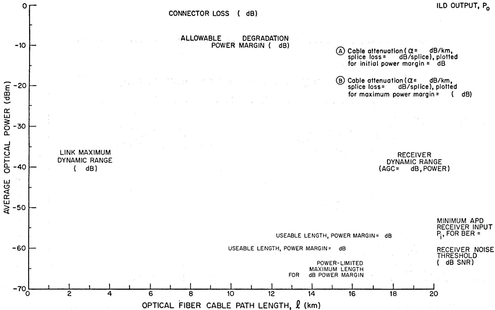
Figure 4. Graphic work sheet for long-haul optical fiber link power budget calculation.
