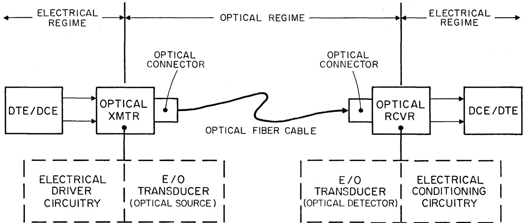
Figure C-1. Block diagram of typical optical fiber point-to-point link.
