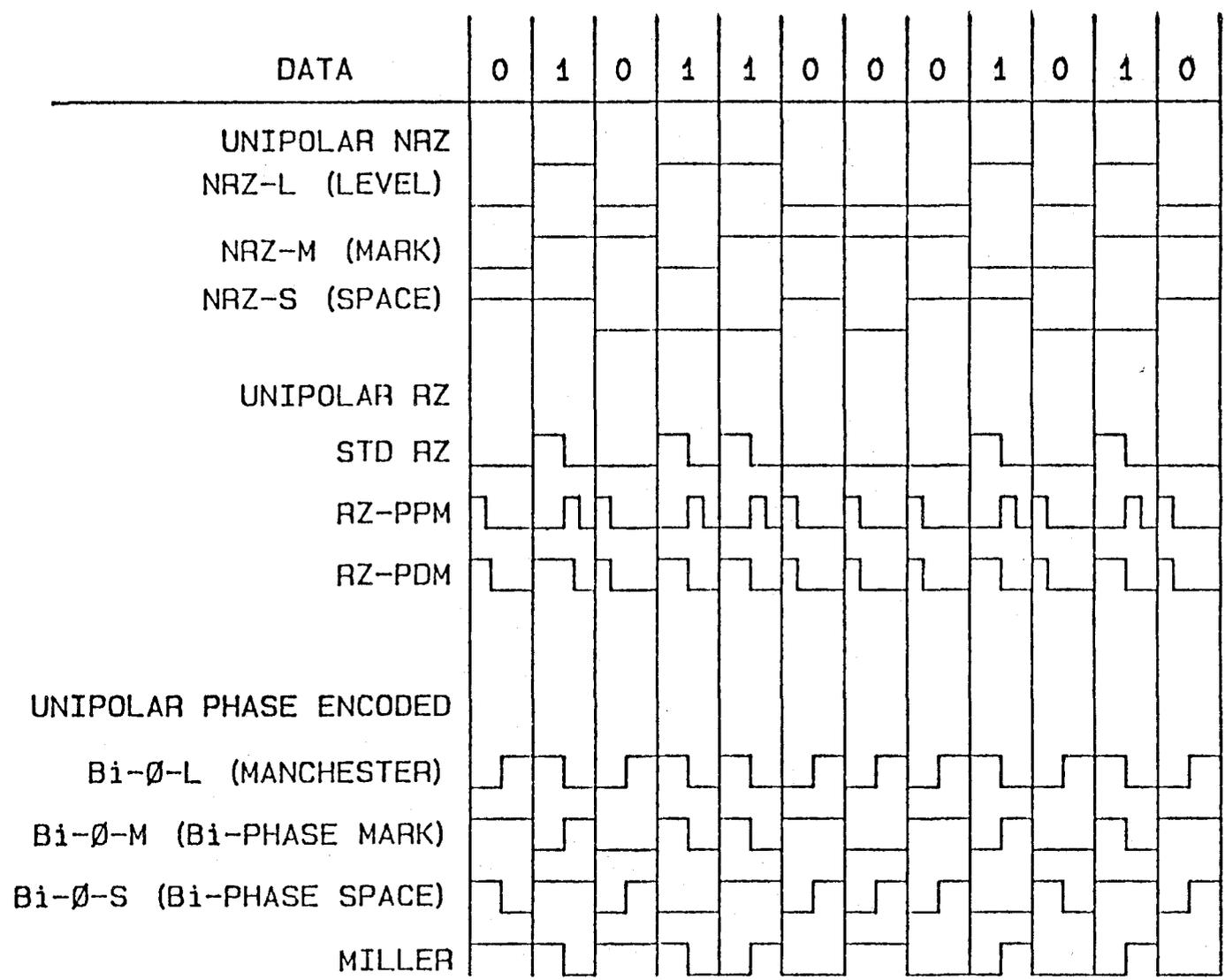
FIGURE 6. Unipolar digital signal formats. (Adapted and reprinted with permission from The Pulse, Tau-Tron, Inc.)
