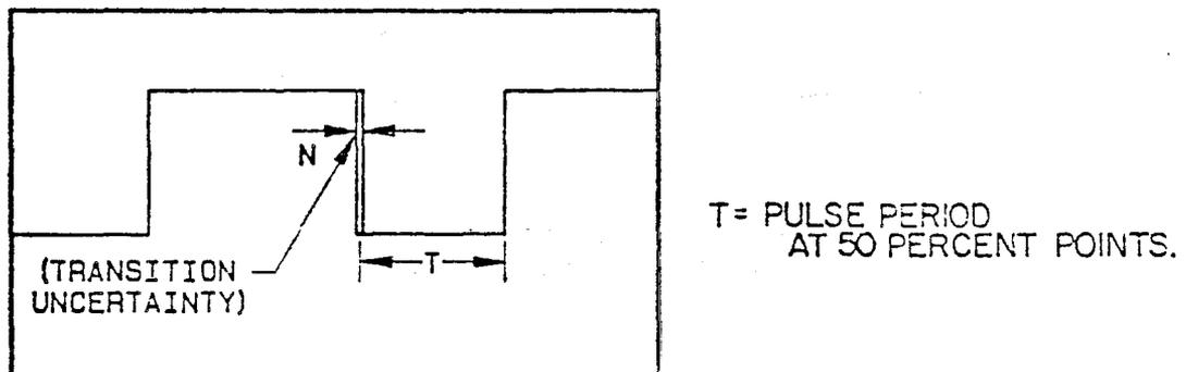
FIGURE 10. Waveform jitter.
