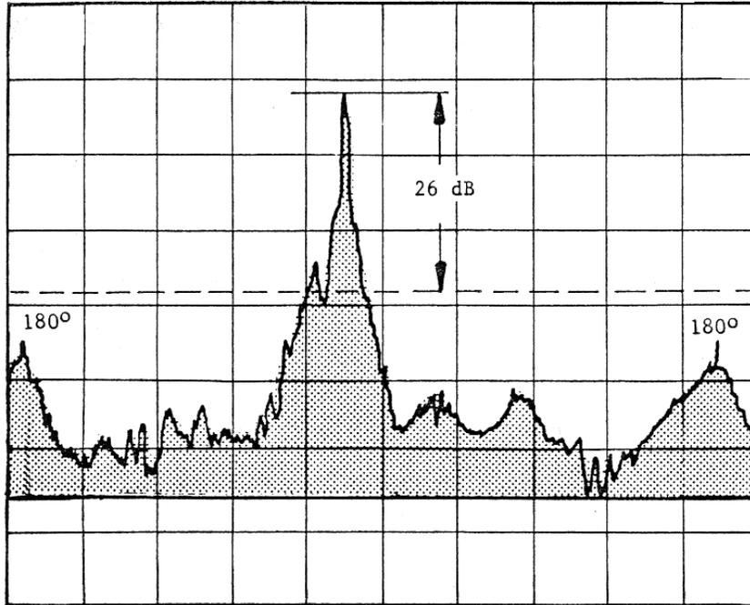
Figure 7-5a. 360-Degree Pattern of a Non-Rotating Antenna.
