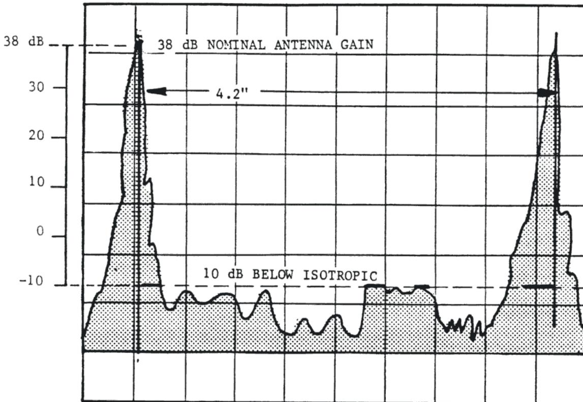
Figure 7-4. Antenna Pattern of Uniformly-Rotating Radar Showing Responses Greater than -10 dBi.
