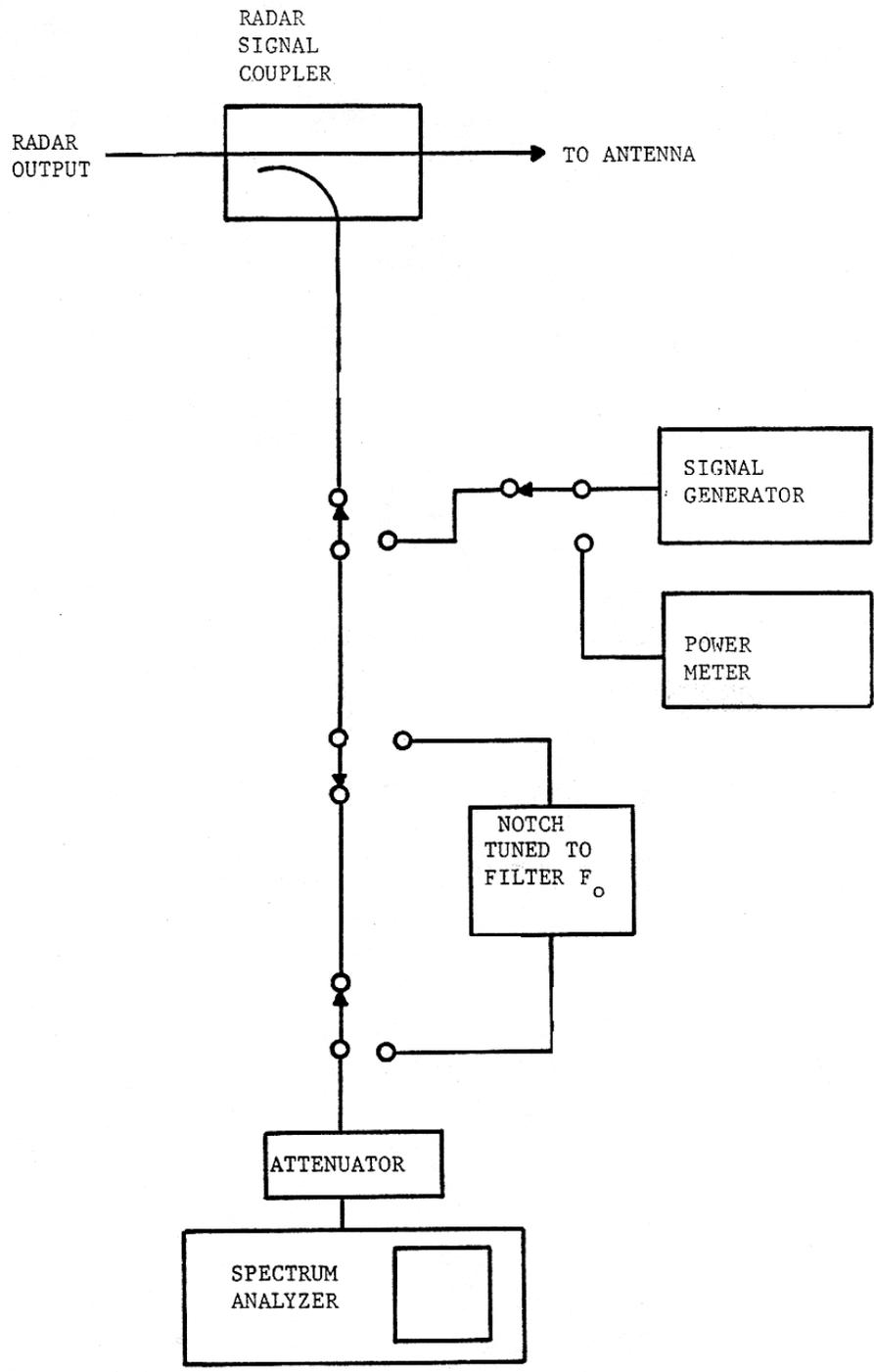
Figure 6-5. Notch Filter Test Set-Up For Emission Spectrum Measurement.
