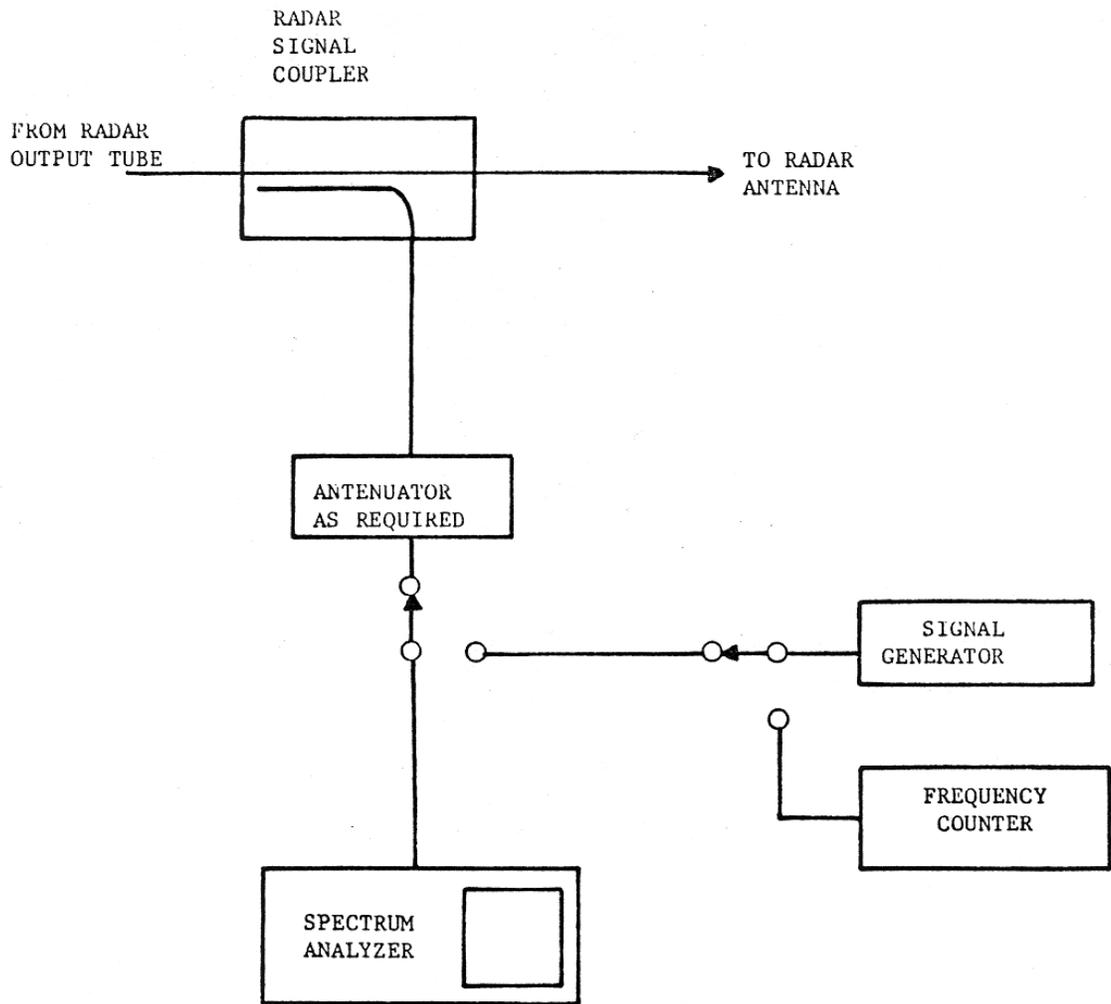
Figure 8-1. Instrumentation to Measure Drift.
