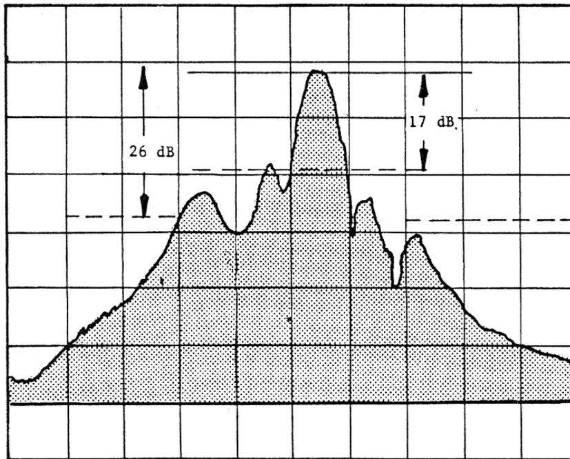
Figure 7-5b. Expanded View of Mainbeam of a Non-Rotating Antenna.
