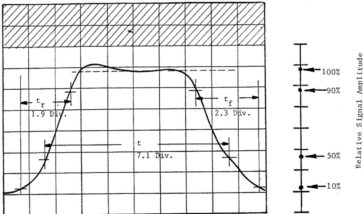
Pulse Width Scale Factor 0.5  $\mu\text{s}/\text{div.}$  Rise Time Scale Factor 0.5  $\mu\text{s}/\text{div.}$
