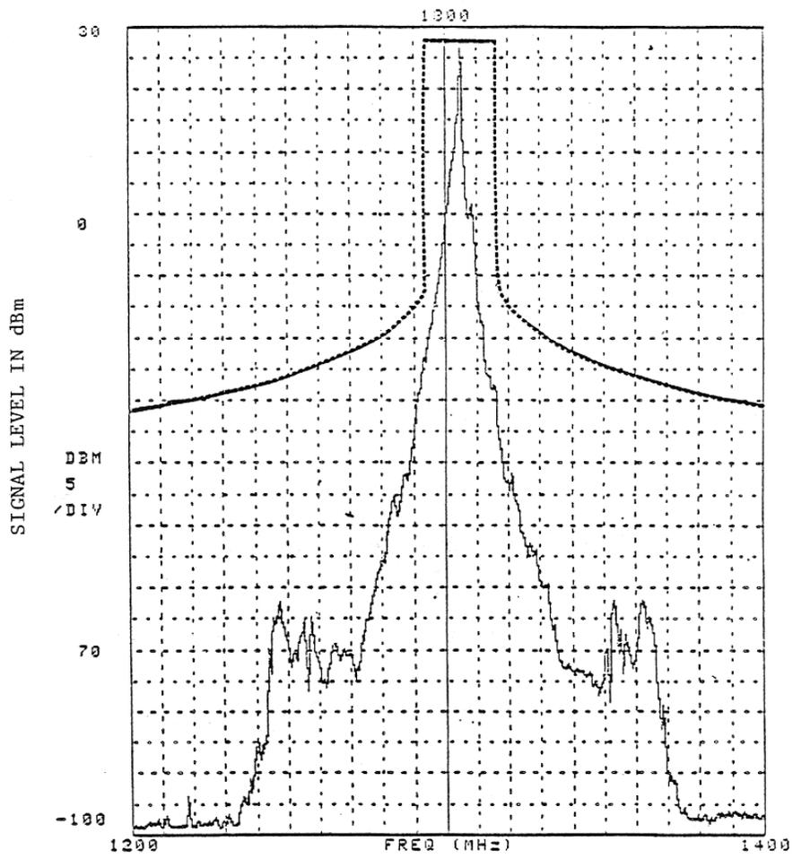
Figure 6-7. Wide-Dynamic Range Measurement of Radar Spectrum.
