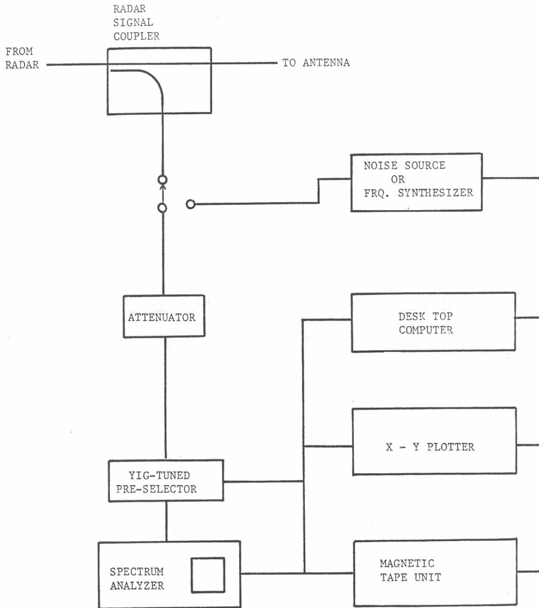
Figure 6-6. Computer-Aided Spectrum Measurement System.
