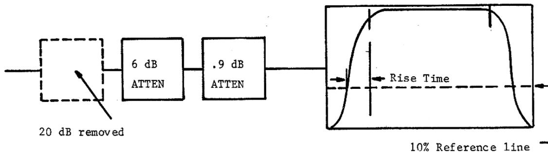
Figure 5-6. Crystal Detector Waveshapes with 10%, 50%, and 90% Attenuators.
