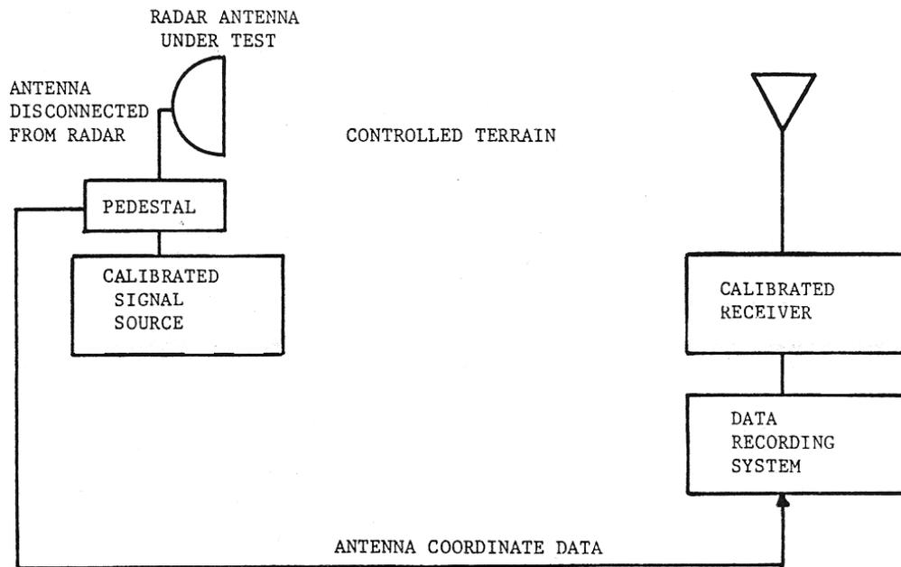
Figure 7-1. Instrumentation for Accurate Median Gain Measurement.
