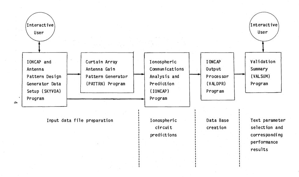
Figure 2. Interrelation between the HF antenna design and validation programs.
