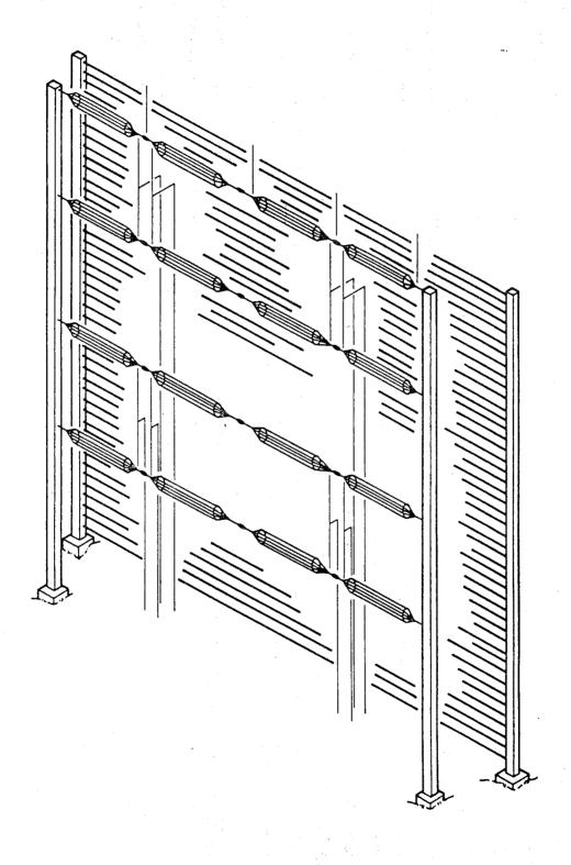
Figure 1. Curtain array with conducting screen (2 bays, 4 stacks).
