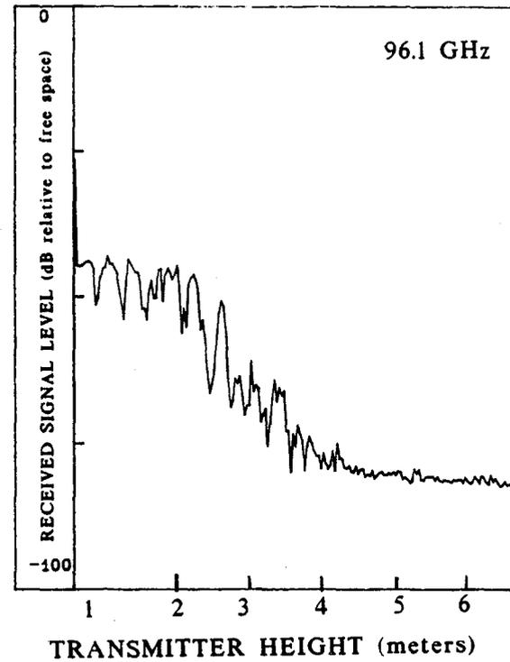
Figure 25. RSL as a function of transmitter height on path 3.
