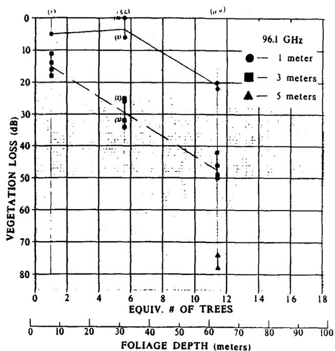
Figure 20. Vegetation loss as a function of foliage depth from peak signal pointing data on paths 1, 2, and 3.
