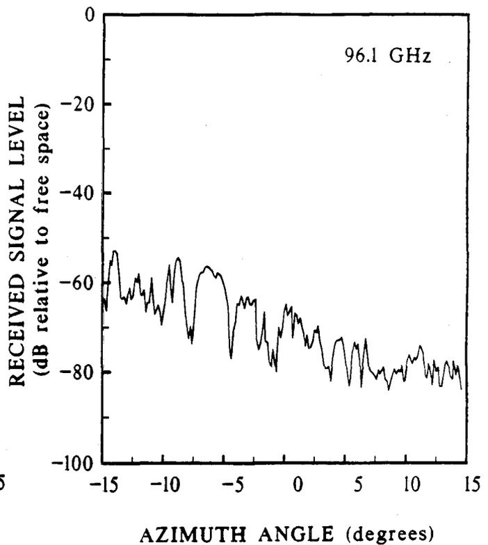
Figure 28. Azimuthal scan of RSL from backscatter measurements at an elevation angle of 95 degrees.
