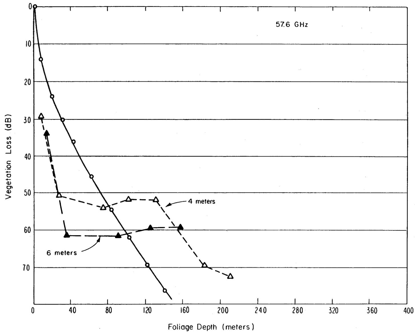
Figure A.7 Measured and predicted values of vegetation loss as a function of foliage depth for 57.6 GHz.
