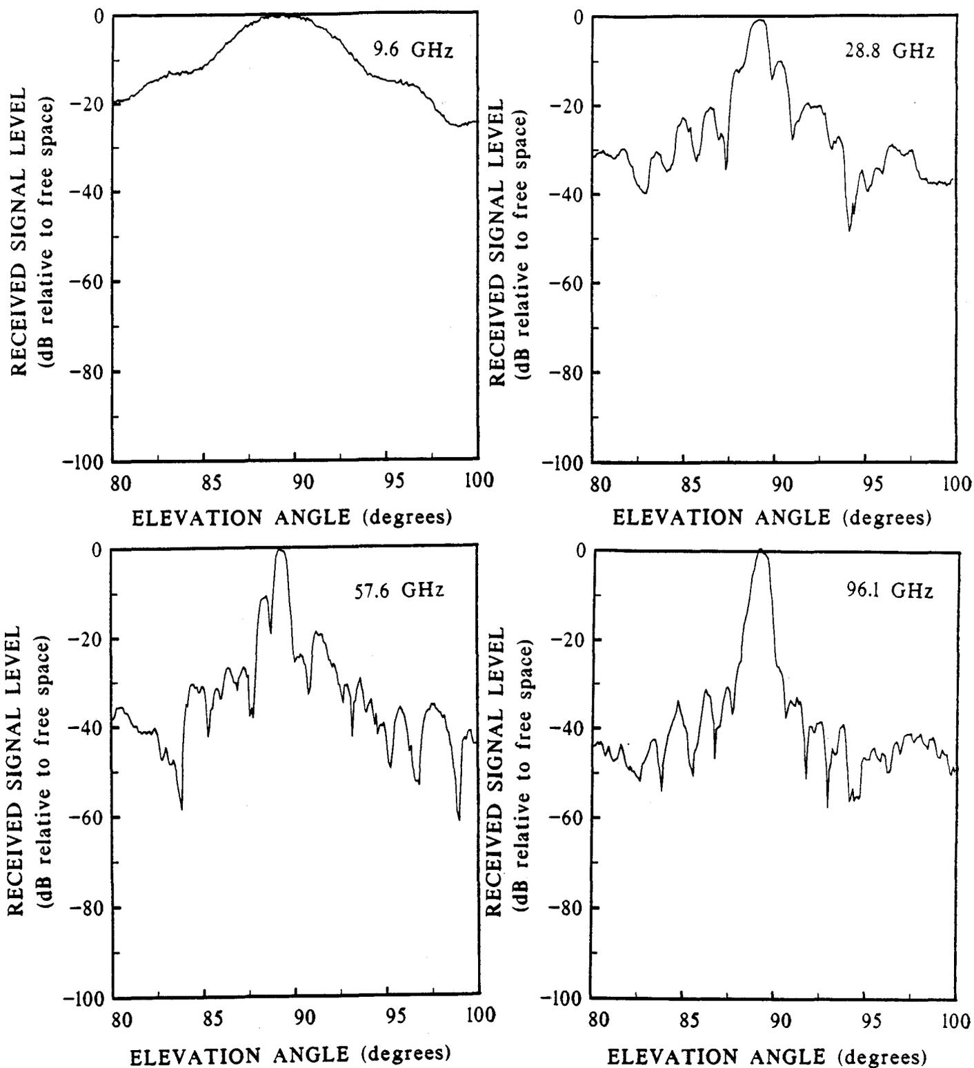
Figure 11. Elevation scan of RSL from calibration path.
