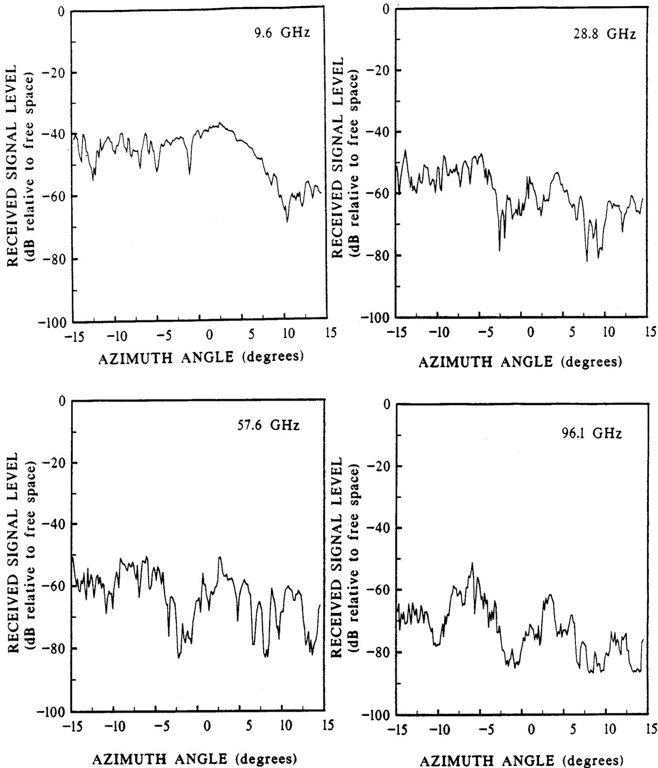
Figure 26. Azimuthal scan of RSL from backscatter measurements at an elevation angle of 90 degrees.
