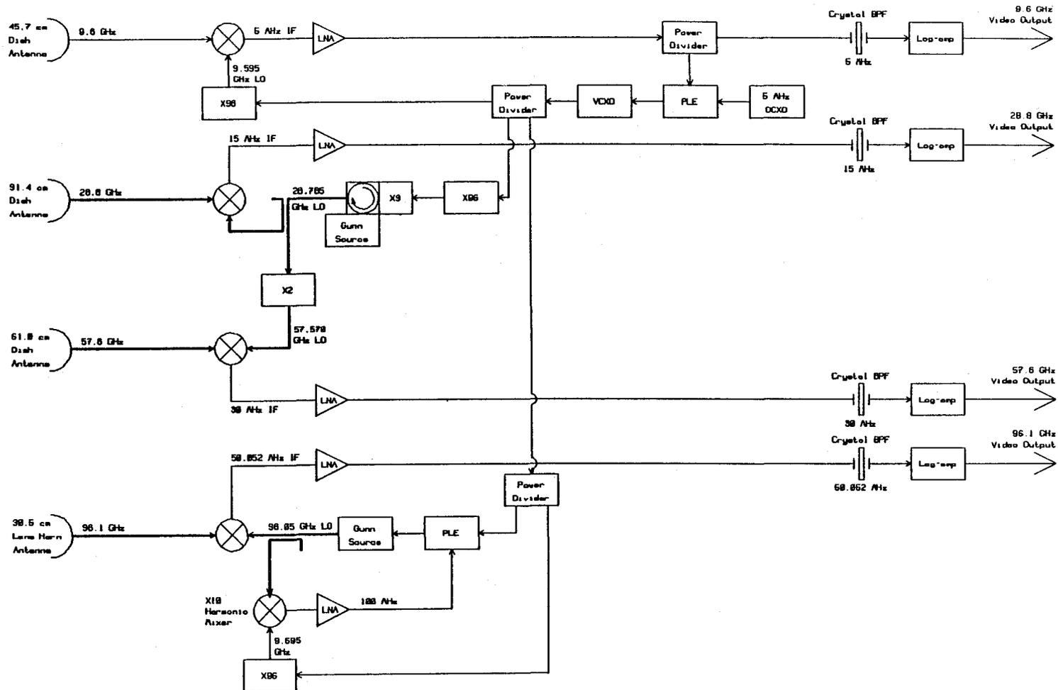
Figure 9. Block diagram of receiver equipment.
