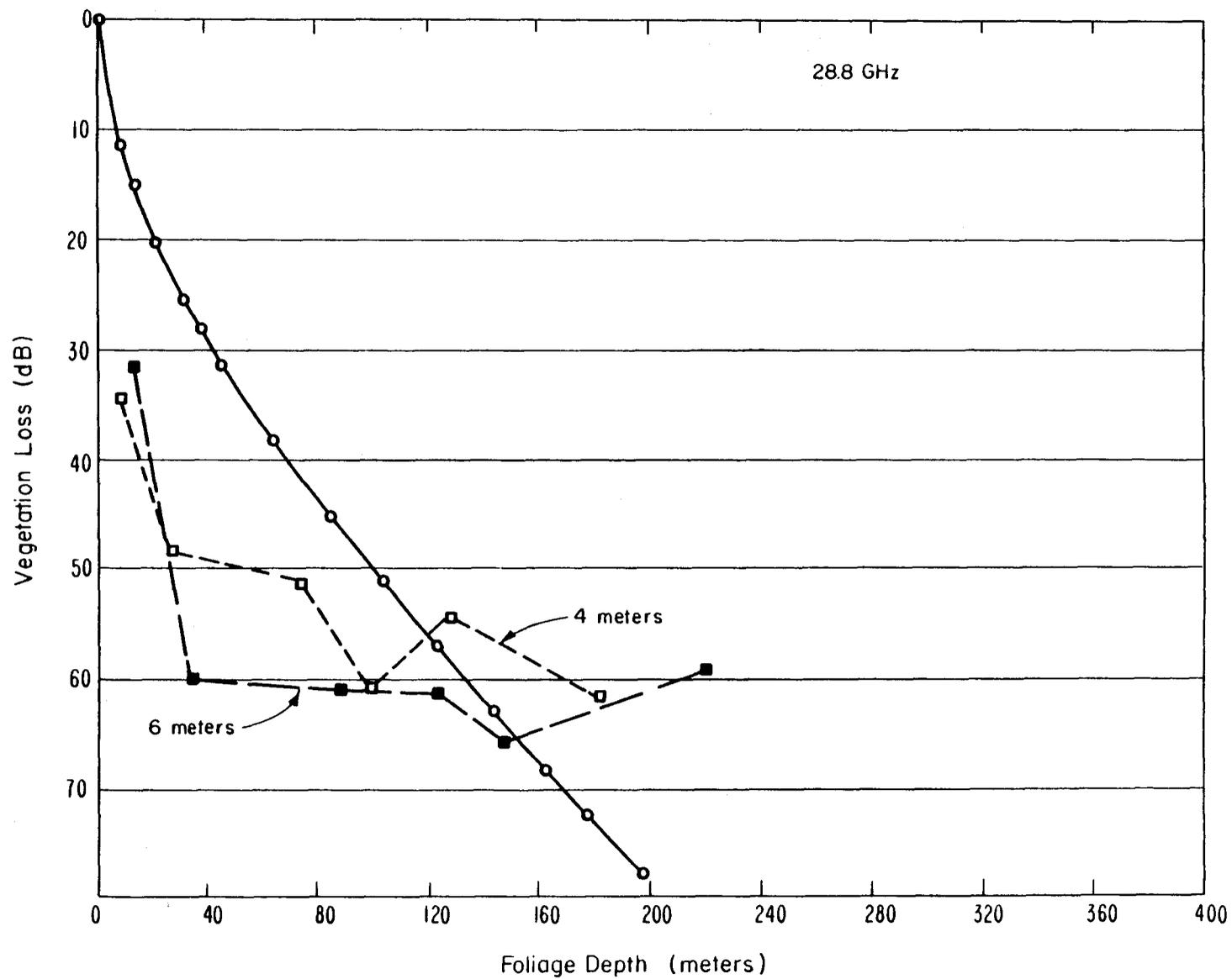
Figure A.6 Measured and predicted values of vegetation loss as a function of foliage depth for 28.8 GHz.
