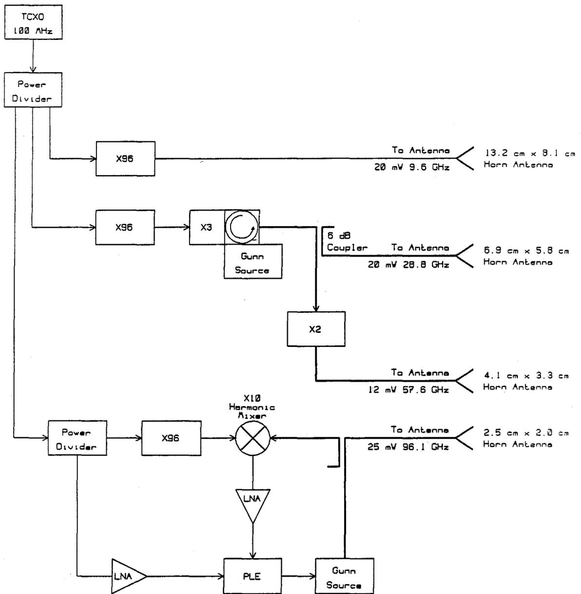
Figure 8. Block diagram of transmitter equipment.
