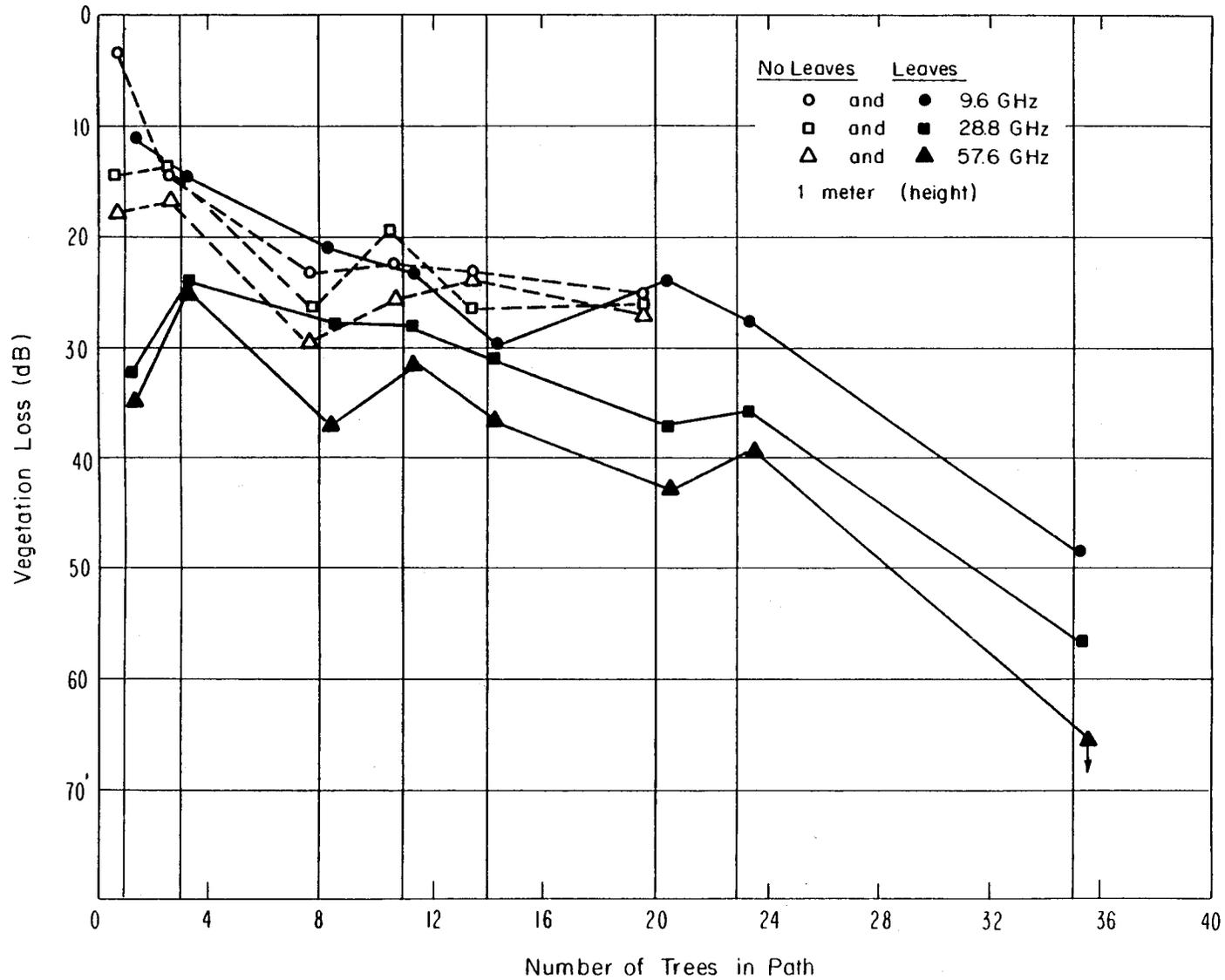
Figure A.2 Average values of vegetation loss as a function of the number of trees on path for 9.6, 28.8, and 57.6 GHz at 1 meter.
