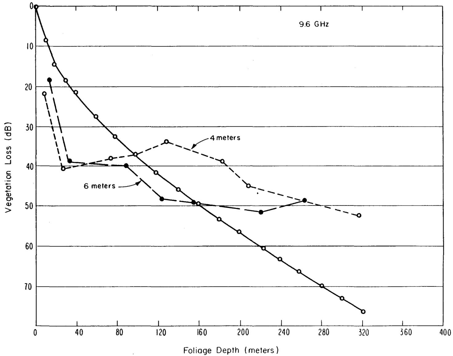
Figure A.5 Measured and predicted values of vegetation loss as a function of foliage depth for 9.6 GHz.
