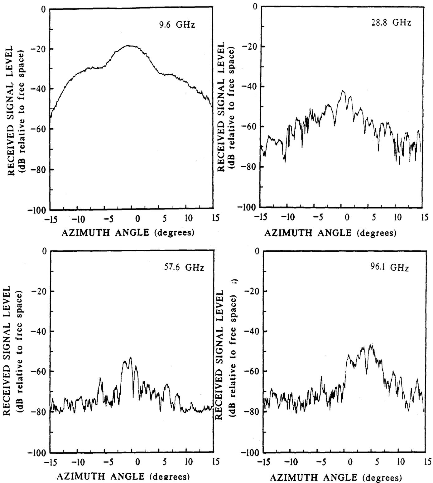
Figure 12. Copolarized azimuthal scan of RSL from path 4.
