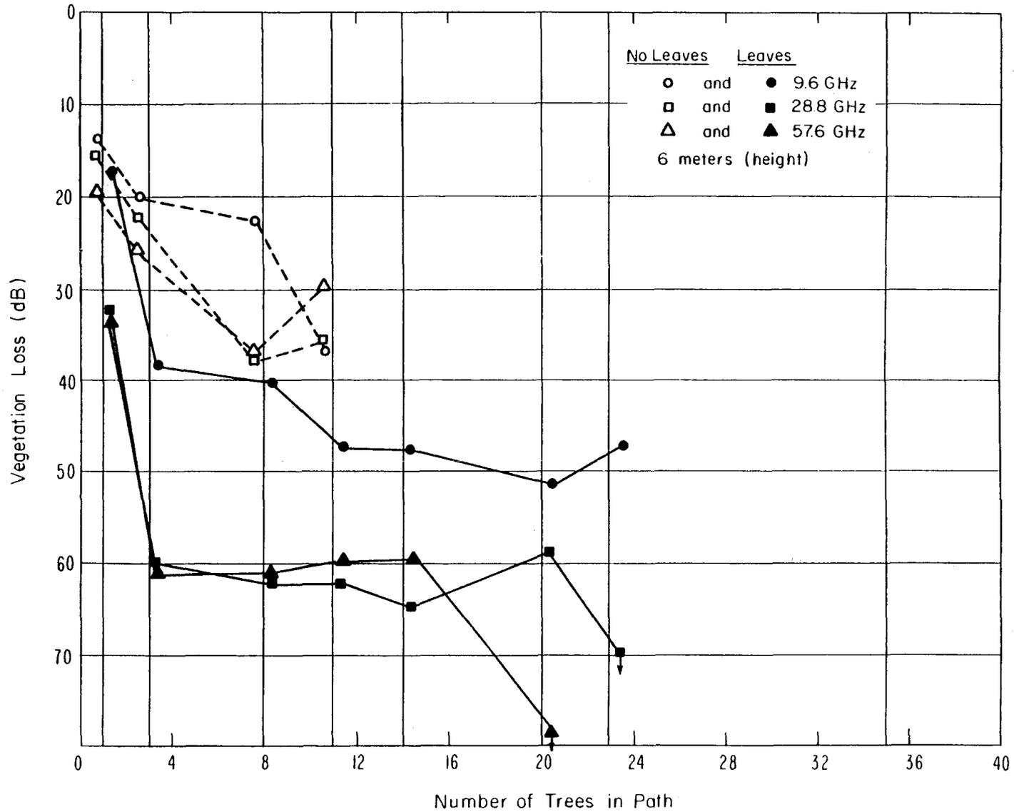
Figure A.4 Average values of vegetation loss as a function of the number of trees in path for 9.6, 28.8, and 57.6 GHz at 6 meters.
