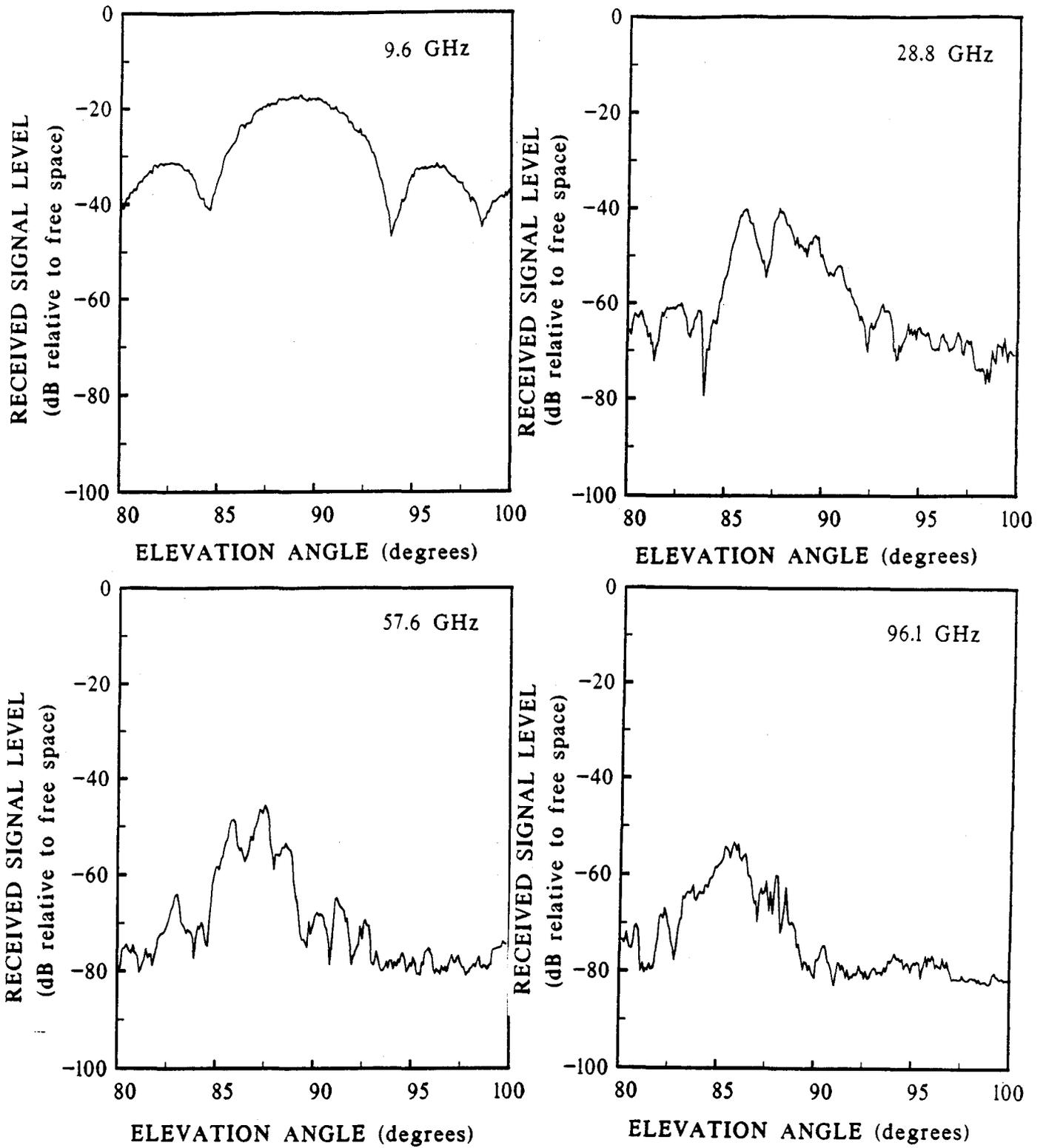
Figure 13. Copolarized elevation scan of RSL from path 4.
