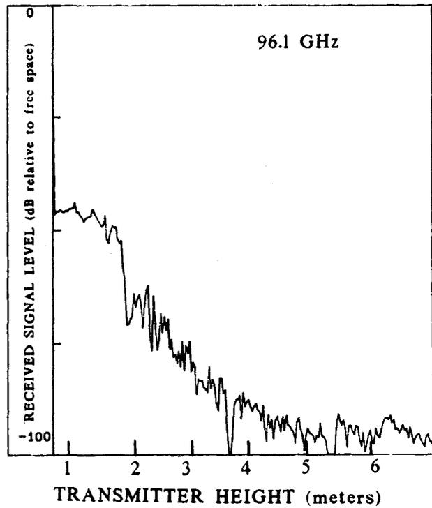
Figure 24. RSL as a function of transmitter height on path 2.
