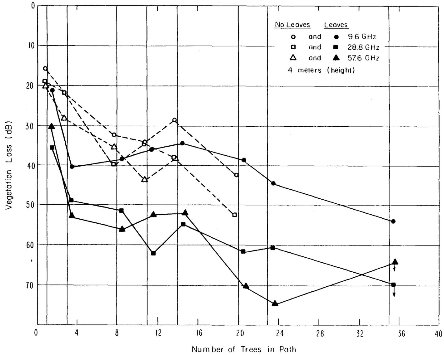
Figure A.3 Average values of vegetation loss as a function of the number of trees in path for 9.6, 28.8, and 57.6 GHz at 4 meters.
