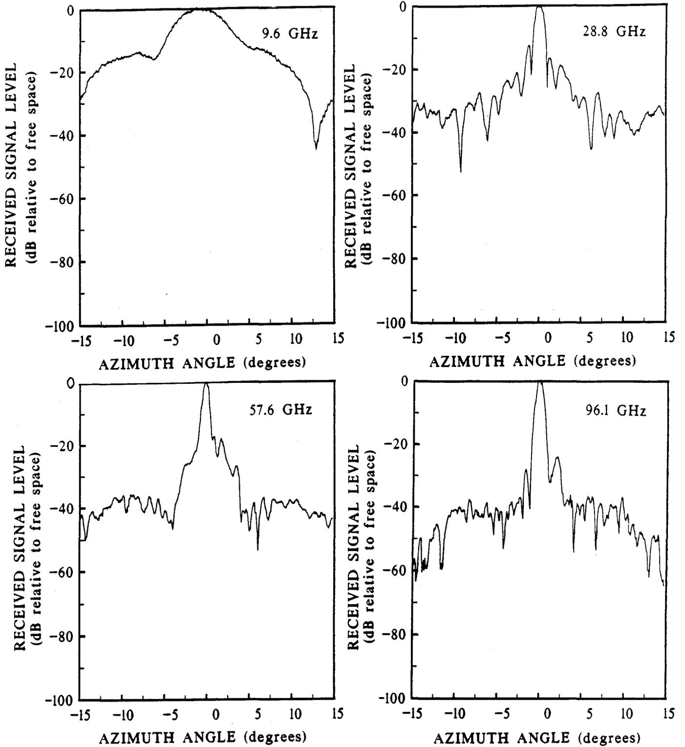
Figure 10. Azimuthal scan of RSL from calibration path.
