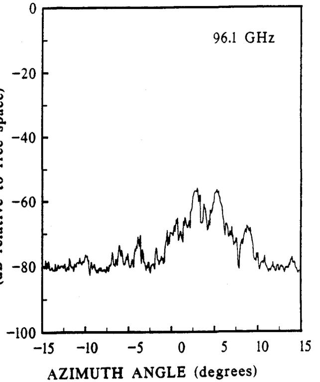
Figure 14. Cross-polarized azimuthal scan of RSL from path 4.
