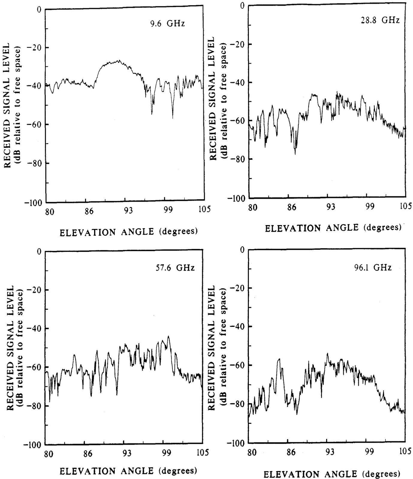
Figure 27. Elevation scan of RSL from backscatter measurements.
