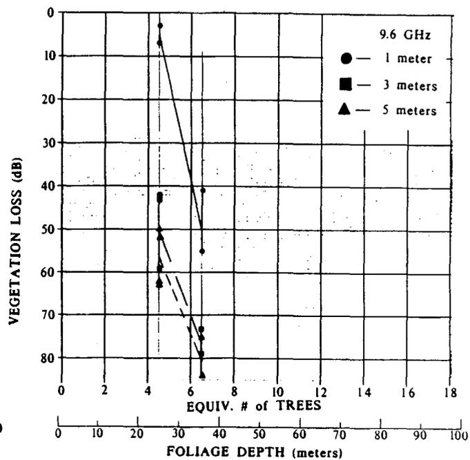
Figure 21. Vegetation loss as a function of foliage depth from peak signal pointing data on paths 8 and 9.
