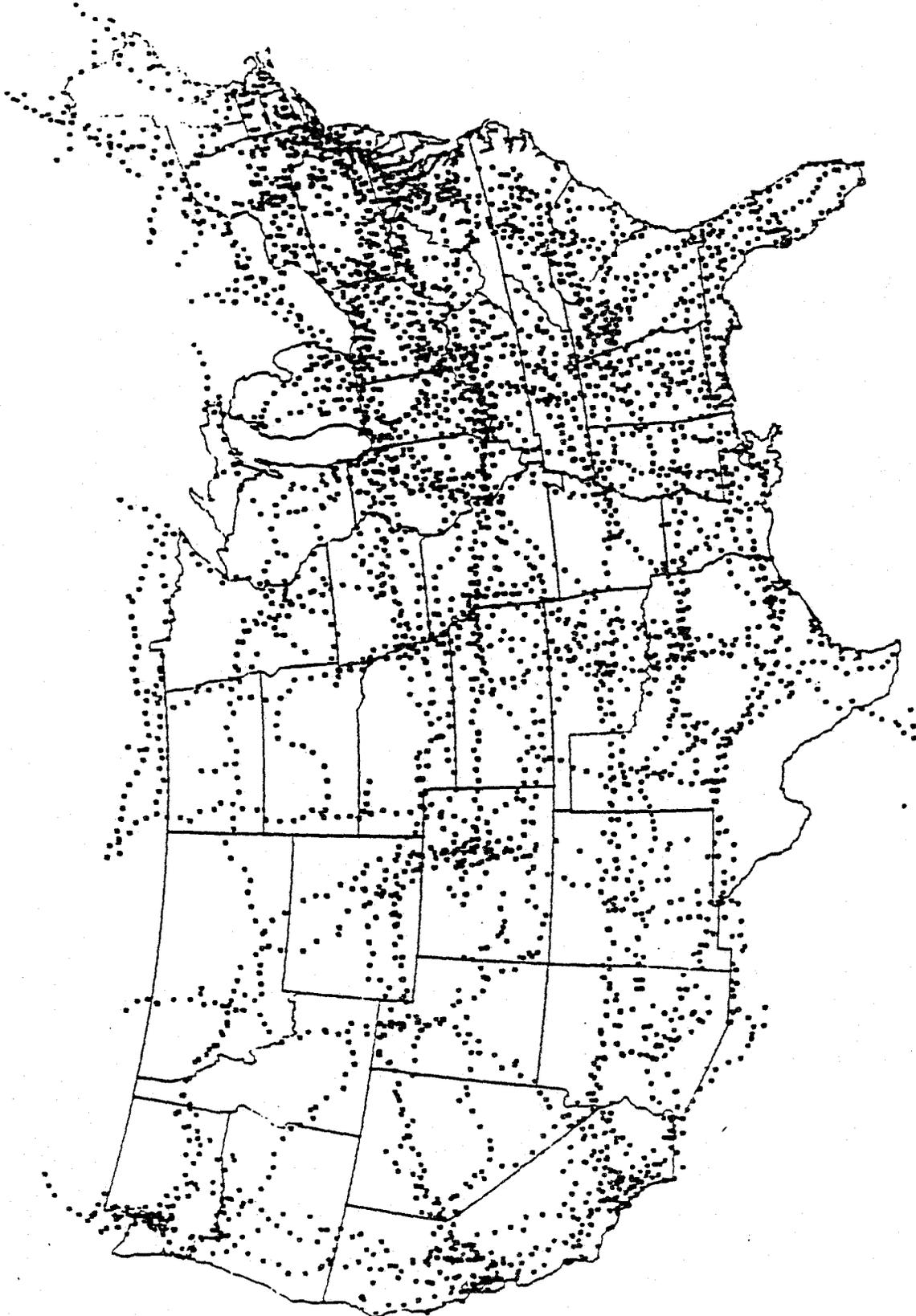
Figure 4-6. 4 GHz point-to-point common carrier stations.
