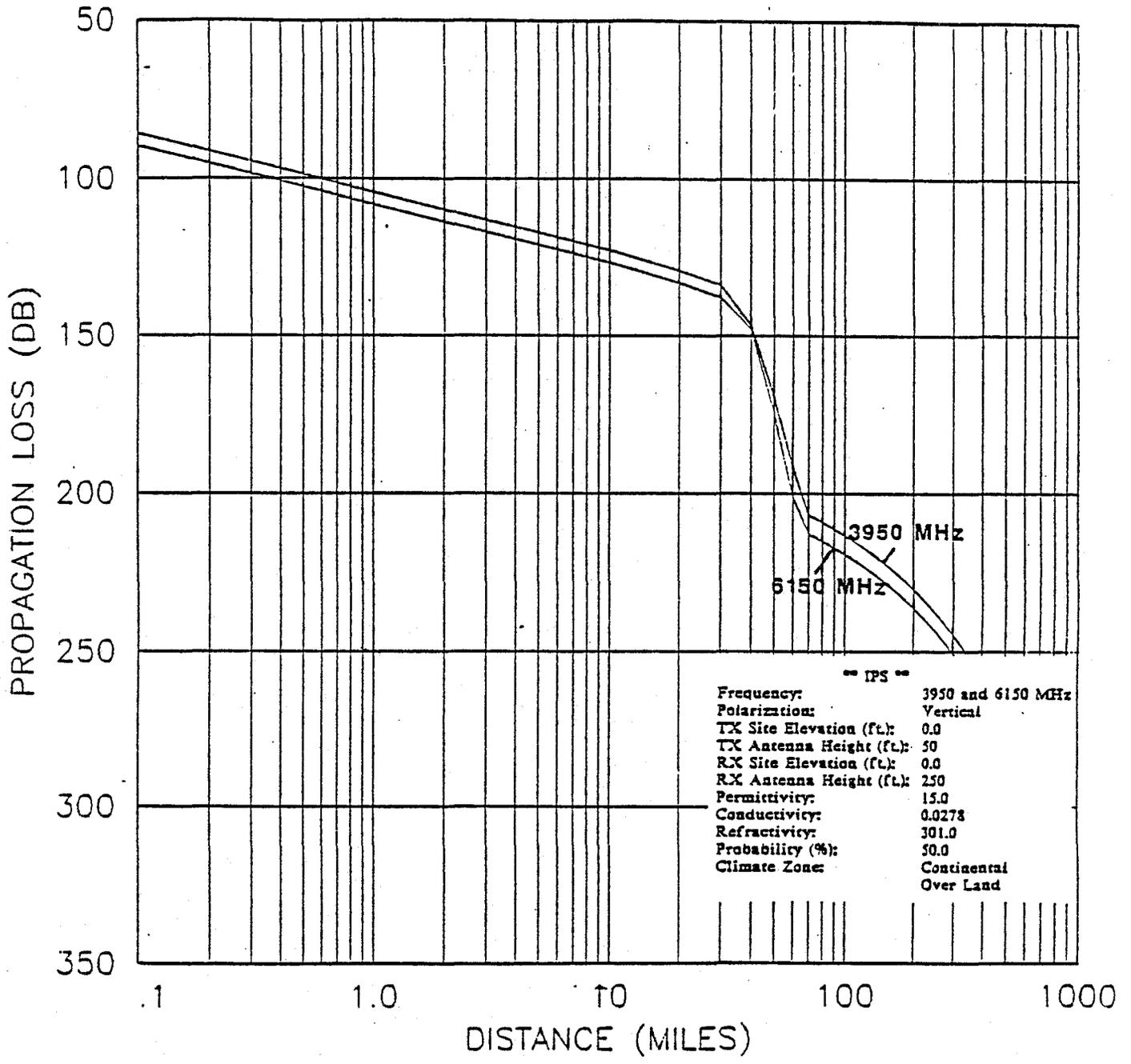
Figure 5-22. Propagation Loss versus Distance Separation curves.
