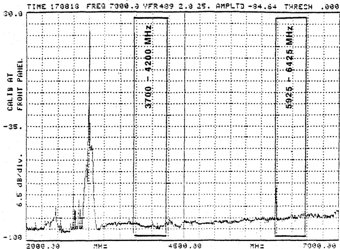
Figure 5-12. Radiated spectrum measurements of the test and evaluation NEXRAD radar at Norman, OK, (pulwidth = 1.67  $\mu$ s).
