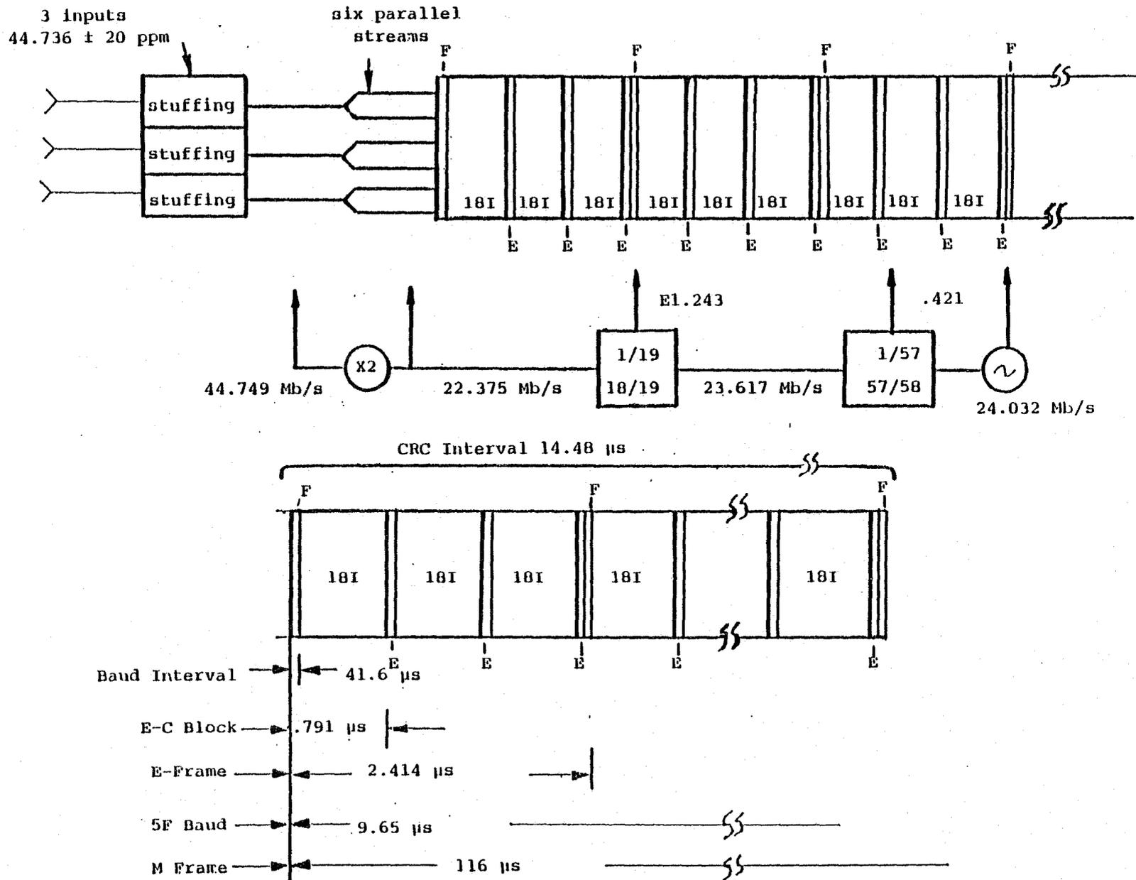
Figure A-4. Three (3) DS-3 Signals in 30 MHz, Error Correcting 64-QAM.
