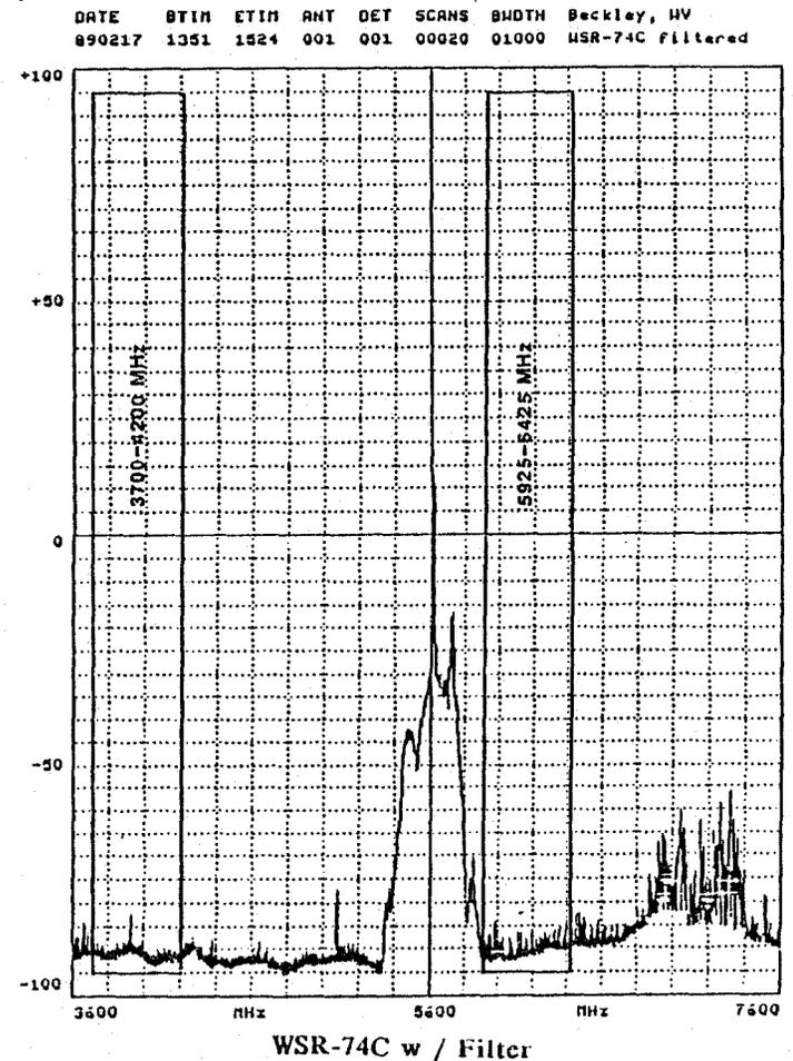
Figure 6-2. Radiated spectrum measurements of the WSR-74C radar at Beckley, WVA without and with an RF Filter.
