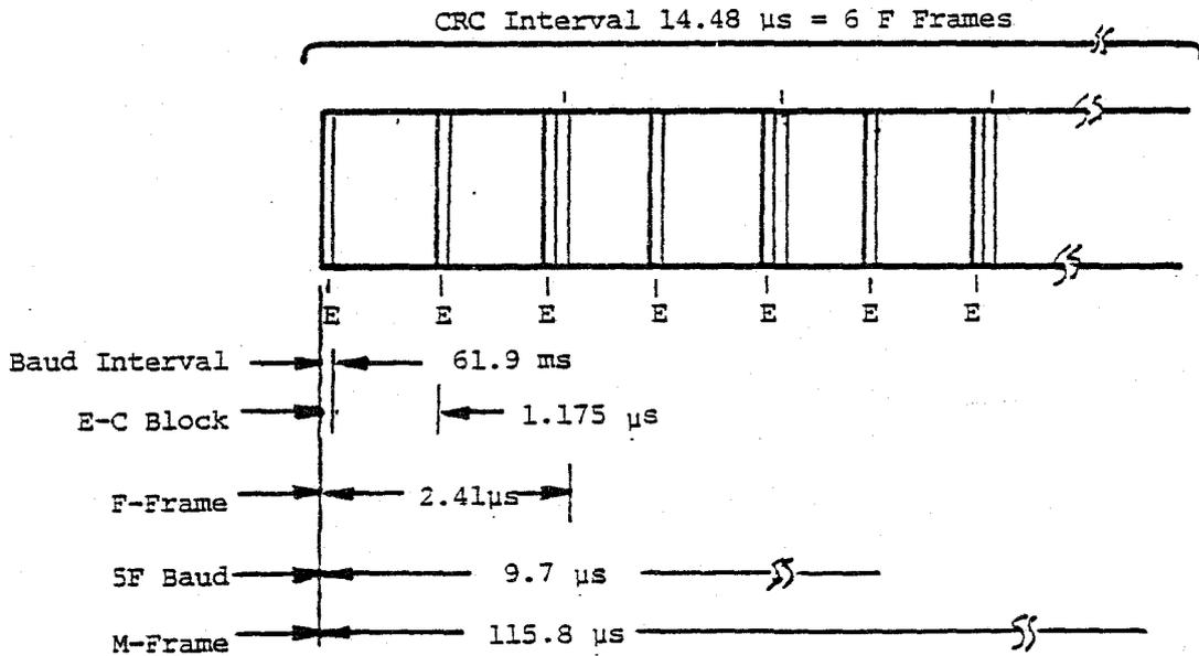
Figure A-5. Two (2) DS-3 IN 20 MHz, Error Correcting 64-QAM.
