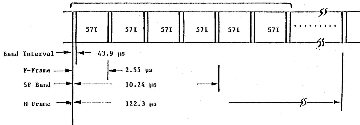
Figure A-3. Three (3) DS-3 Signals in 30 MHz, Non-Error Correcting 64-QAM.
