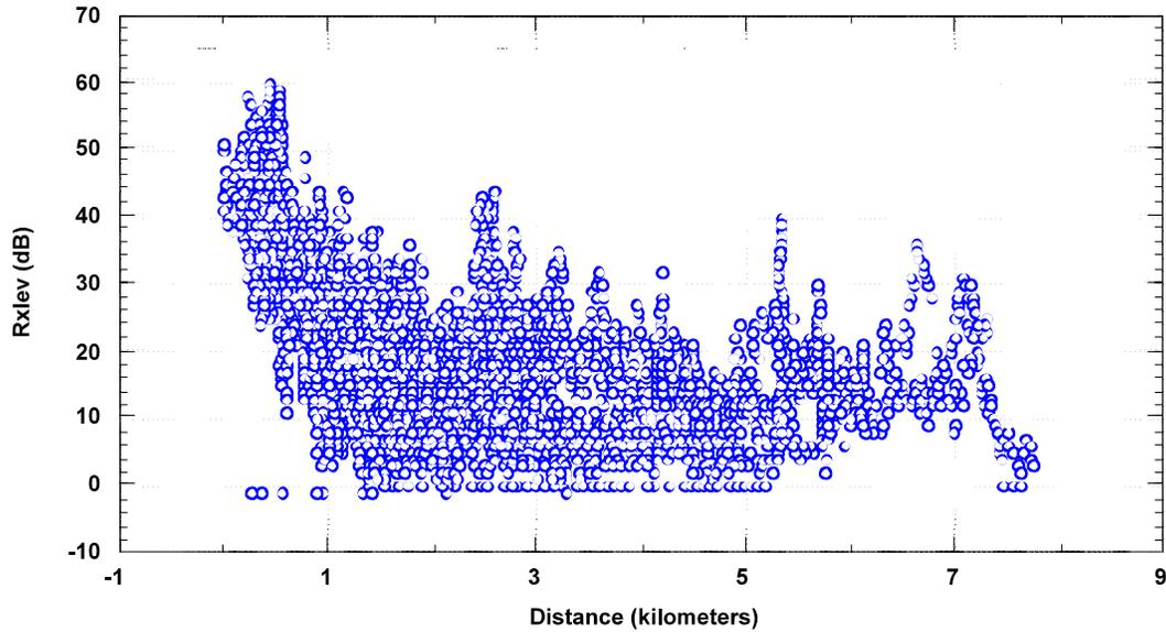
Figure 3.8. Downlink Rxlev vs. distance (TAG 5, WCO cell).
