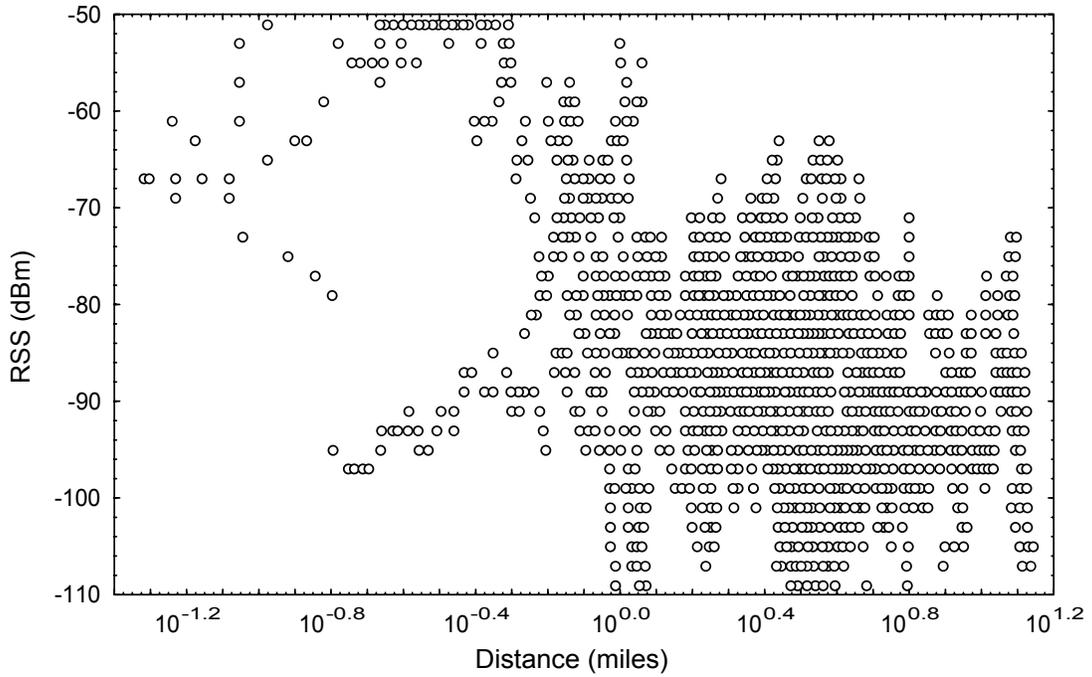
Figure 5.2. Downlink received signal strength (RSS) vs. distance (TAG 4, TMCO cell).
