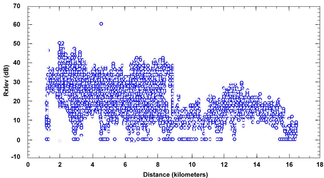
Figure 3.14. Downlink Rxlev vs. distance (TAG 5, GMM cell).
