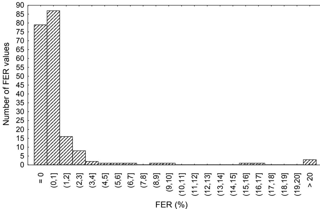
Figure 4.7. Histogram of downlink frame error rate (FER; TAG 2, TMCO cell).
