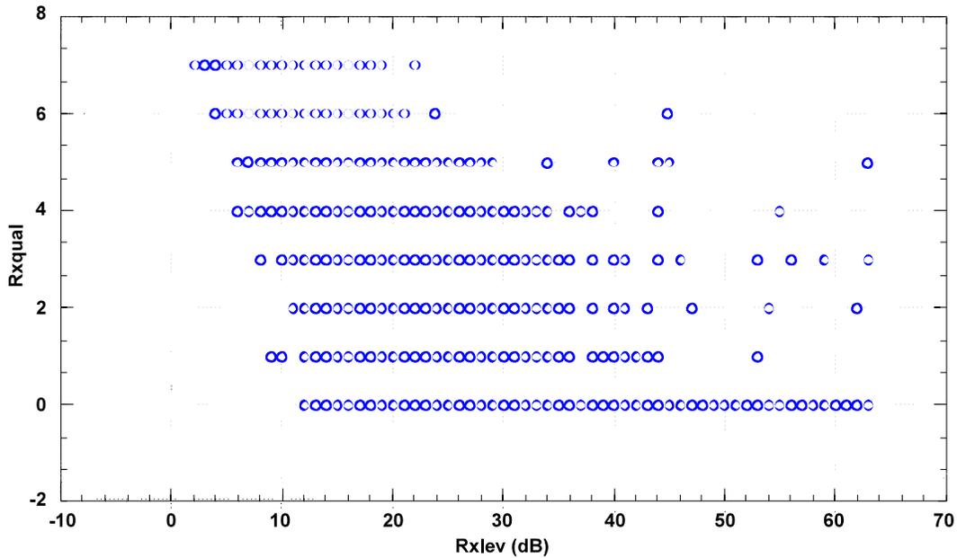
Figure 3.7. Downlink Rxqual vs. Rxlev (TAG 5, TMCO cell).
