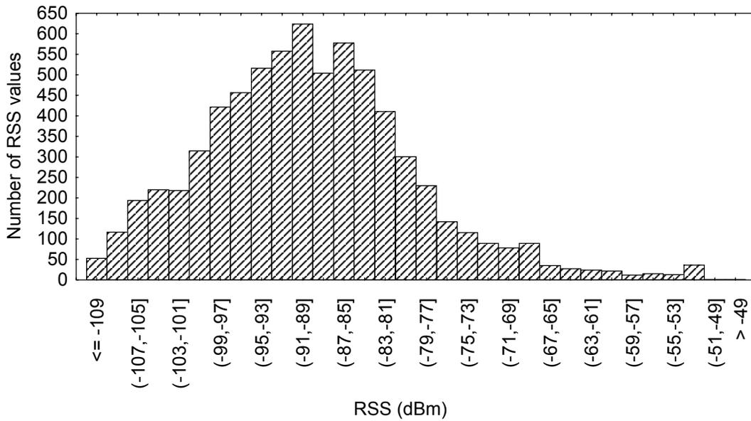
Figure 5.3. Histogram of downlink received signal strength (RSS) values (TAG 4, TMCO cell).
