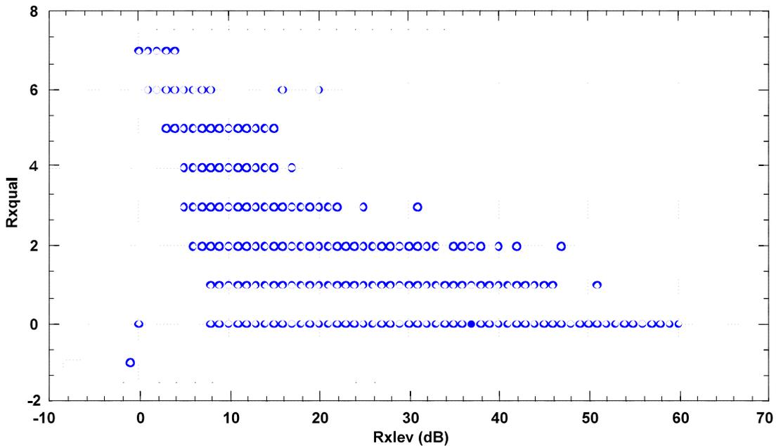
Figure 3.13. Downlink Rxqual vs. Rxlev (TAG 5, WCO cell).
