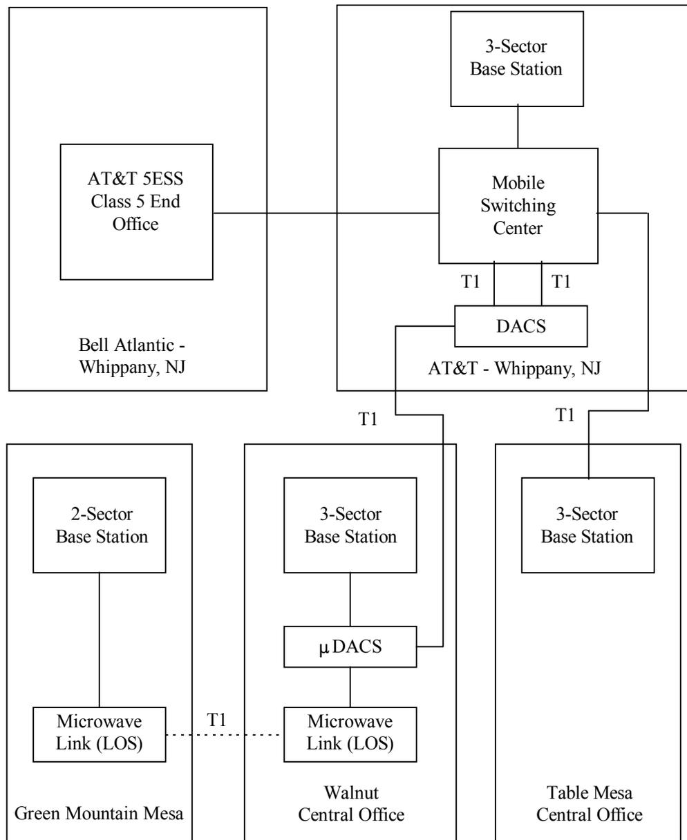
Figure 5.1. Block diagram of the TAG 4 test system configuration.
