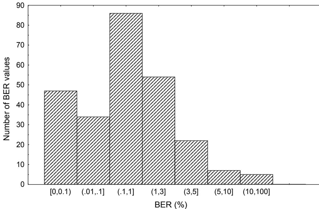
Figure 8.6. Histogram of average uplink bit error rate (BER; TAG 1, TMCO cell).
