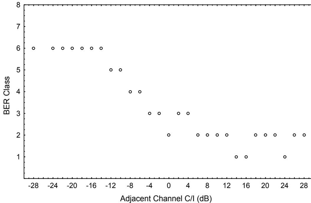
Figure 5.17. Average bit error rate (BER) class vs. carrier-to-interference ratio (C/I) for the adjacent channel interference case (TAG 4).
