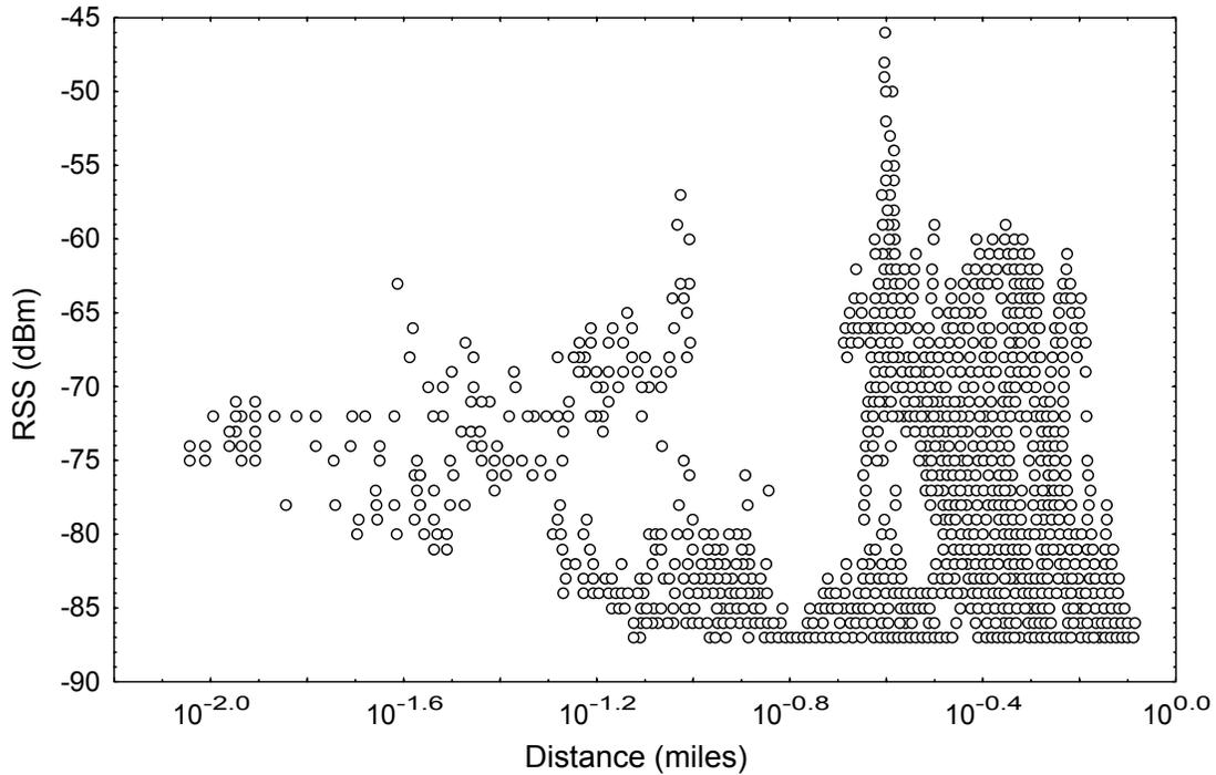
Figure 6.1. Downlink received signal strength (RSS) vs. distance (TAG 7, TMC0 cell).
