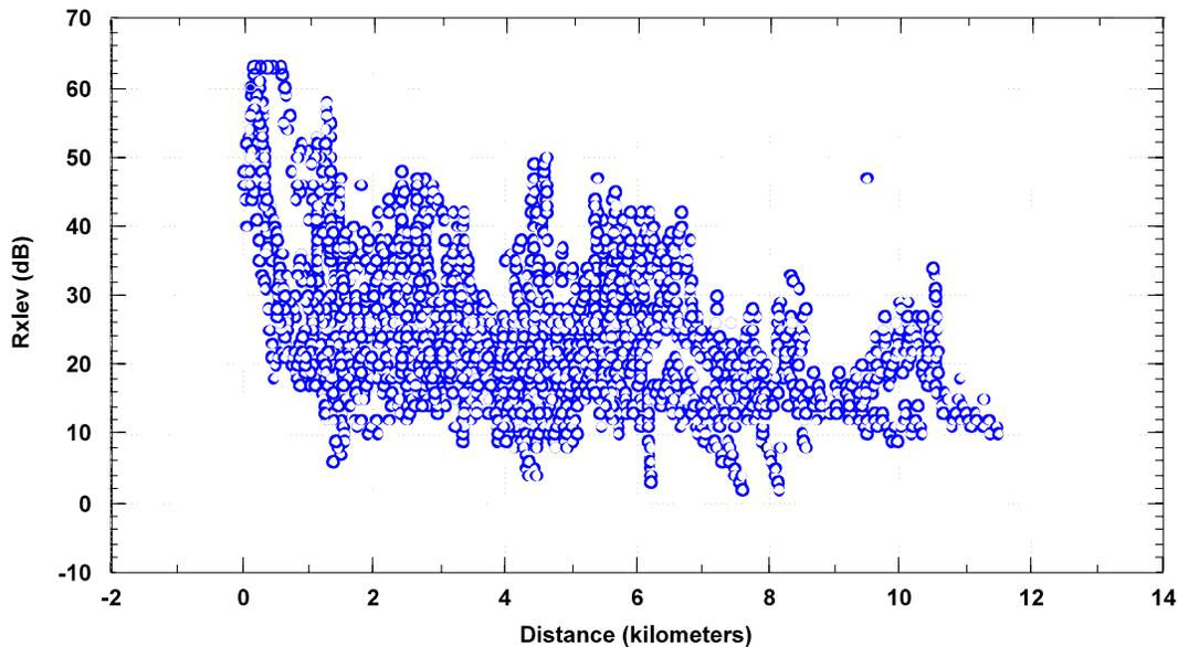
Figure 3.2. Downlink Rxlev vs. distance (TAG 5, TMCO cell).
