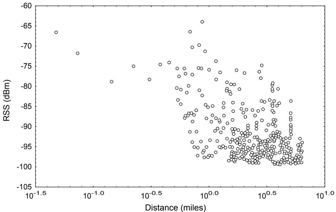
Figure 8.3. Downlink received signal strength (RSS) vs. distance (TAG 1, TMCO cell).
