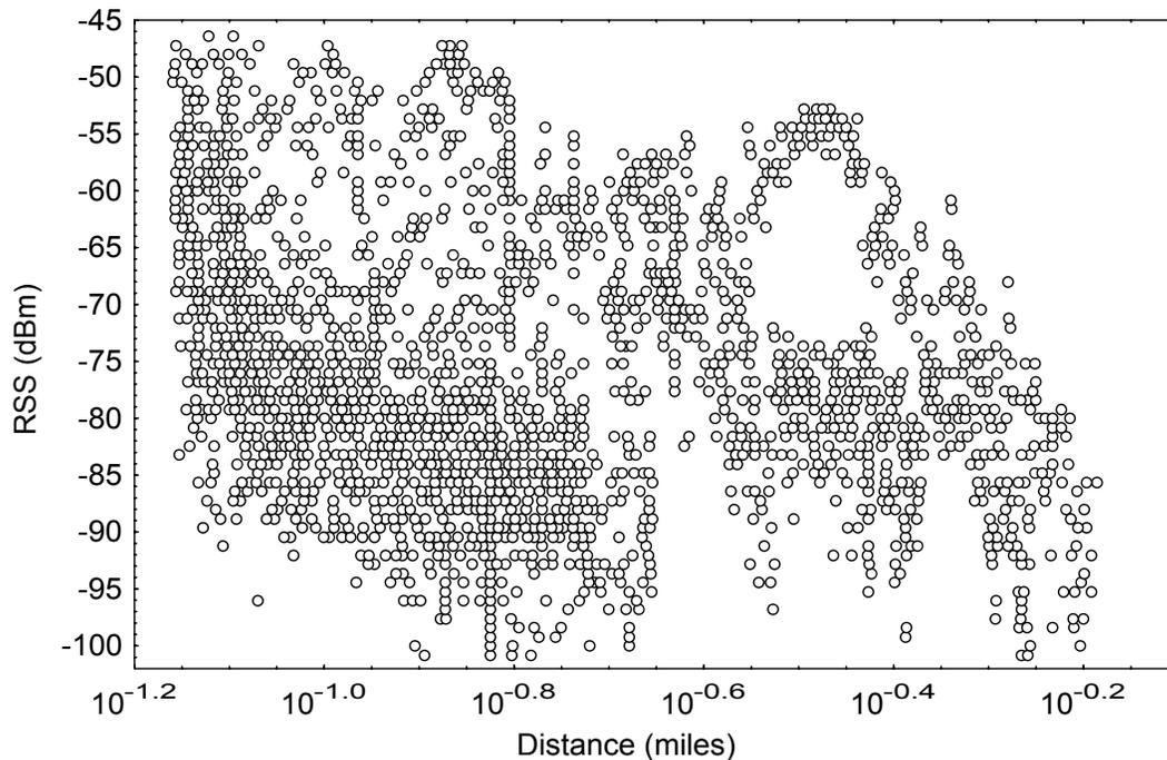
Figure 7.2. Downlink received signal strength (RSS) vs. distance (TAG 3, microcell site 1).
